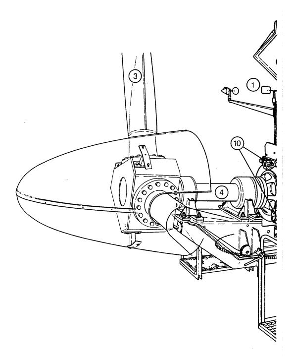
A disc brake is located directly on the main shaft to stop the rotor when necessary and to lock the rotor when wind speeds reach a certain level. Positioned to ensure that the braking load effect is not transferred to the gear box, the disc brake is equipped with
