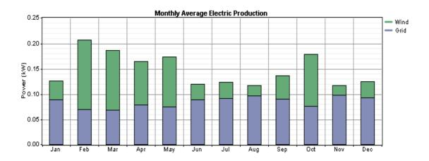
The following graph represents the distribution of the demand and the wind turbine power supply for a year. The graph represents the rural environment. In blue color is the demand while in green the wind turbine electrical production.
