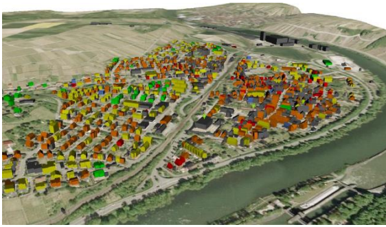
Figure 2: Example of heating demand per building in the SUNSHINE project (Bloem et al. 2015)
