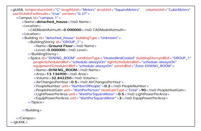
Figure 2: Excerpt of the final gbXML file for one of the 72 base case buildings, in this case the detached house with an orientation (CADModelAzimuth) of  $0^{\circ}$ .
