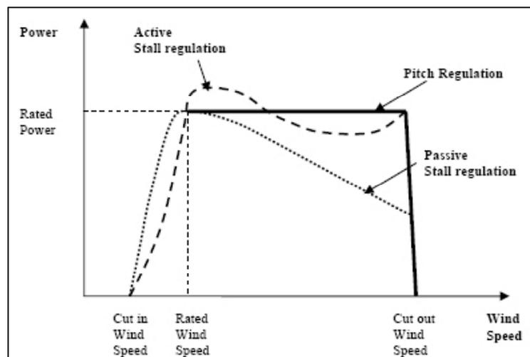
*Figure 4 Passive and active stall regulation and pitch power control (M.Ragheb, 2009)*
