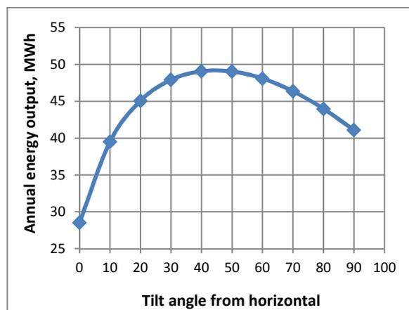
Figure 17 Annual energy output at different tilt angles
