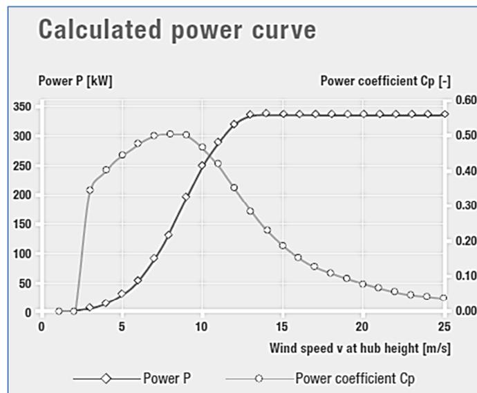
Figure 44 Enercon E-33/330kW wind turbine technical specification (Enercon, 2010)
