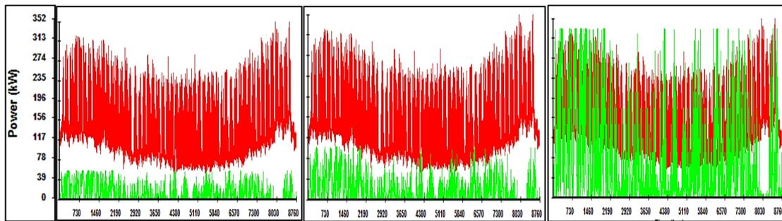
Figure 25 Energy supply (green) / demand (red) annual profile of 50kW(left), 100kW (middle), 330kW (right) wind turbines
