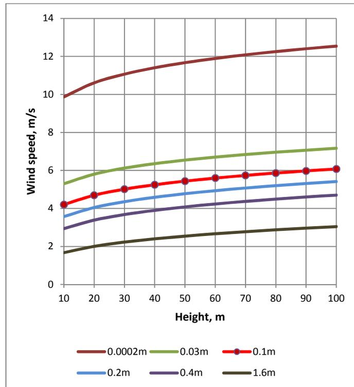
Figure 9 An example of logarithmic profile of wind speed with height for different roughness lengths
