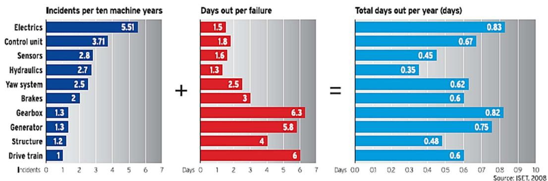
Figure 29 Failure rates and outage times of wind turbine components (ISET 2008 cited in (Milborrow, 2010))
