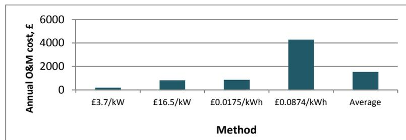
Figure 35 Annual O&M costs for PV panels using different estimating methods.
