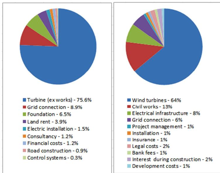
Figure 30 Cost structure of a wind turbine installation
