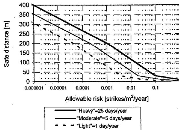
*Figure 38 Safety distance for the chosen level of risk of ice strikes for 3-blades turbine with a 50m of diameter (Colin Morgan E. B.)*
