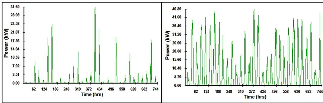
Figure 21 Difference in power output from 50kW PV, January (Left) and July (right).
