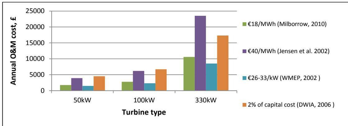
Figure 34 Annual O&M costs for wind turbines using different estimating methods.
