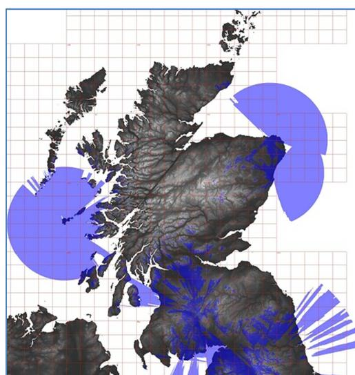
*Figure 14 Introductory map of radar restricted zones (blue areas) for wind turbines with up to 60m height (NATS)*
