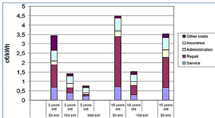
Figure 32 O&M Costs for selected types and ages of turbines (Jensen et al. (2002) cited in (Operation and Maintenance Costs of Wind Generated Power))
