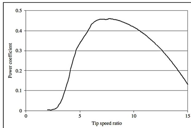
Figure 3 Illustration of power coefficient/tip-speed ratio curve,  $C_p/\lambda$  (Olimpo Anaya-Lara, 2009, p. 5)
