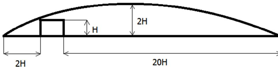
*Figure 12 Turbulence zone behind obstacles with height  $H$  (Harry L. Wegley)*
