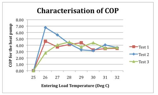
Figure 19: The Coefficient of performance of the test rig for experiment 1.
