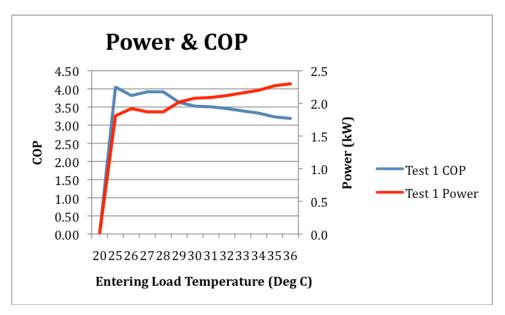
Figure 21: Power consumption and COP for experiment 2.
