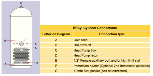
Figure 11: Newark Copper 300 Litre Heat Pump cylinders.
