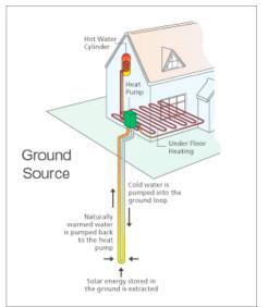
Figure 6: GSHP with ground loop water to water (HPA n.d.).
