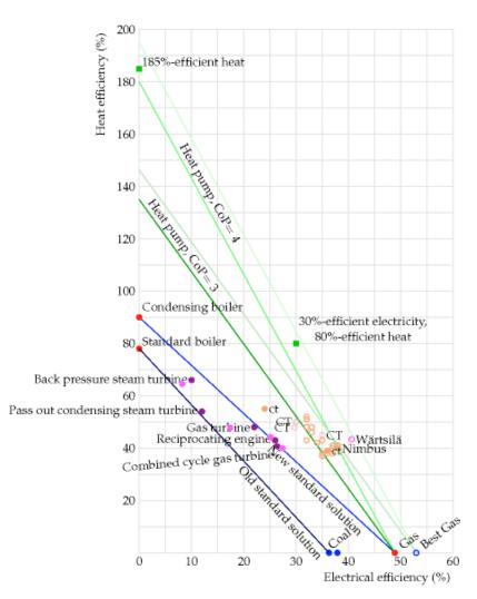
Figure 7: The Effectiveness of a heat pump compared to other technologies (MacKay 2009)
