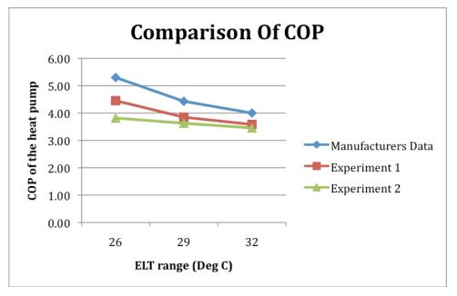
Figure 22: Comparison between experiments and manufacturers data for 0.25 l/s.
