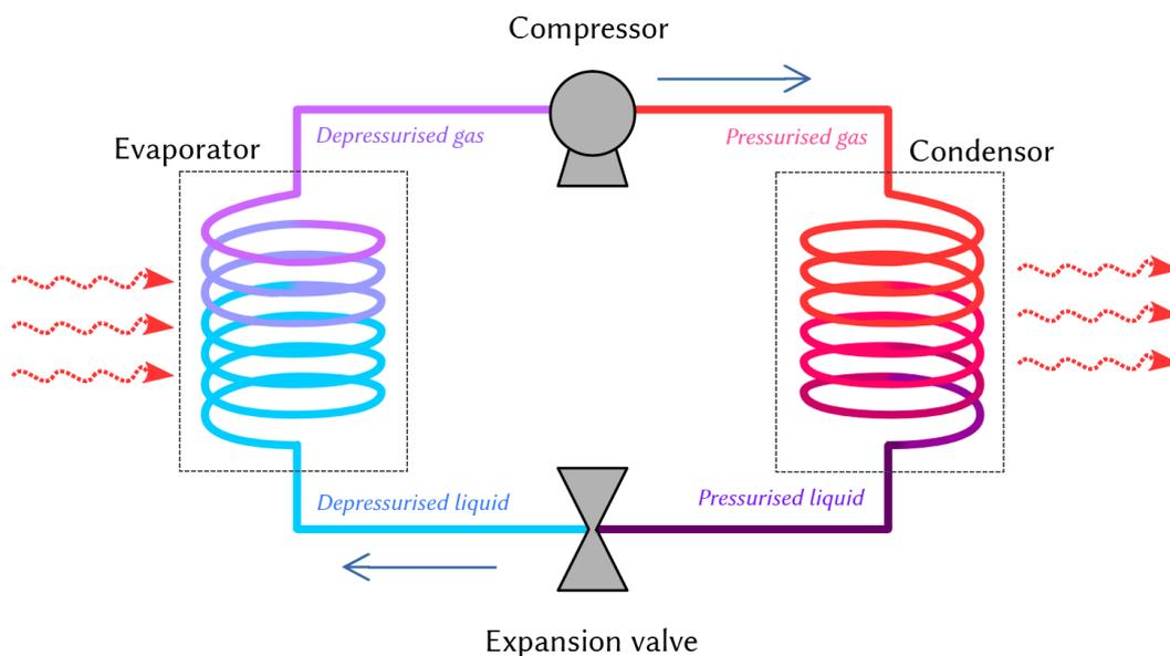
Figure 9: Conceptual diagram of a heat pump
