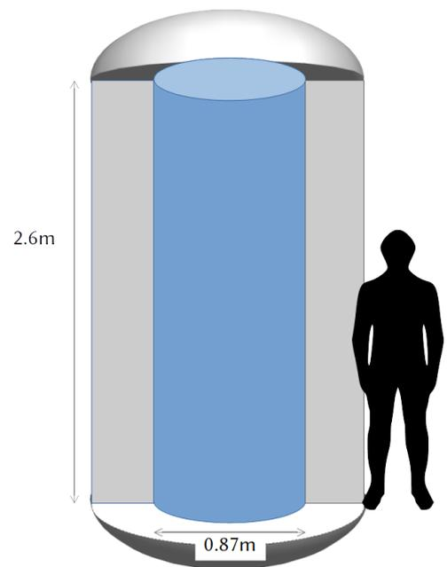
Figure 15: Dimensions of the modelled tank
