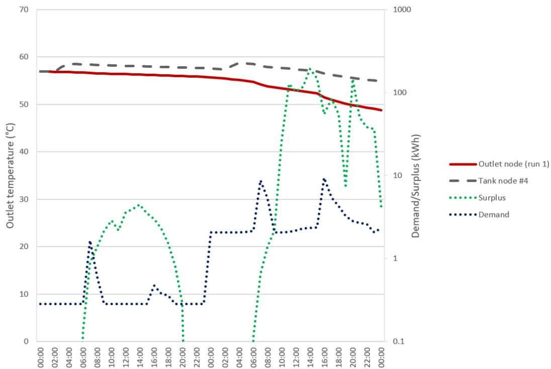
Figure 31: Simulation output for May 1st-2nd 2019. In this case no heating was needed as the system was able to ‘coast’ to the prediction horizon from a near-full tank.
