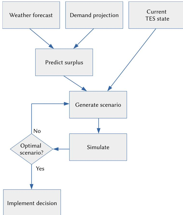
Figure 20: Process flow for MPC controller
