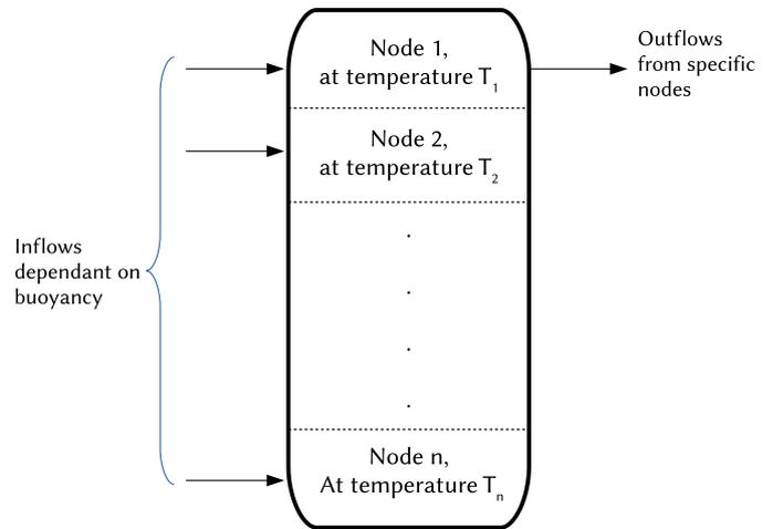
Figure 7: One dimensional multi-node model for TES
