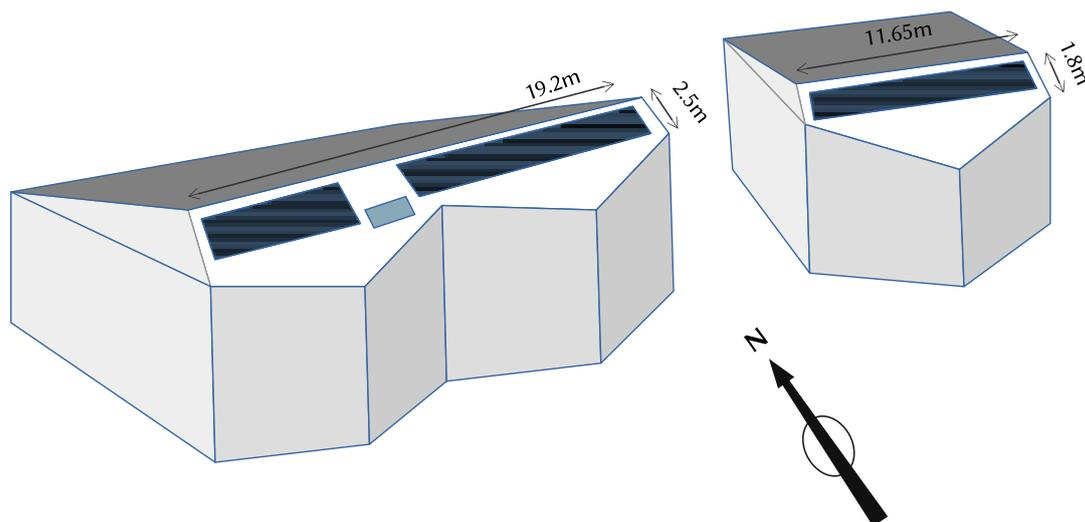
Figure 18: Plausible sizes of solar arrays on study buildings
