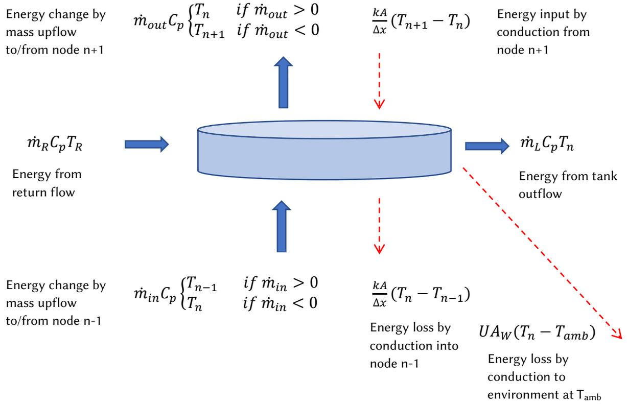
Figure 8: Energy balance on an arbitrary tank node  $n$ .  $m_{out} = 0$  at top node,  $m_{in} = 0$  at bottom node,  $m_R$  and  $m_L$  are only nonzero for nodes with external connections.
