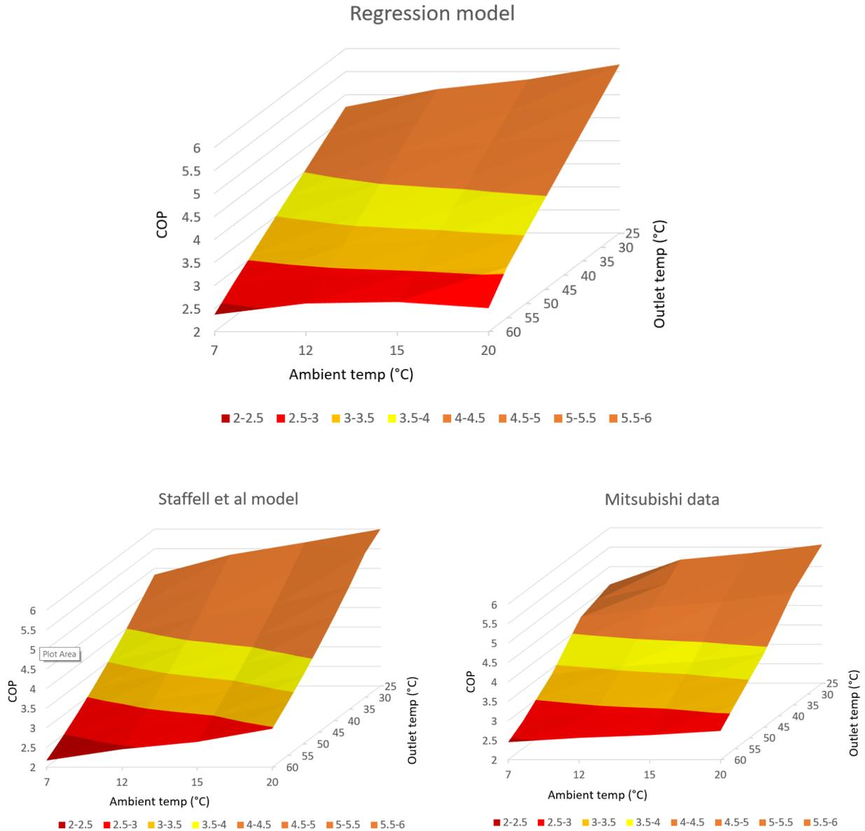
Figure 16: 2-dimensional characteristics of the ASHP, obtained by regression (top), compared to a standardised model after Staffell et al (2012) (lower left) and from raw manufacturer data (lower right)
