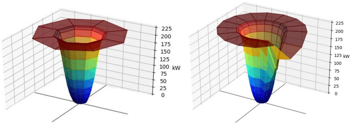
Figure 33: Wind farm "power cones"— left: the theoretical, rotationally symmetric cone; right: a hypothetical power cone showing an obstacle reducing power output from southeasterly wind.
