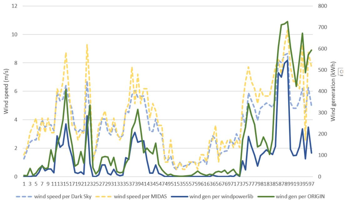
Figure 25: Wind speed from MIDAS and Dark Sky, and generation data from windpowerlib and ORIGIN compared
