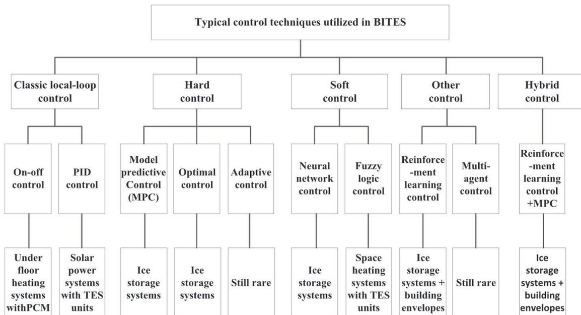
Figure 10: Control techniques used in Buildings Integrated with Thermal Storage (BITES) with some typical applications. From Yu et al (2015) after Afram and Janabi-Sharifi (2014)
