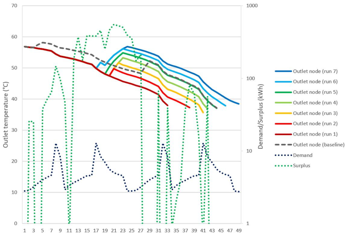
Figure 30: Scheduling simulation output for February 1st-2nd 2019. 7 runs were performed to find a successful scenario with 6 hours of heating.
