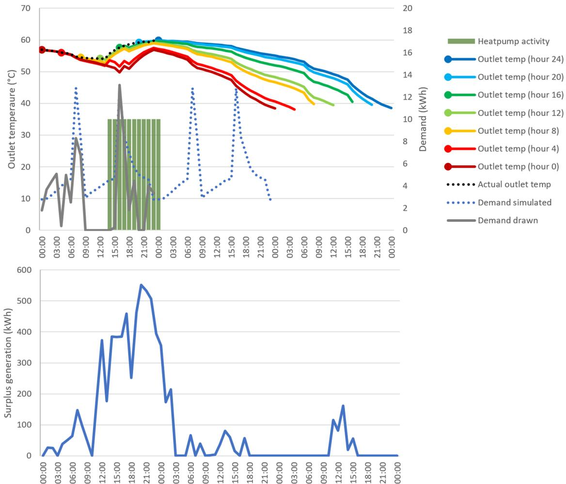
Figure 32: Output from a simulated 24-hour run of the scheduler
