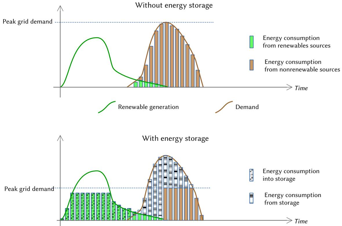
Figure 2: The intelligent use of storage to reduce grid demand and increase consumption of intermittent renewable sources.
