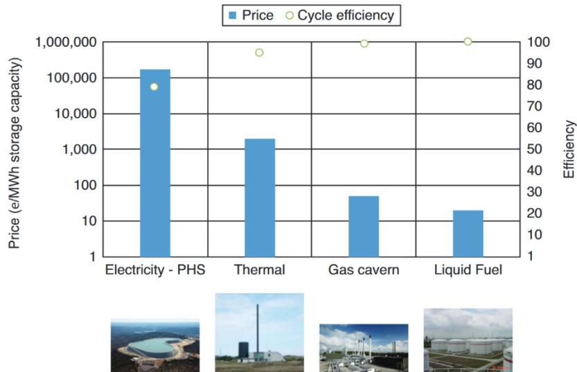
Figure 1: Investment cost and cycle efficiency comparison of electricity storage (as pumped hydropower), thermal energy storage, gas cavern storage and liquid fuel. From Lund et al (2016)
