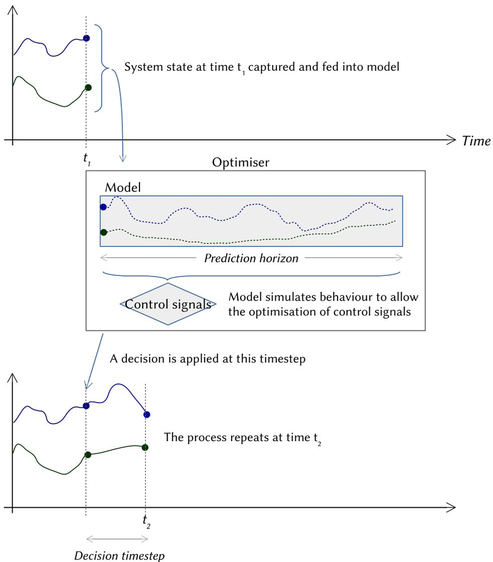
Figure 11: Conceptual outline of an MPC process
