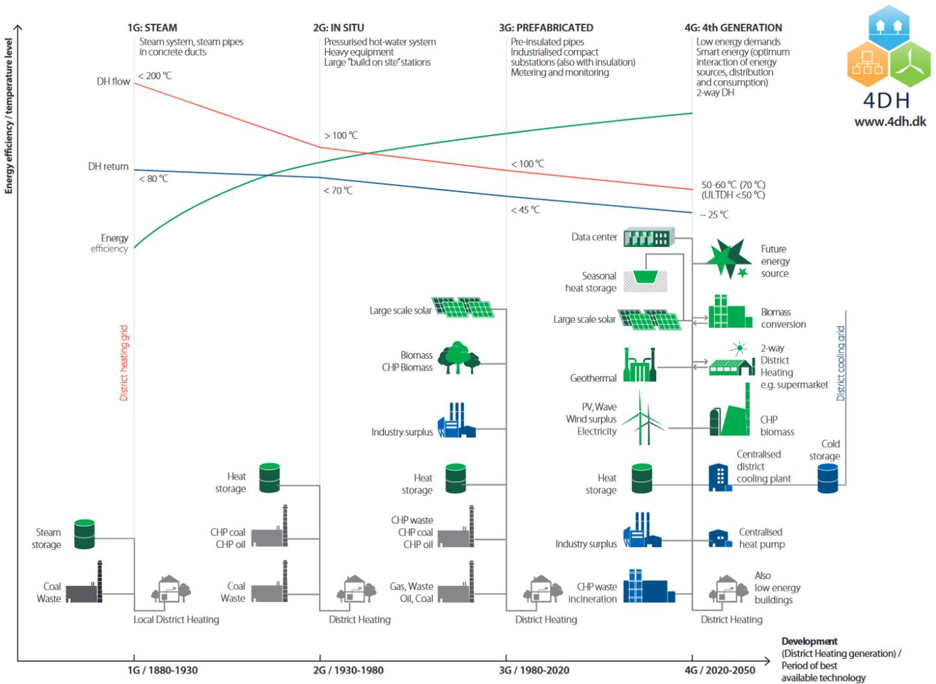
Figure 6: "Progression of District Heating – 1st to 4th generation," Thorsen et al (2018)
