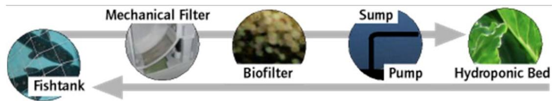
Figure 25: Basic aquaponic system layout (Goddek et al., 2015)
