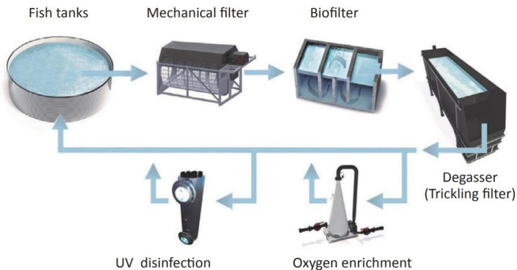
Figure 46: RAS recirculation key components (FAO, 2015)
