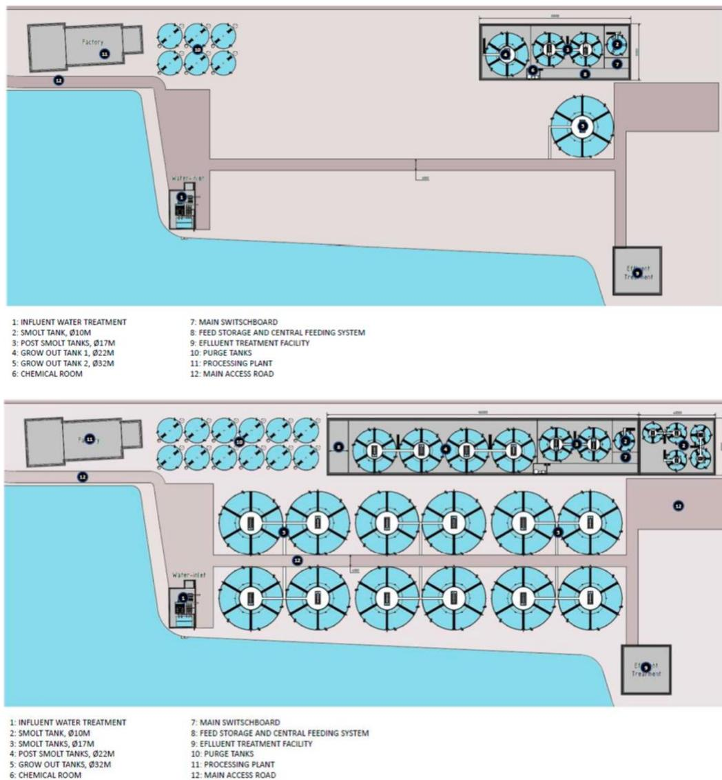
Figure 49: Example of modular design for a recirculating aquaculture system plant (Niri.com, 2018)
