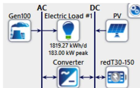
**Figure 42: PV-Diesel Generator System with Vanadium Flow Battery**
