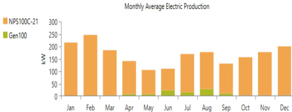
**Figure 45: Monthly Average Electric Production of Wind-Diesel (vanadium flow) System**
