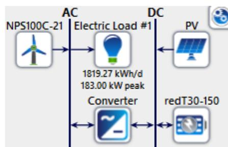
**Figure 48: Wind-PV with Vanadium Flow battery System**
