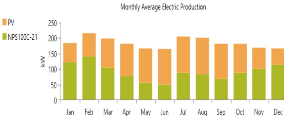
**Figure 49: Monthly Average Electric Production of Wind-PV (vanadium flow) System**
