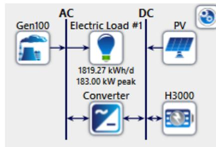
**Figure 26: PV-Diesel Generator with lead acid battery**
