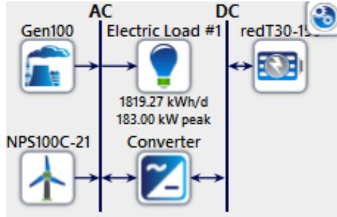
**Figure 44: Wind-Diesel Generator with vanadium flow battery System**
