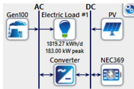
**Figure 34: PV-Diesel Generator with lithium-ion battery**
