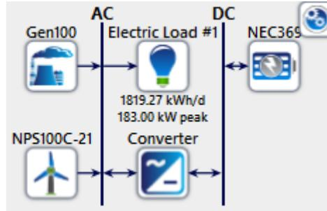
**Figure 36: Wind-Diesel Generator with lithium-ion battery**
