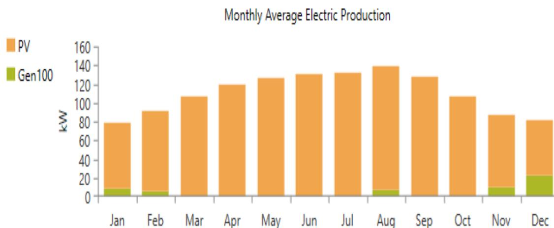
**Figure 27: Monthly average electricity production from PV-Diesel system (lead acid)**
