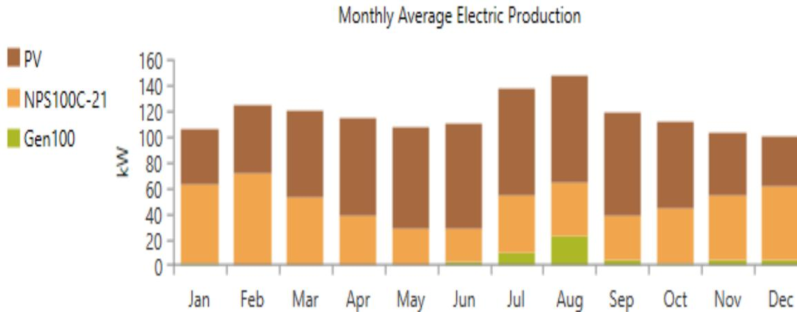
**Figure 47: Monthly Average electric Production from Wind-PV-Diesel (vanadium flow) System**
