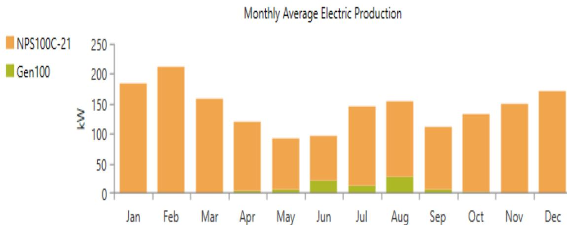
**Figure 29: Monthly Average Energy Production of Wind-Diesel Generator (lead acid) System**
