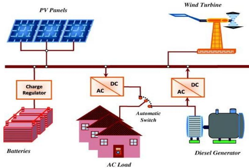
**Figure 8: Wind-PV-Diesel system with storage (Abdelhamid Kaabeche, 2014)**
