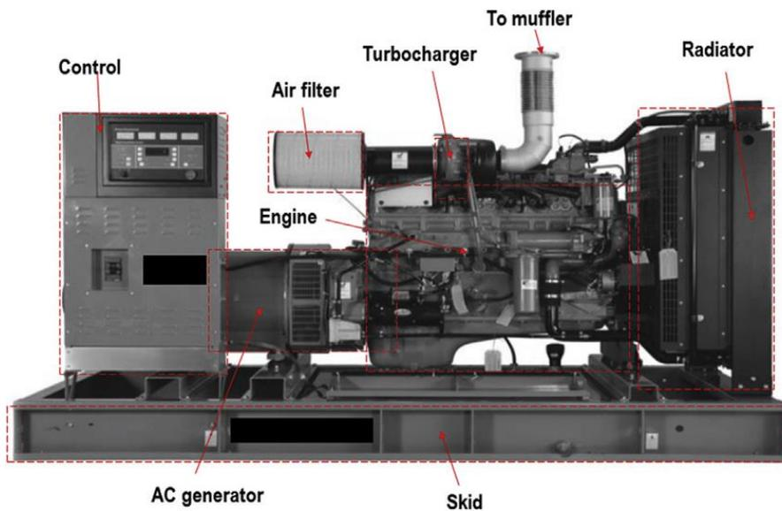
**Figure 7: A typical diesel engine and its main components (Kelly Benton, 2017)**
