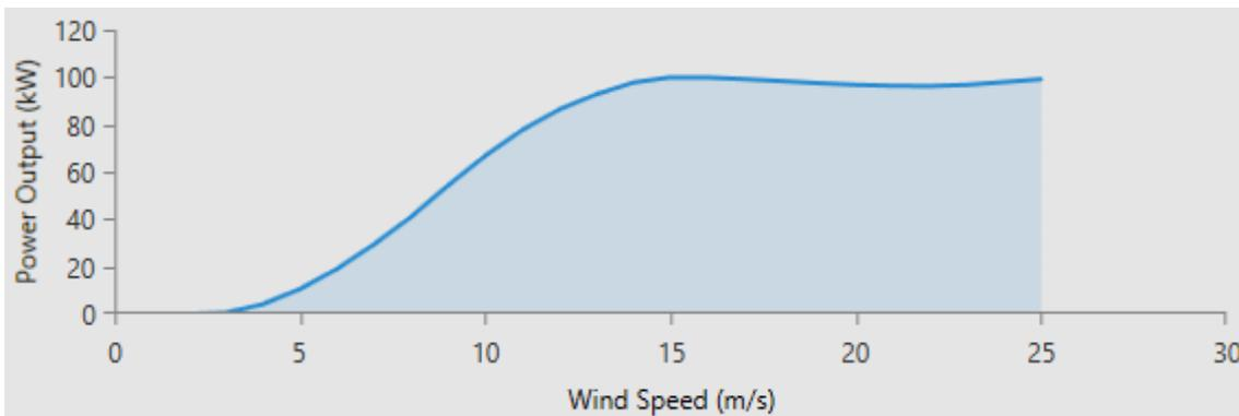
**Figure 23: Wind Turbine Power Curve**
