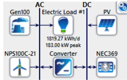
**Figure 38: Wind-PV-Diesel Generator (lithium-ion) System**
