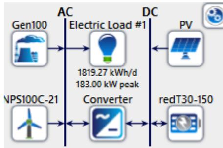
**Figure 46: Wind-PV-Diesel Generator with vanadium flow battery System**
