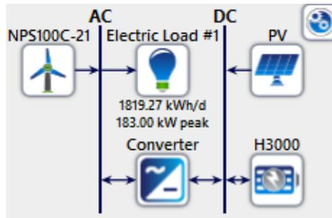
**Figure 32: Wind-PV System with lead acid battery**
