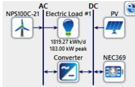
**Figure 40: Wind-PV (lithium-ion) System**
