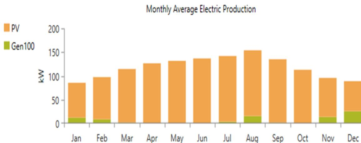
**Figure 43: Monthly Average Electric Production from PVs-Diesel (vanadium-flow) System**
