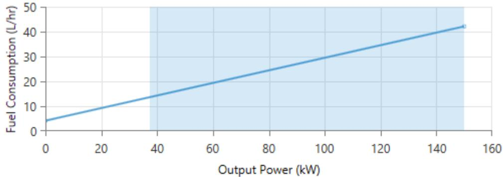
**Figure 24: Fuel curve of the diesel generator**
