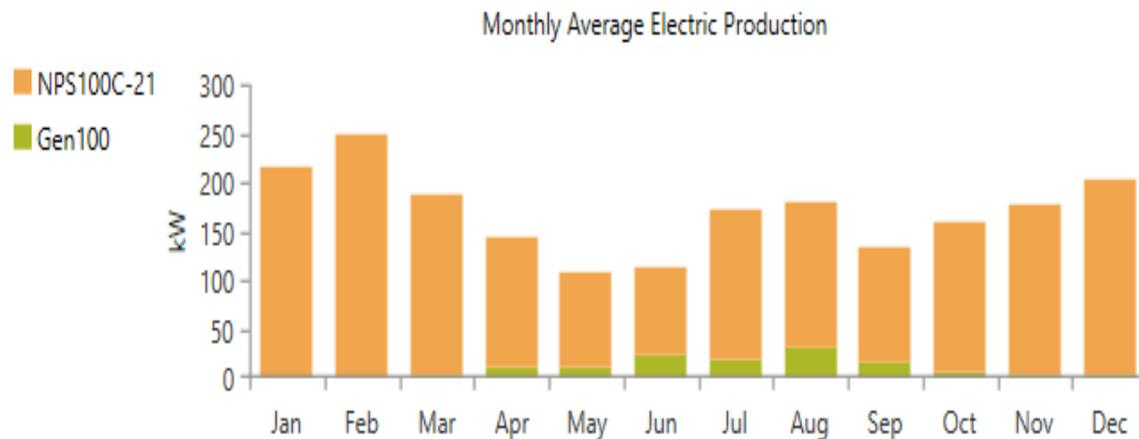
**Figure 37: Monthly Average Electric Production of Wind-Diesel (lithium-ion) System**
