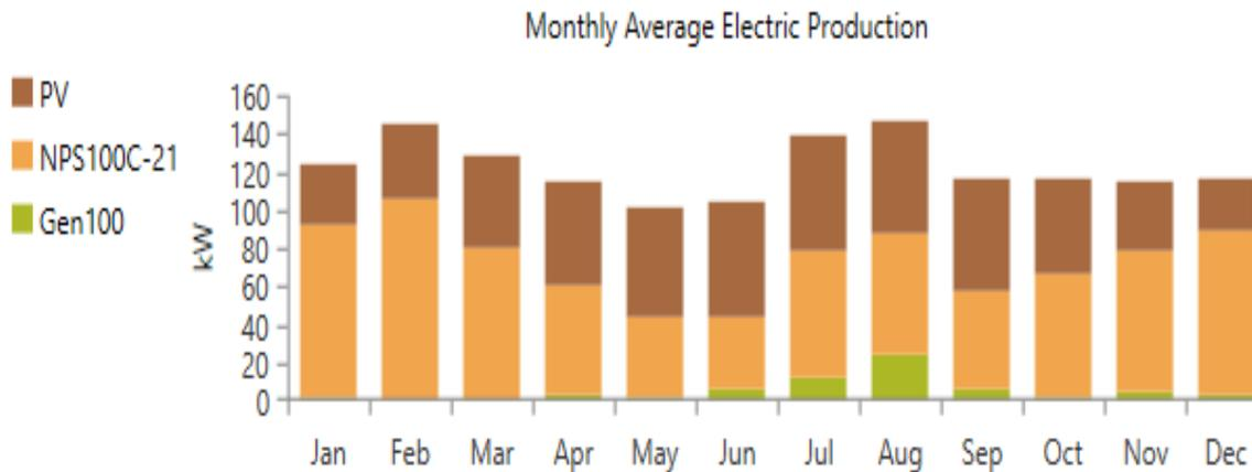
**Figure 39: Monthly Average Electric Production from Wind-PV-Diesel (lithium-ion) System**
