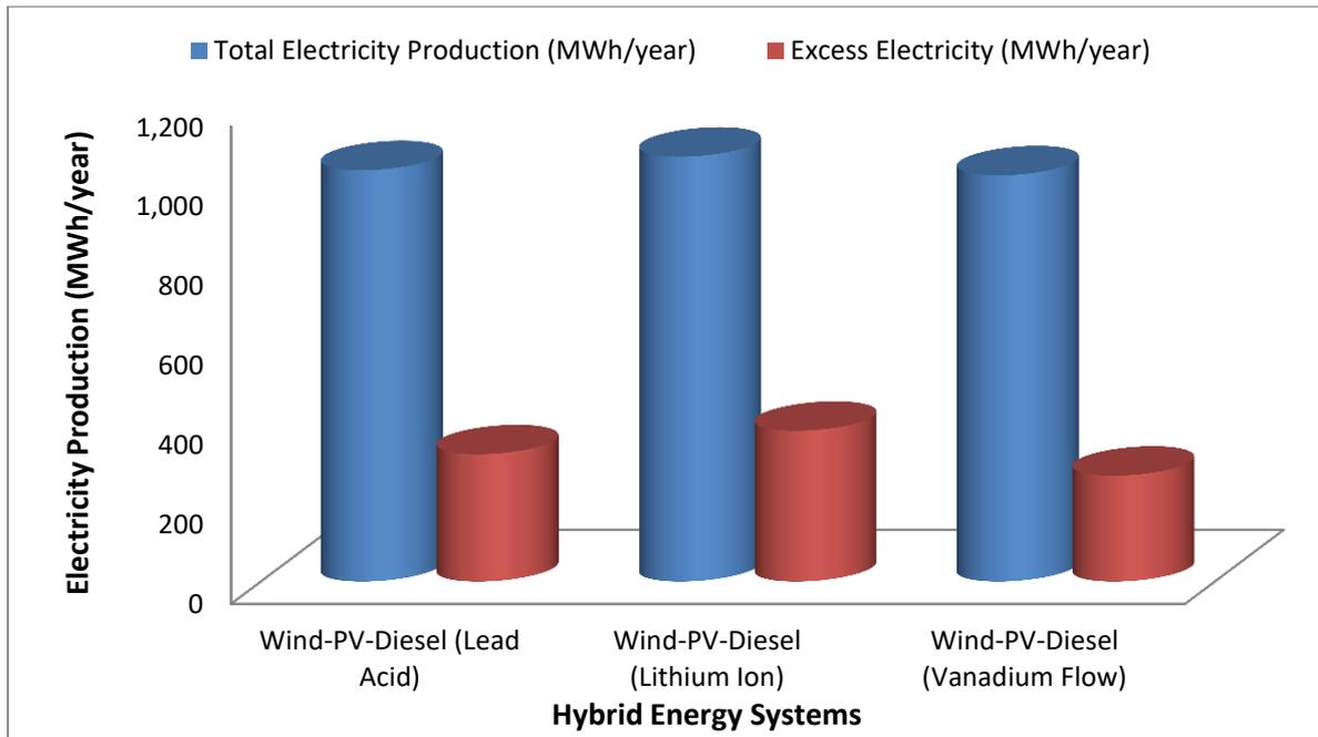
**Figure 53: Electricity Production and Excess Electricity for the Optimized Energy Scenarios**
