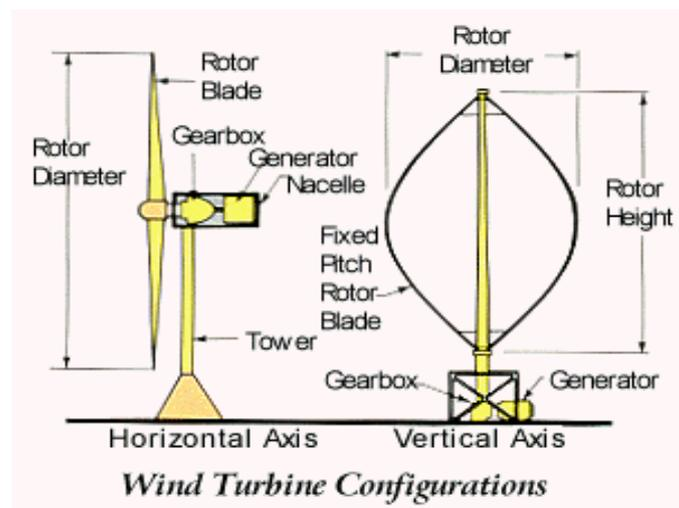
**Figure 12: Horizontal axis and vertical-axis wind turbine (Renewable Energy Sources , 2009)**
