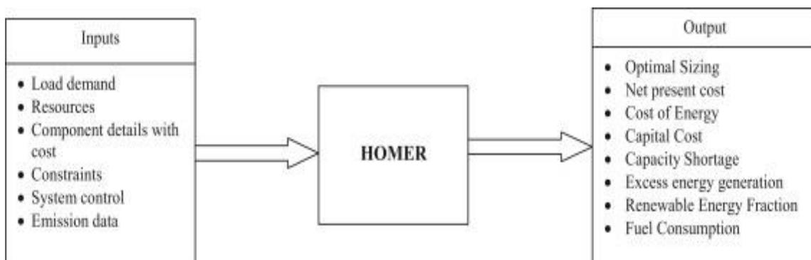
**Figure 17: Representation of inputs and outputs of HOMER (Sunanda Sinha, 2014)**
