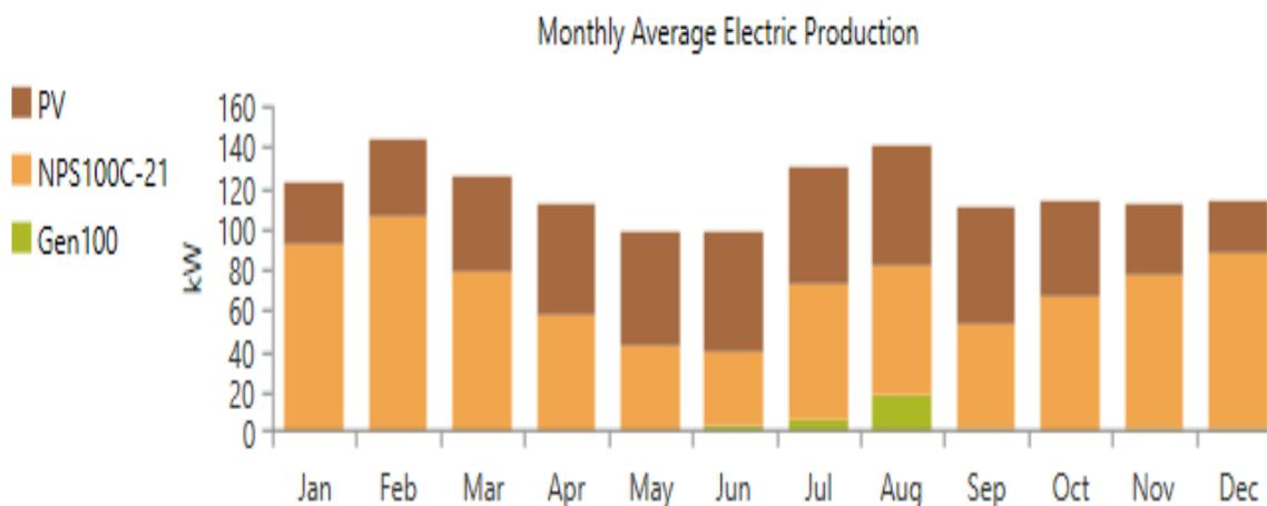
**Figure 31: Monthly Average Electric Production from Wind-PV-Diesel (lead acid) System**
