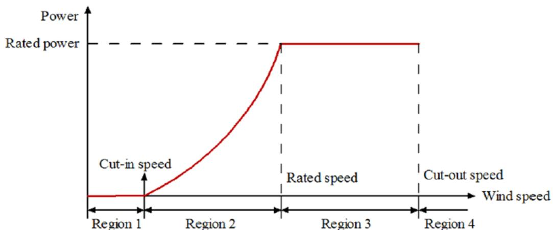
**Figure 13: Typical power curve of a wind turbine (Rahul Dutta, 2014)**
