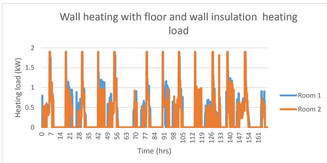
Figure 74: Heating load for wall heating with better control and floor and wall insulation
