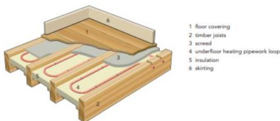
Figure 17: Timber floor UFH design with lightweight screed
