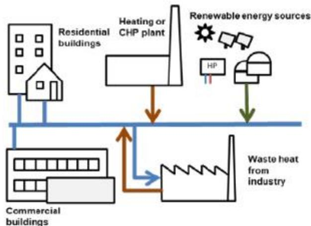
Figure 10: Schematic DH network with multiple supply options
