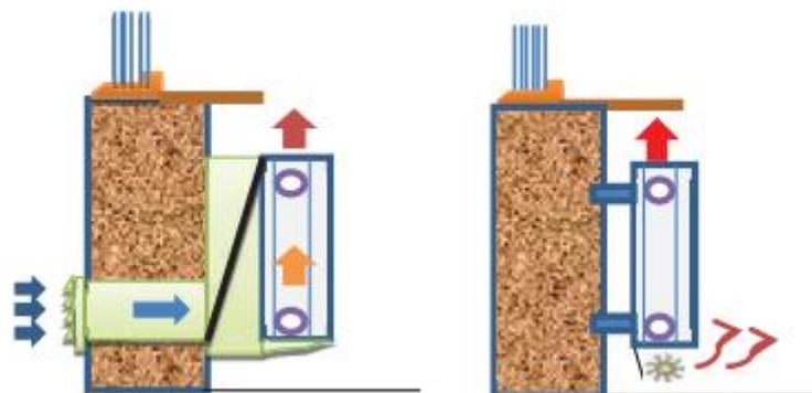
Figure 22: Ventilation radiator (left) and add on fan radiator (right)
