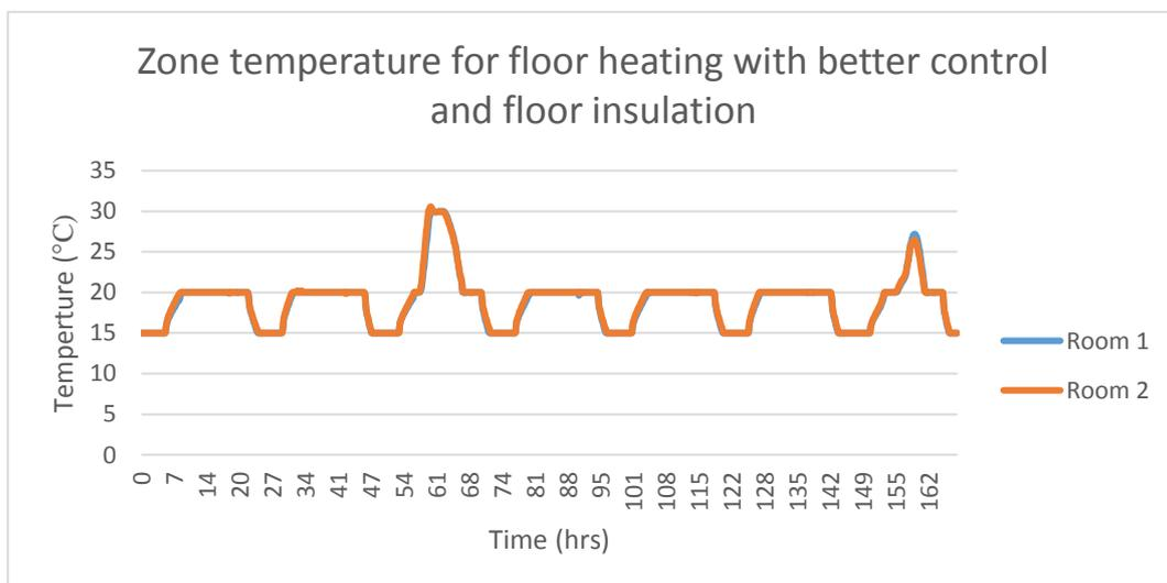
*Figure 35: Floor heating with better control and floor insulation zone temperature*
