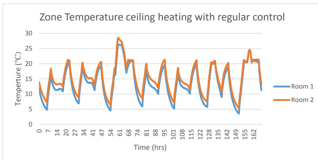
Figure 39: Ceiling heating with regular control zone temperature
