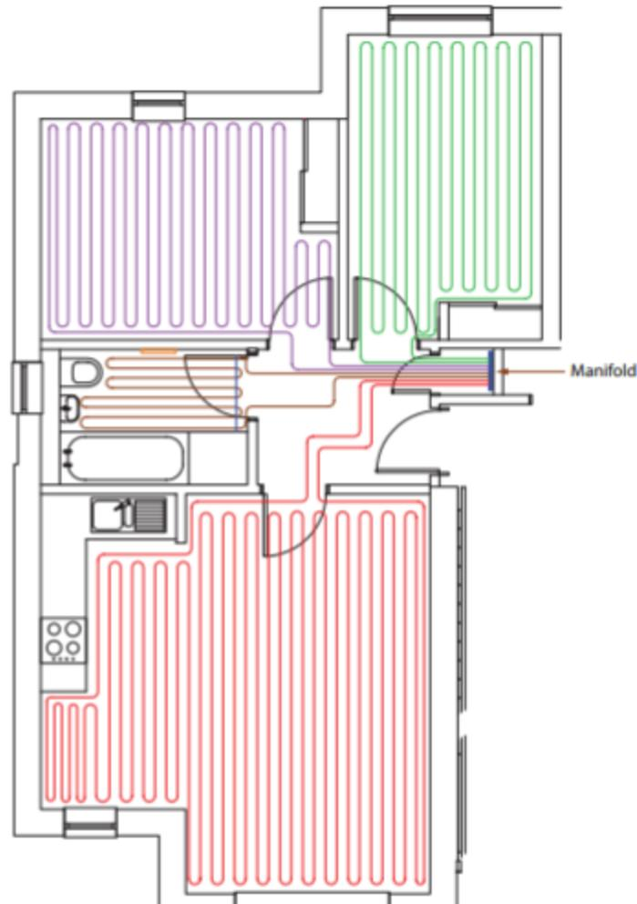
*Figure 56: Typical UFH piping system layout for an apartment (Bleicher & Vatal, 2016)*
