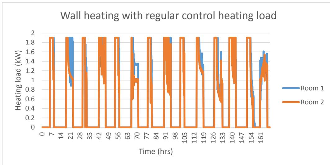
Figure 73: Heating load for wall heating with regular control
