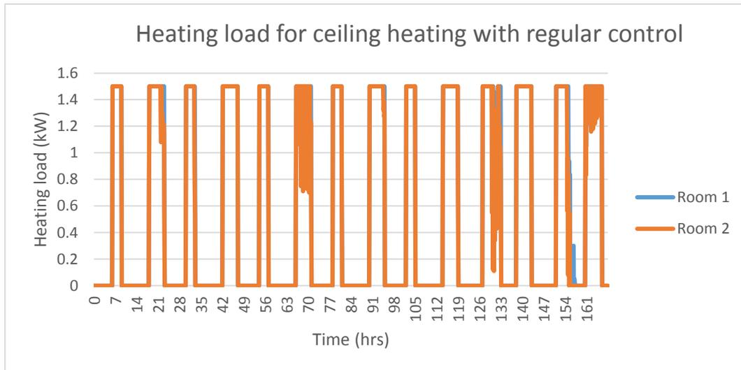
Figure 41: Ceiling heating with regular control heating load
