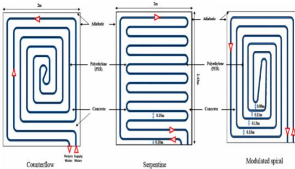
Figure 59: Three possible pipe configurations for UFH (Oubenmoh et al., 2018)
