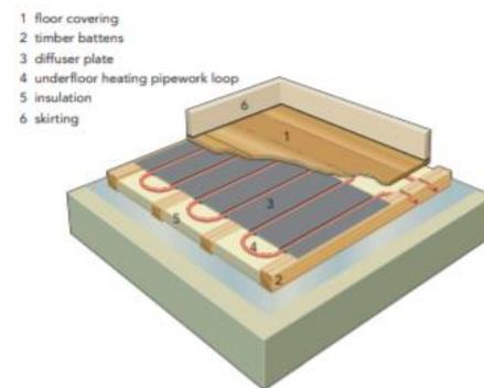
Figure 14: Timber floor UFH design with diffuser plate
