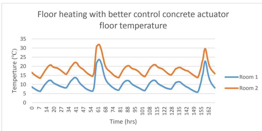
Figure 64: Floor temperature for floor heating with better control and concrete actuator
