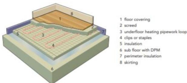
Figure 15: Concrete floor UFH design
