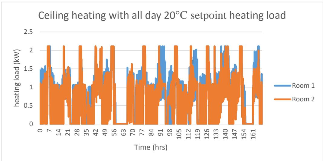
Figure 72: Heating load for ceiling heating with better control 20°C set point
