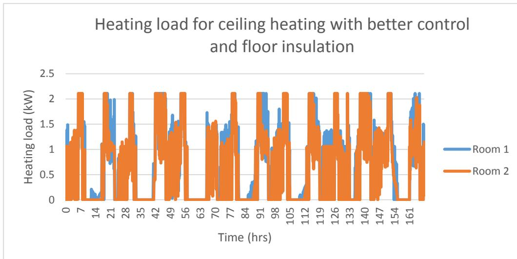
Figure 44: Ceiling heating with better control and floor insulation heating load
