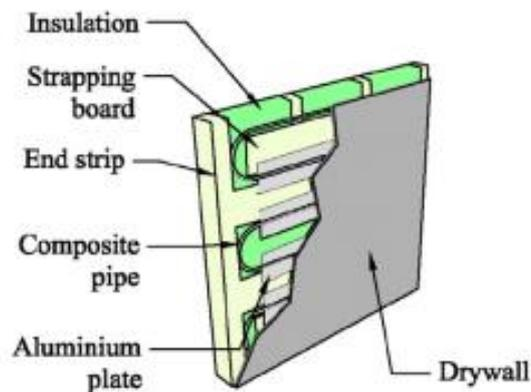
*Figure 21: Wall or ceiling heating panel*
