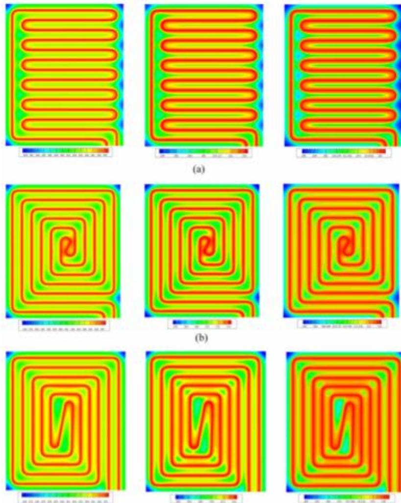
Figure 60: Floor surface temperature of three configuration from 35-50°C left to right (Oubenmoh et al., 2018)
