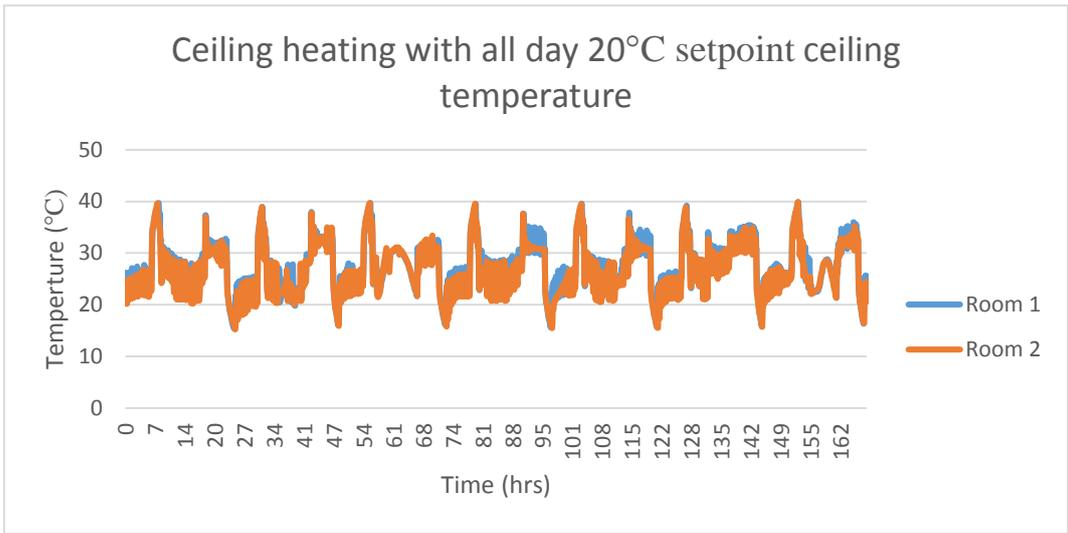
Figure 71: Ceiling temperature for ceiling heating with better control 20°C set point
