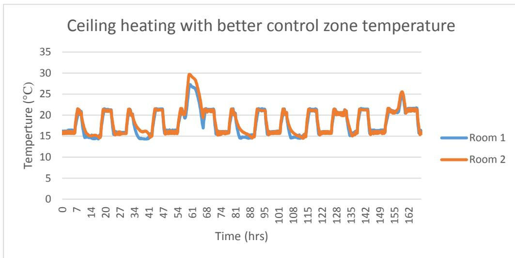
Figure 68: Zone temperature for ceiling heating with better control no floor insulation
