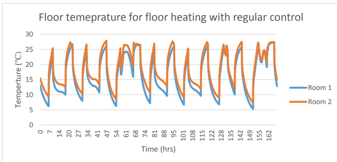
Figure 30: Floor heating with regular control zone floor temperature
