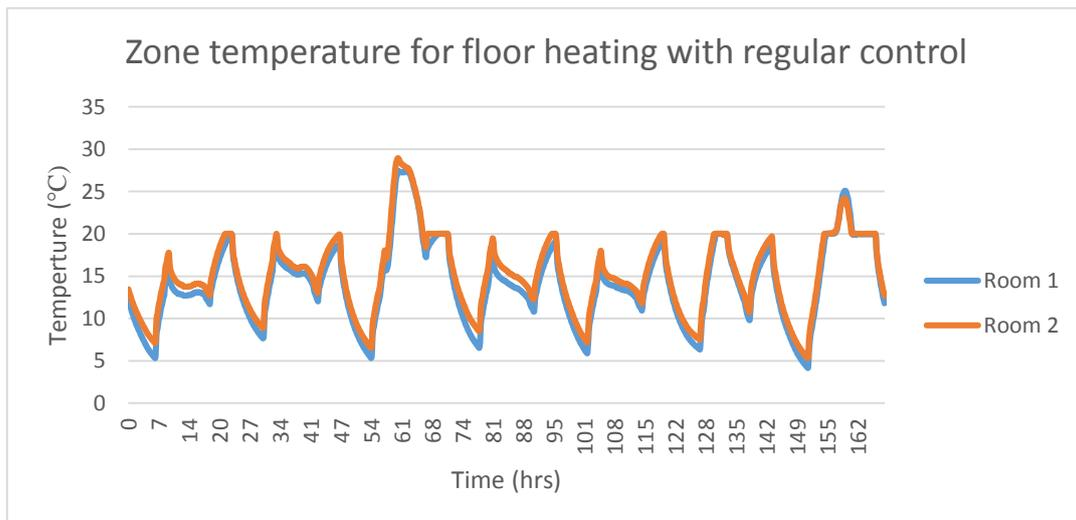
Figure 29: Floor heating with regular control zone temperature
