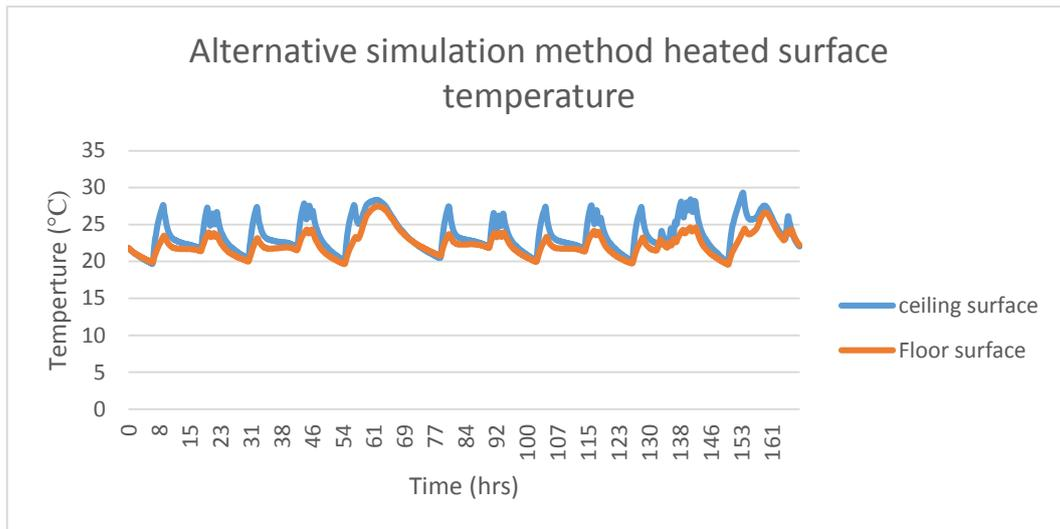
Figure 52: Surface temperature for floor and ceiling panel alternative simulation method
