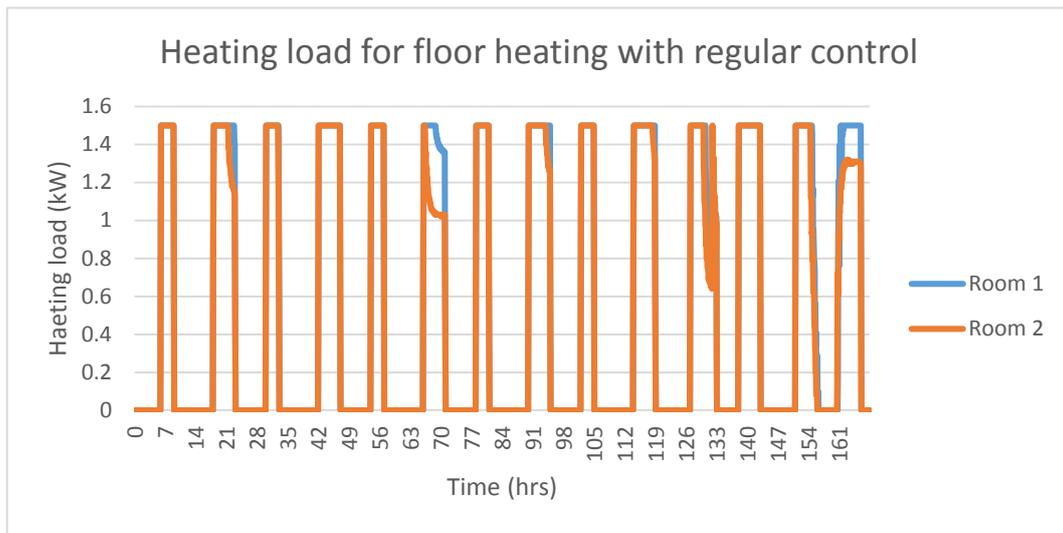
Figure 31: Floor heating with regular control heating load
