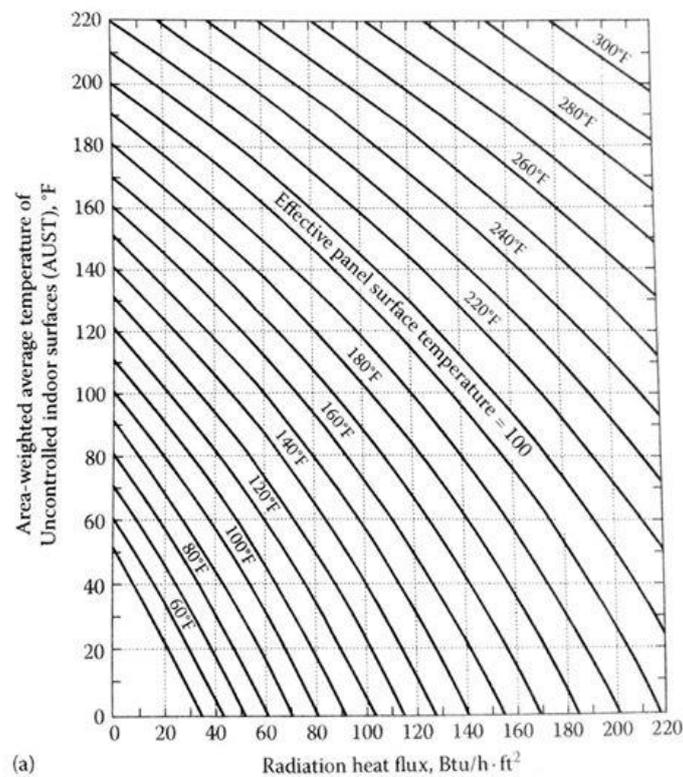
Figure 19: Radiation heat flux plots for ceiling, wall or floor heated panels
