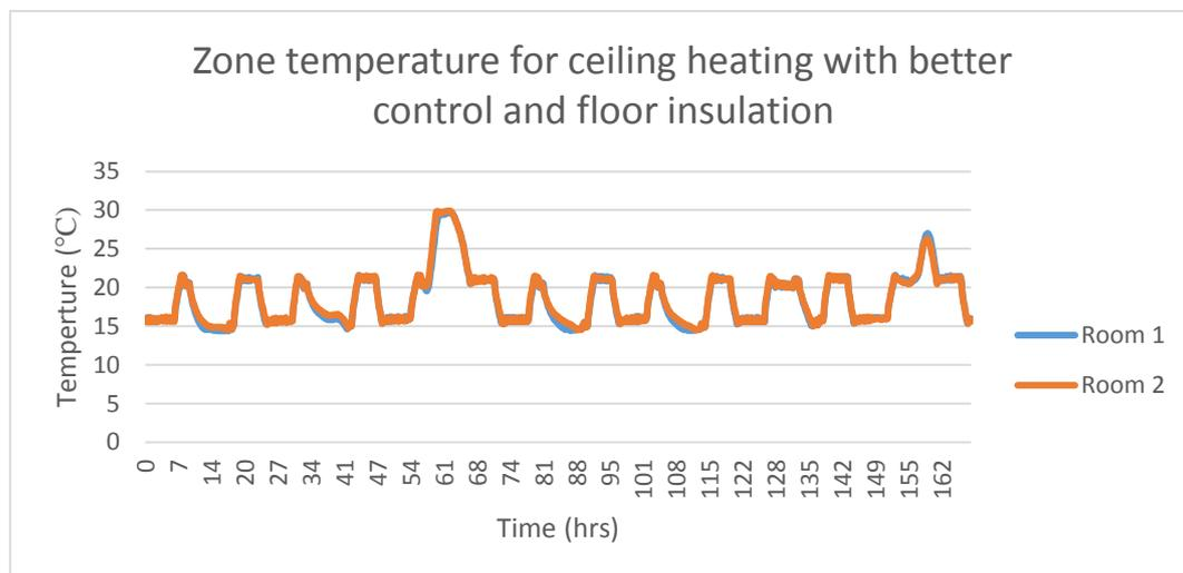
Figure 42: Ceiling heating with better control and floor insulation zone temperature
