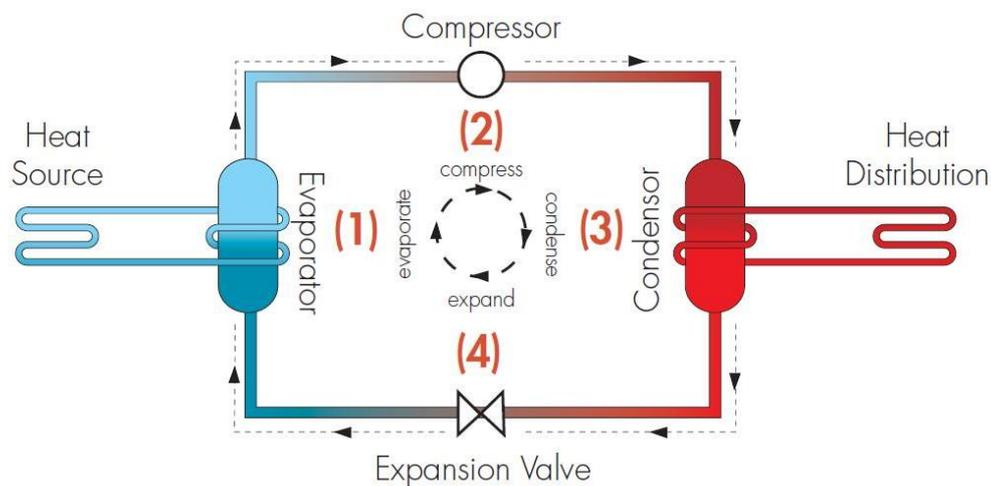
*Figure 12: Heat pump cycle*
