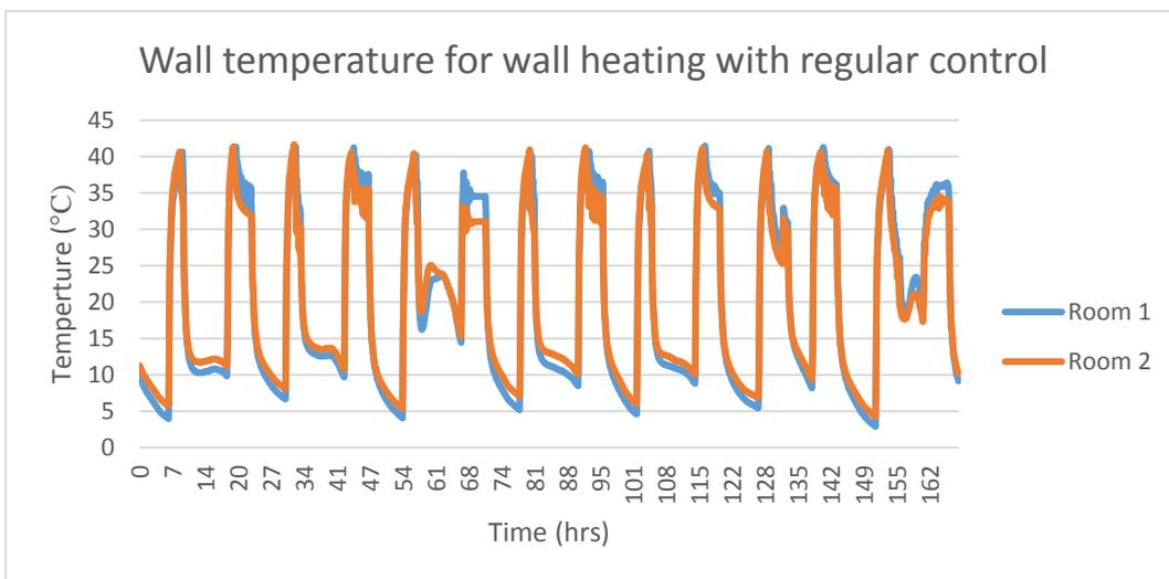
Figure 47: Wall heating with regular control wall temperature
