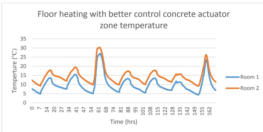
Figure 63: Zone temperature for floor heating with better control concrete actuator
