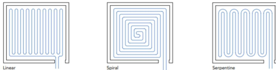
*Figure 18: Typical UFH pipework layout patterns*
