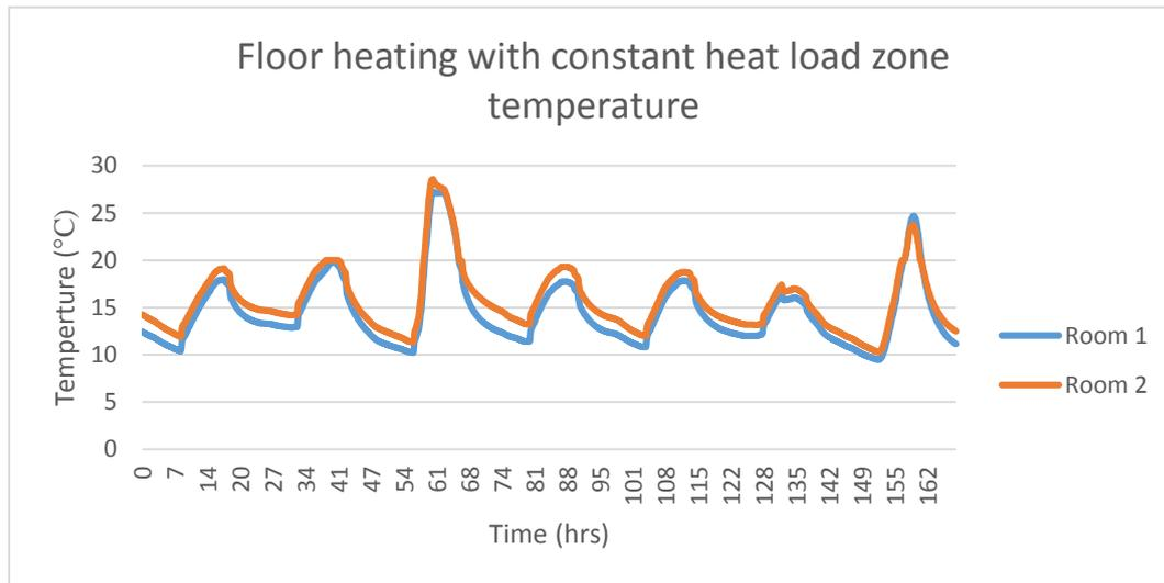
*Figure 66: Zone temperature for floor heating with constant 600W heat input*
