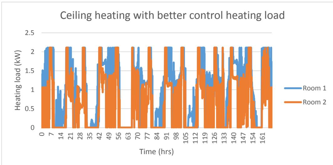
Figure 69: Heating load for ceiling heating with better control no floor insulation
