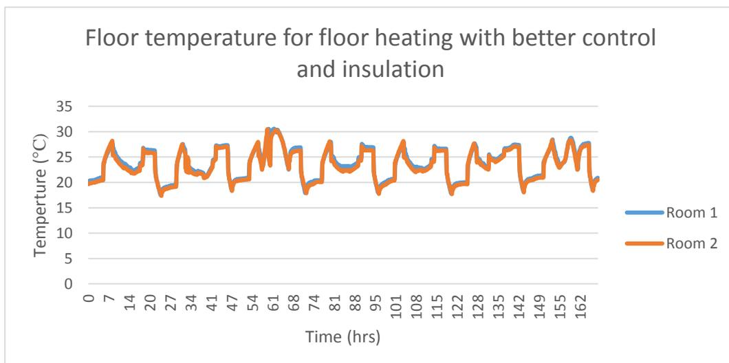
Figure 36: Floor heating with better control and insulation floor temperature
