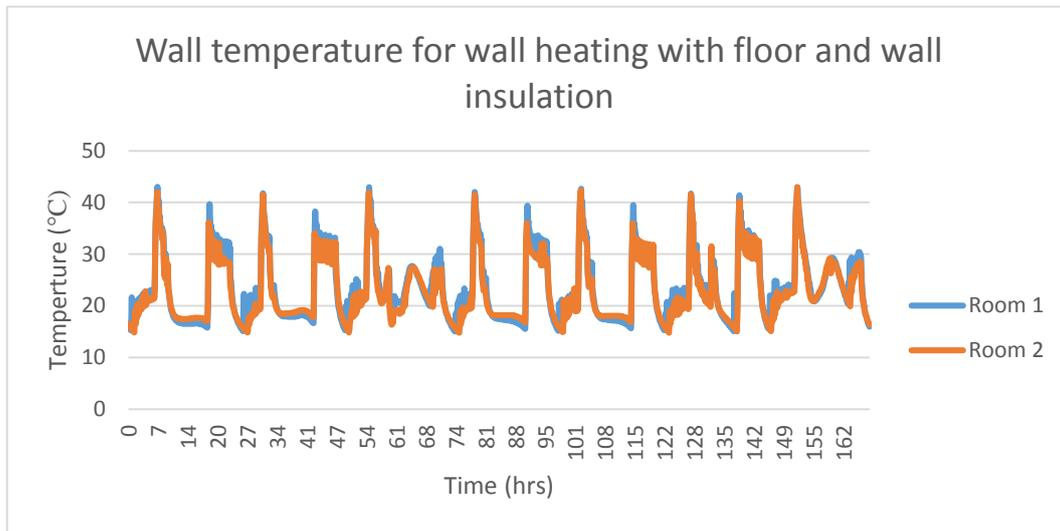
Figure 49: Wall heating with floor and wall insulation wall temperature
