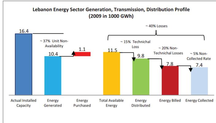
Figure 2.5: Transmission, Distribution and Losses (Fardoun, et al., 2012)
