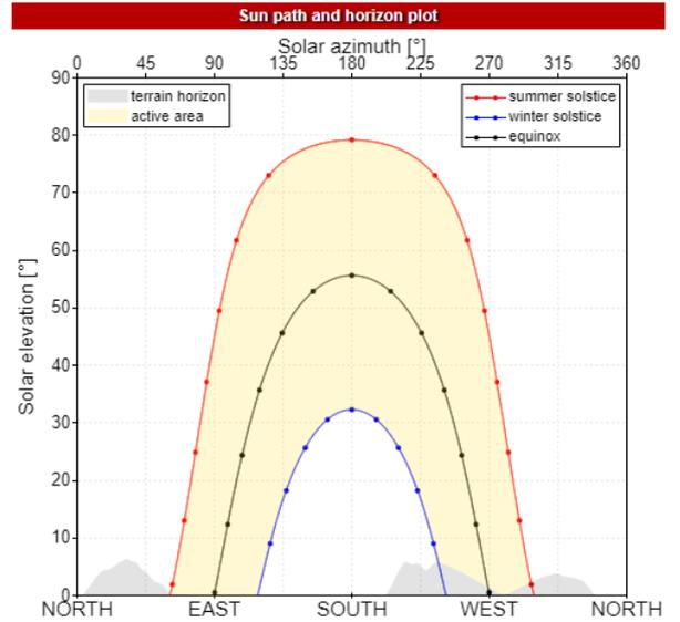
Figure 3.8: Solar Path and Horizon
