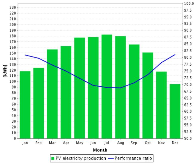
Figure 3.7: 1 kW PV Performance on 15° Plot
