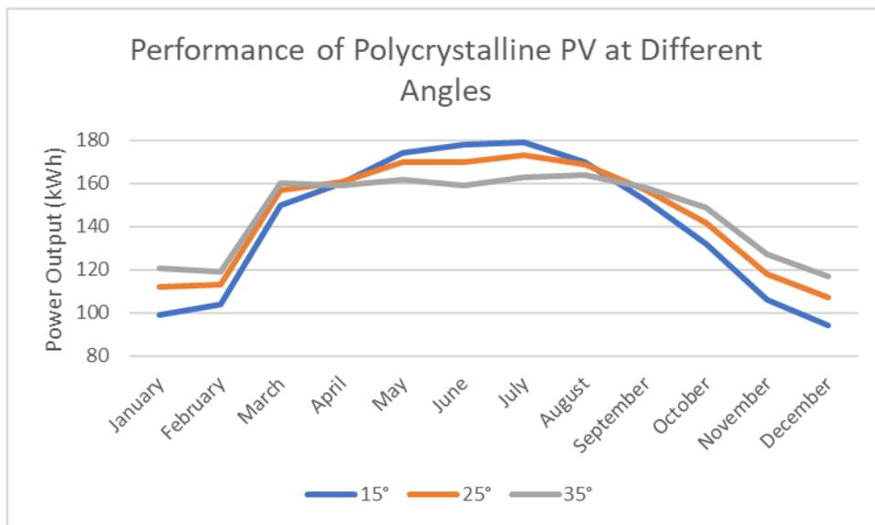
Figure 3.9: Variation of PV Power Output with Respect to change of panel's angle
