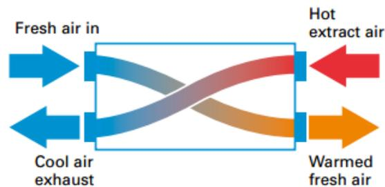
Figure 13: Schematic of a heat recovery system [60].
