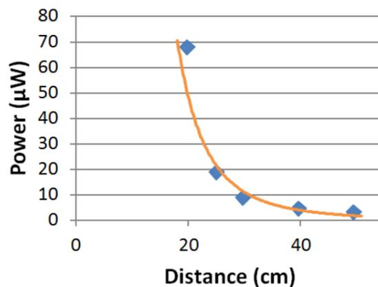
Figure 10 - Graph showing the trend in power output against the distance between the incident and rectenna (Tudose and Voinescu, 2013)
