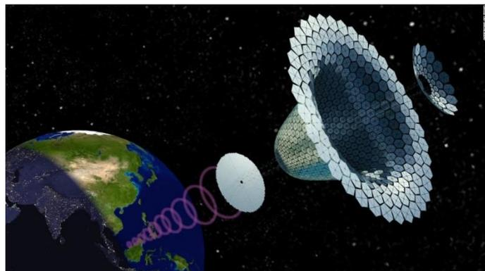
Figure 8 - A rendering of NASA's SPS-ALPHA 2012 (Mankins, 2012)
