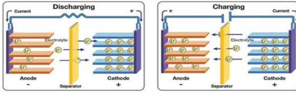
*Figure 12: Representation of the operation of a Lithium-ion battery (Research & Development, 2017)*
