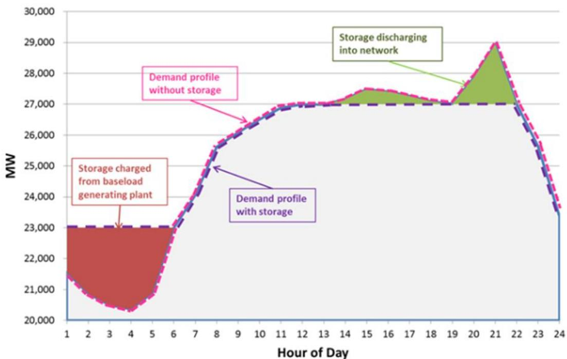
*Figure 8: Representation of the change of the demand profile using storage over a day*
