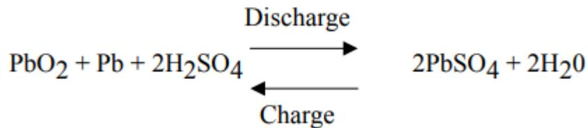
*Equation 1: Chemical reactions within a lead-acid cell (Dietel, 2011)*
