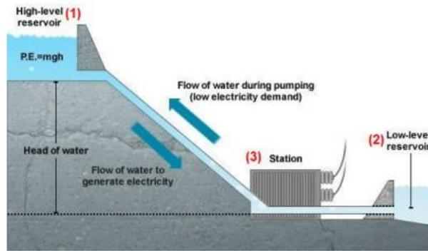
*Figure 11: Hydro Pump Storage Operating System (American Society of Civil Engineers, 1996)*
