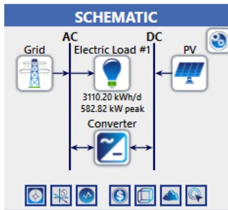
*Figure 33: Configuration of the Capileira power system PV capacity*
