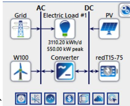
*Figure 63: Configuration of the energy system of Capileira with the use of storage*
