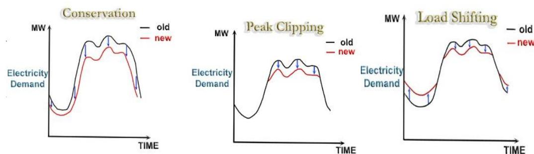
*Figure 6: Representation of different measures to smooth out demand peaks (Esru.strath.ac.uk, 2017)*
