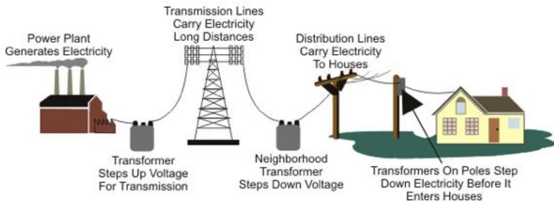
*Figure 1: conventional electrical network transmission (Solanki,2017)*
