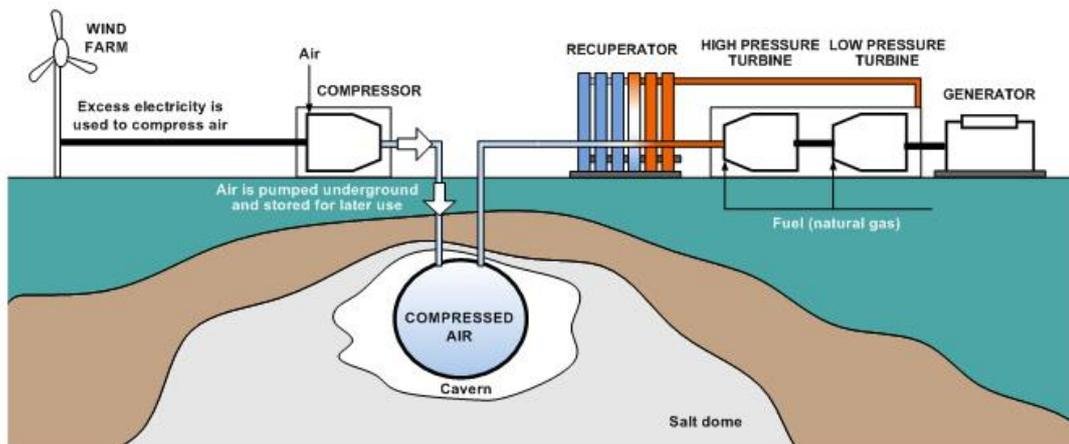
*Figure 10: Possible configuration of a CAES system (Sc.ehu.es, 2017)*
