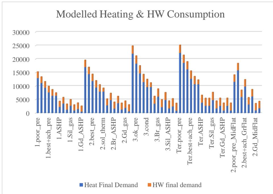
Figure 58 - Heating energy consumption from HEM modelling
