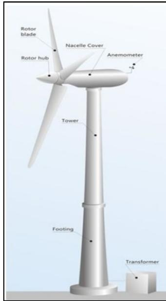
**Figure 5:** Wind turbine components (Cao, Xie and Tan, 2012)
