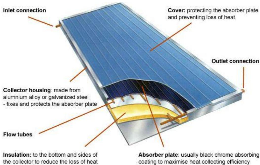
Figure 4: Flat plate collector elements (Source: GreenSpec, 2016)
