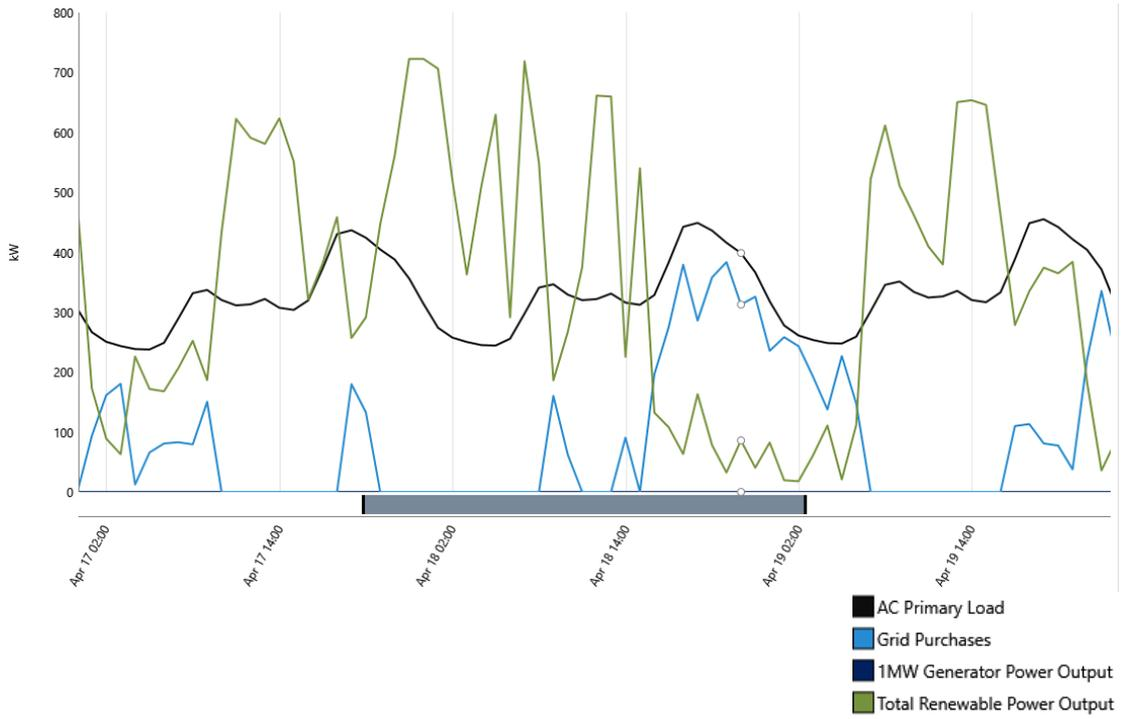
Fig 12. Power against time of wind-diesel-grid system
