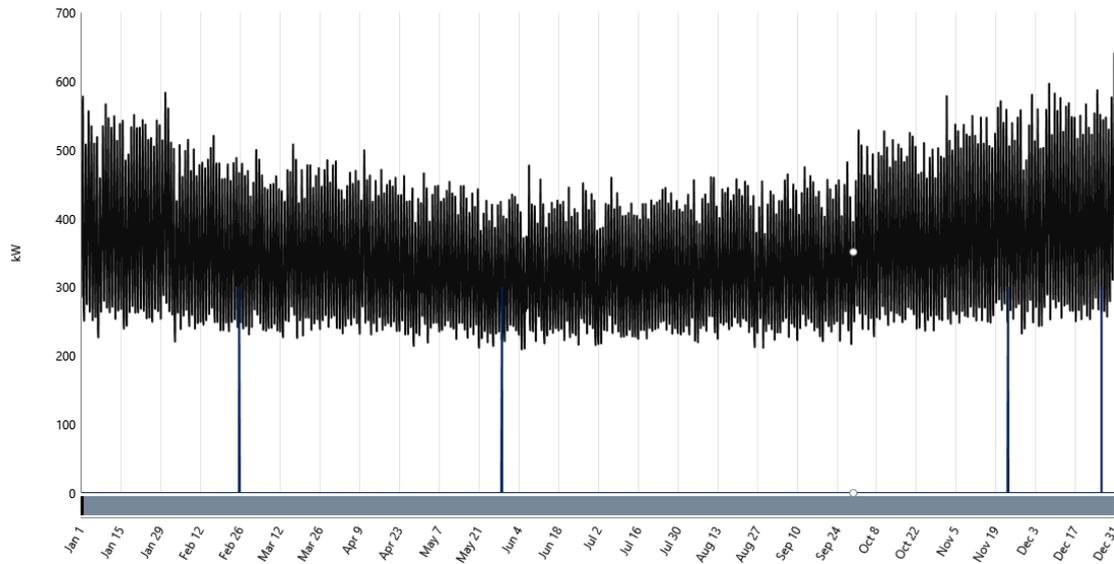
Fig 16. Operation of Diesel Generator (represented as blue lines) and demand profile
