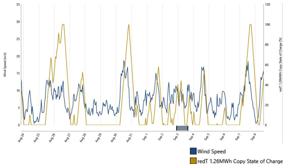
Fig 19. Effect of wind speed on battery's state of charge
