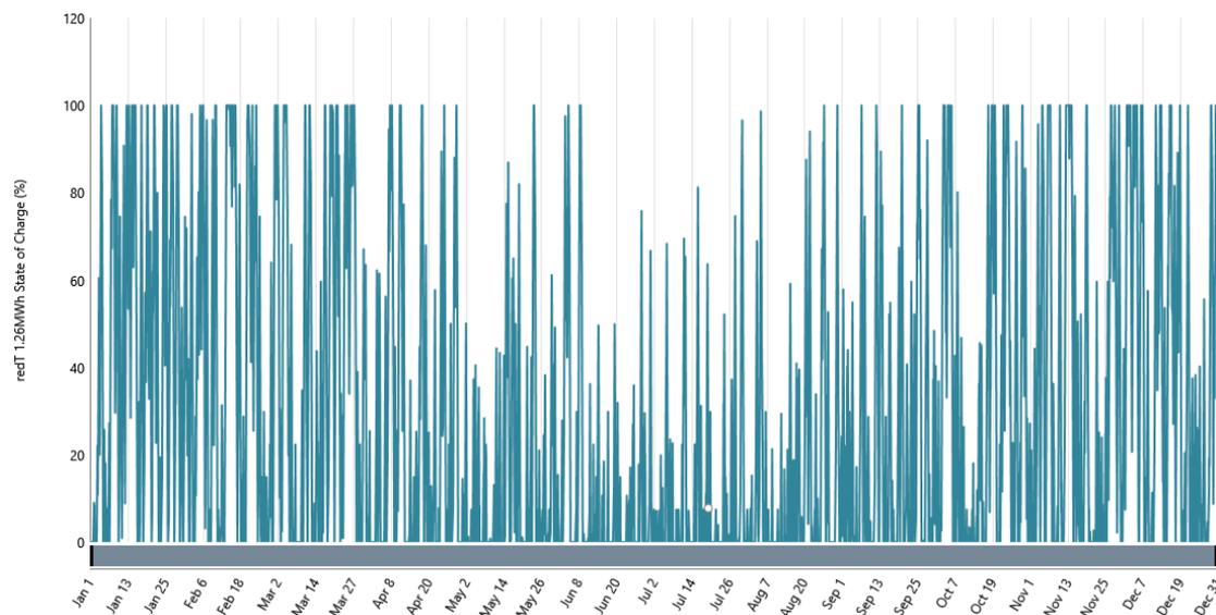
Fig 22. 105kW, 1260kWh battery's state of charge over a year
