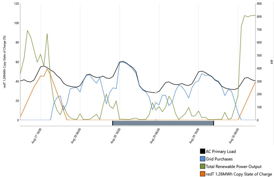
*Fig 20. Grid Imports during times of low power generation*
