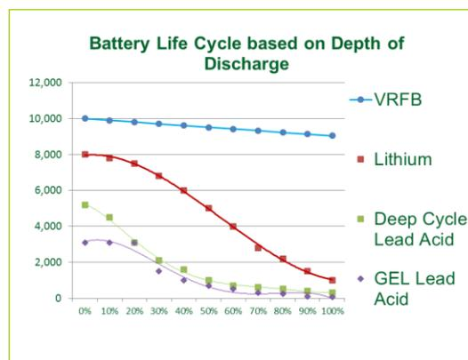
Fig 18. Comparison of different storage types based on their battery life cycle against depth of discharge <sup>[19]</sup>
