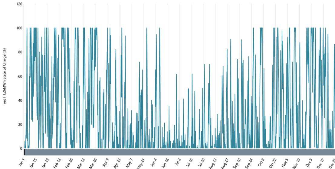
Fig 23. 420kW, 5040kWh battery's state of charge over a year
