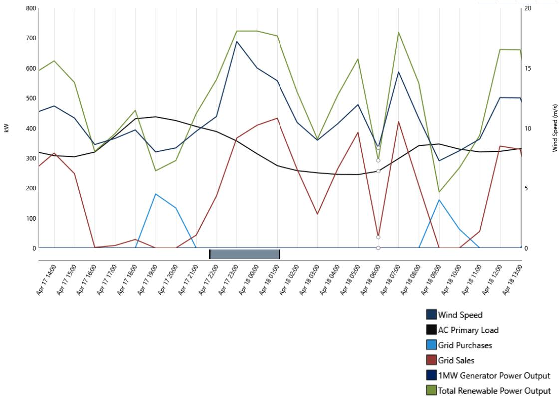
Fig 13. Graph showing rise in grid sales due to rise in wind speed
