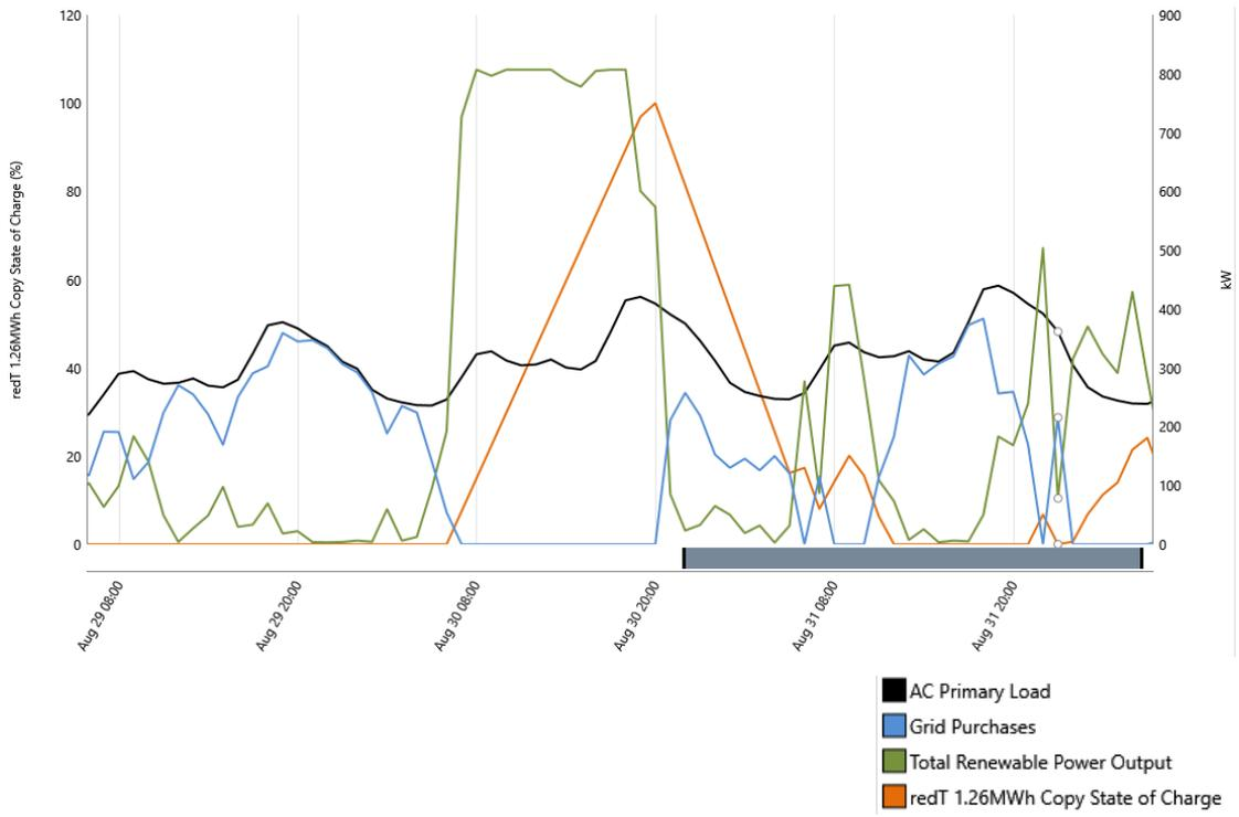
Fig 21. Power from grid and storage used to serve load after 8pm
