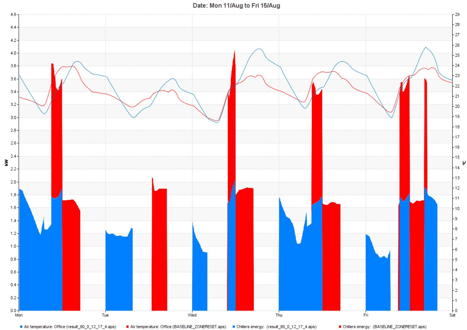
Figure 62: Result of MPC showing demand limiting and peak shifting, compared to the baseline. It also shows the zone temperature for the day. (red baseline, blue MPC)
