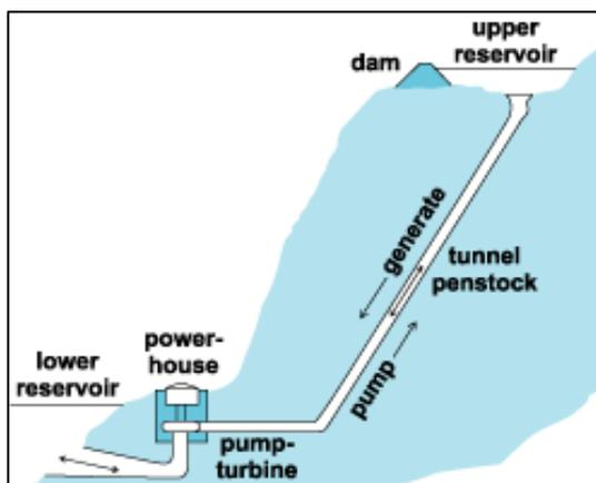
water from the upper reservoir can be released and allowed to flow back through to the lower reservoir to produce electricity. Though this type of system is a net user of power it provides a dynamic and rapid response when a heavy load is
