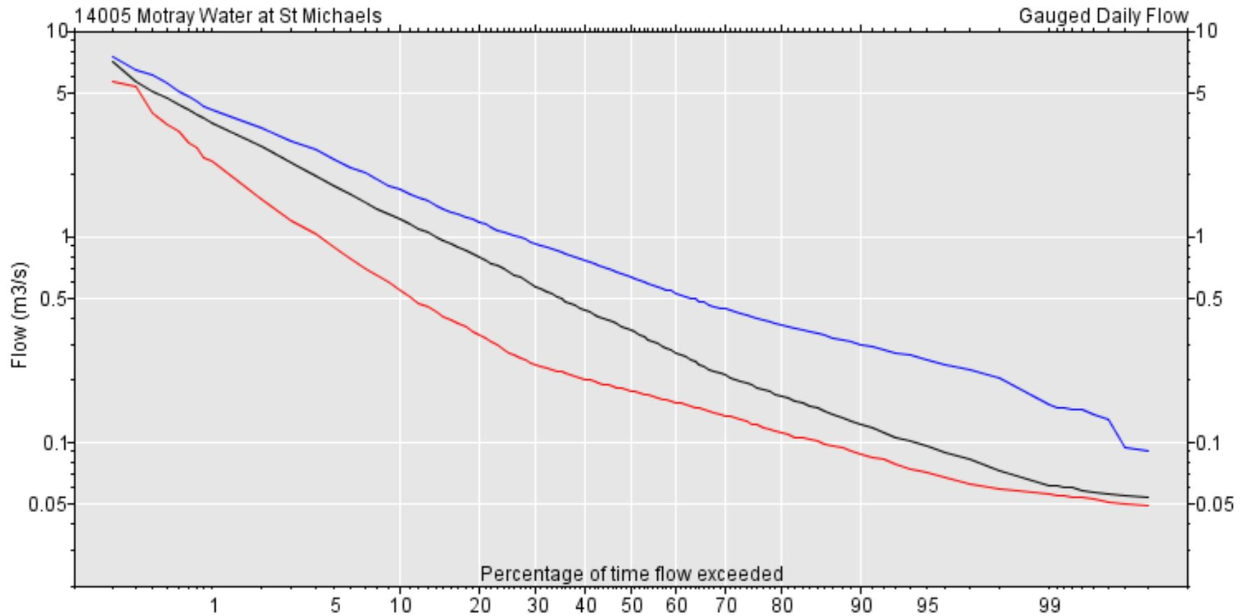
Figure 20: Flow Duration Curve for the Motray Water (2014)
