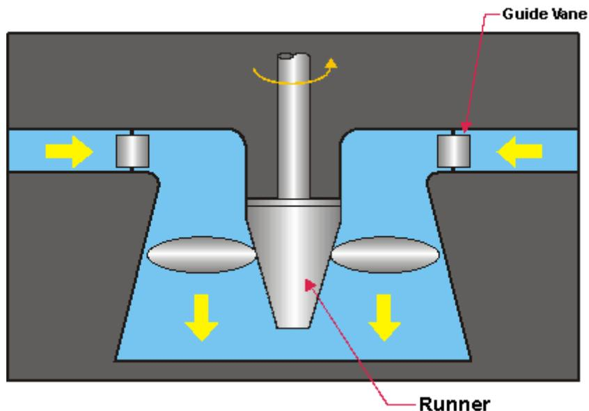
*Figure 12: Propeller Turbine*
