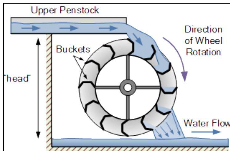
*Figure 15: Overshot Waterwheel Operation*
