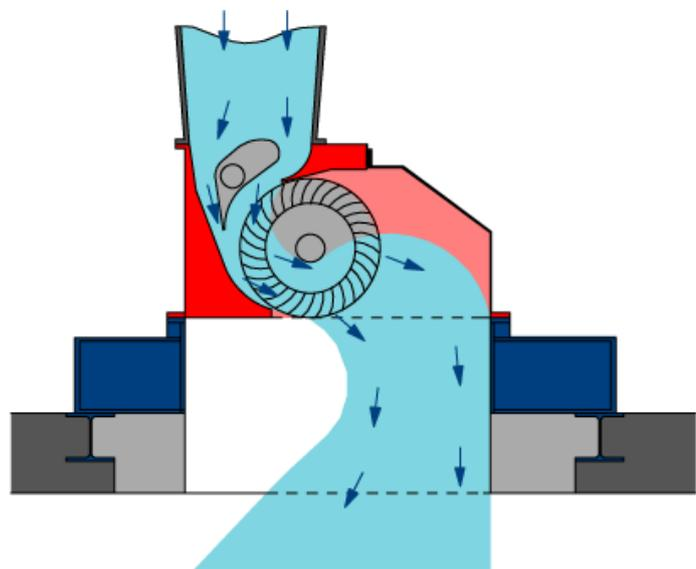
Figure 11: Crossflow Turbine
