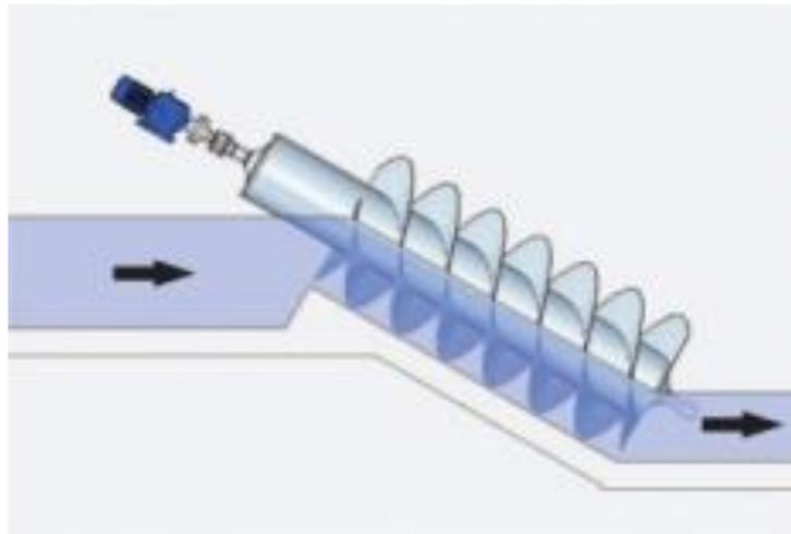
*Figure 16: Reverse Archimedes Screw*
