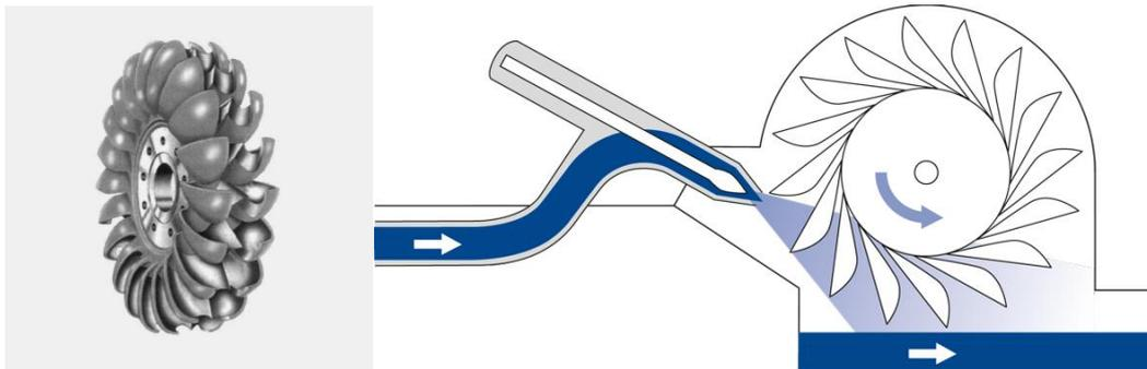
Figure 9: Pelton turbine and its operation
