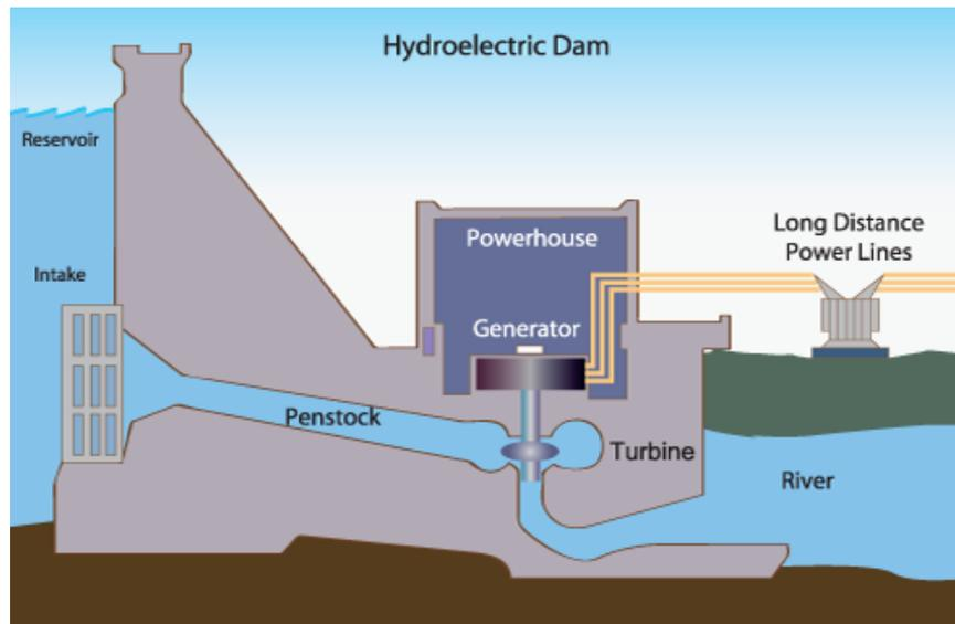
Figure 6: Operation of a hydroelectric dam
