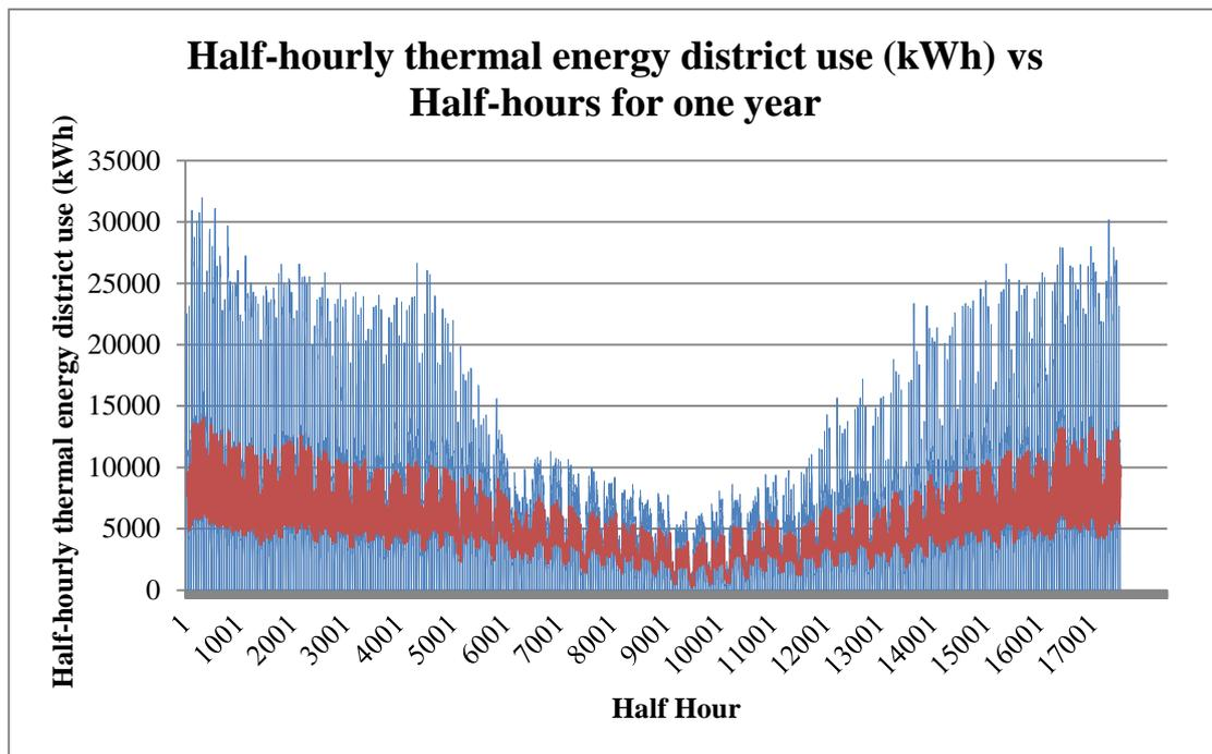
*Figure 36: Thermal demand profile of proposed site*
