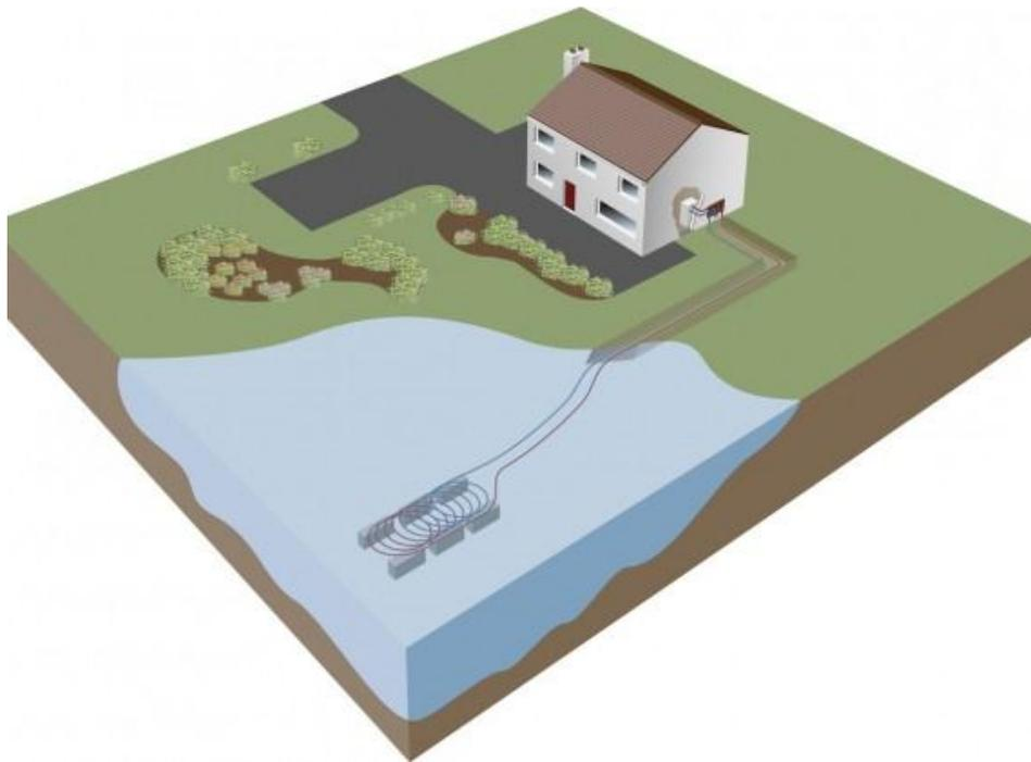
*Figure 5: Closed-loop water source heat pump graphic (KensaHeatPumps, 2015)*
