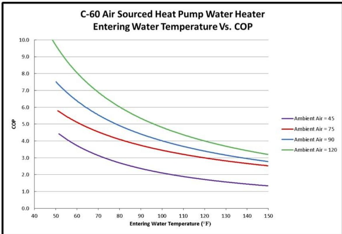
Figure 4: Relationship between COP and outlet temperature (Mathissen, 2011)
