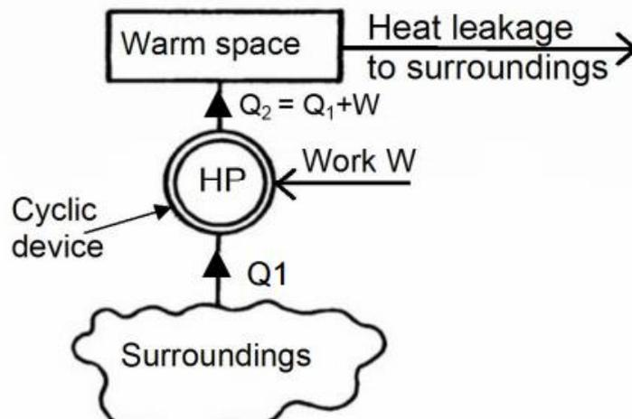
Figure 1: Heat pump schematic (Tuohy, 2008)
