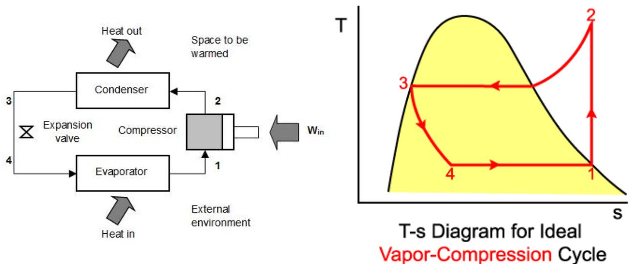
Figure 2: Simple vapour-compression component cycle, T-S diagram for cycle (Tuohy, 2008), (Moran, 2015)
