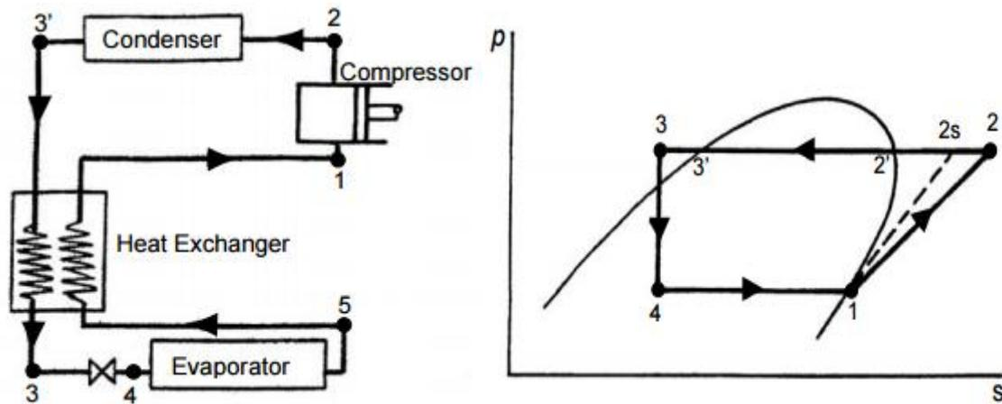
Figure 3: Realistic vapour-compression cycle, with heat exchanger (Tuohy, 2008)
