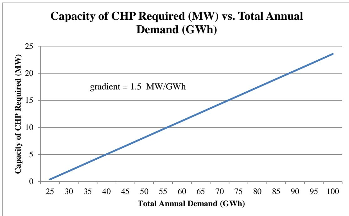
Figure 39: Capacity of CHP required vs. Annual demand
