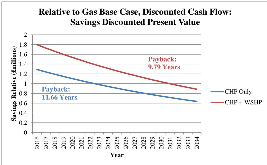
Figure 51: Discounted cash flow, Comparison to Gas
