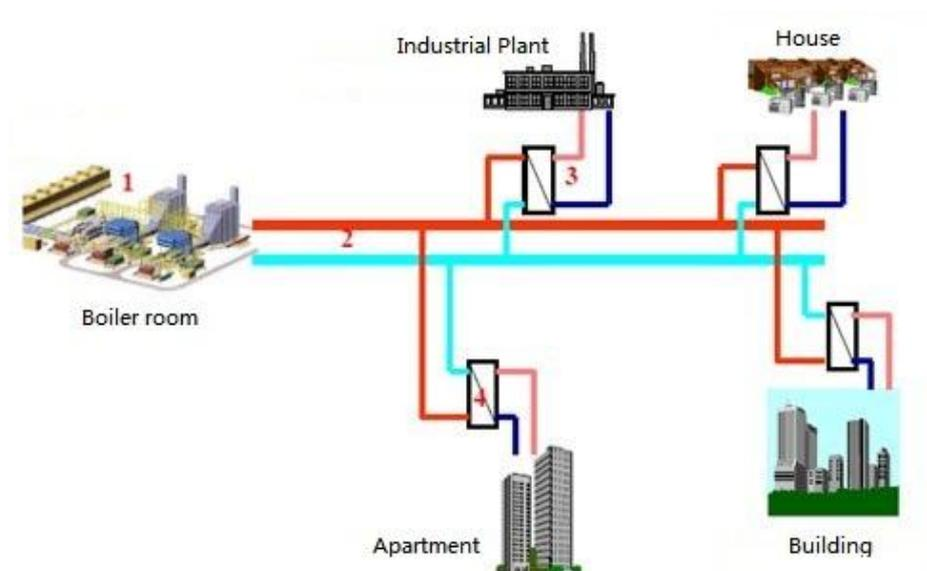
Figure 8: Simple schematic of district heating (SmartHeat, 2012)
