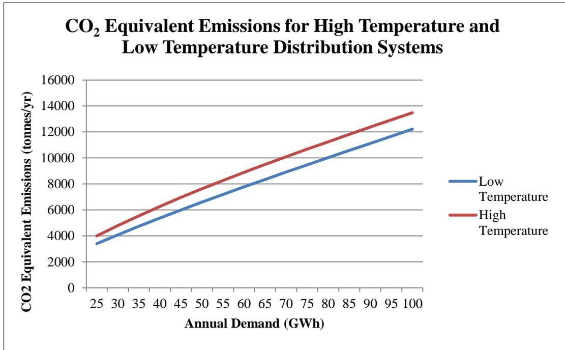
Figure 47: CO<sub>2</sub> emissions: Distribution systems
