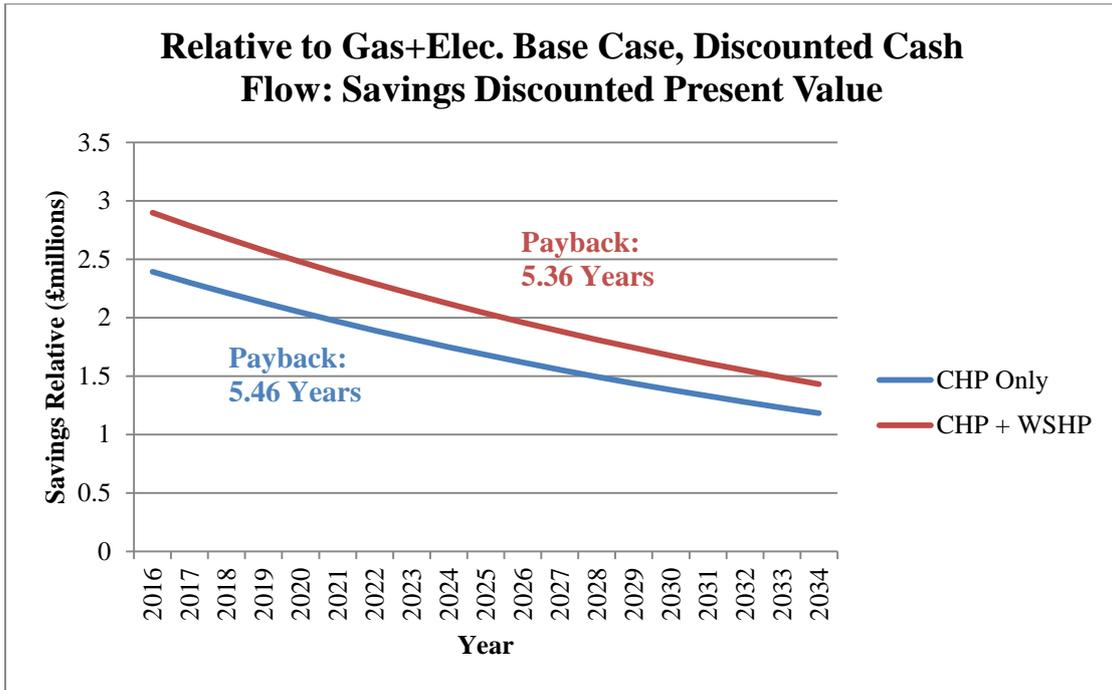
Figure 52: Discounted cash flow, Comparison to Gas + Elec.
