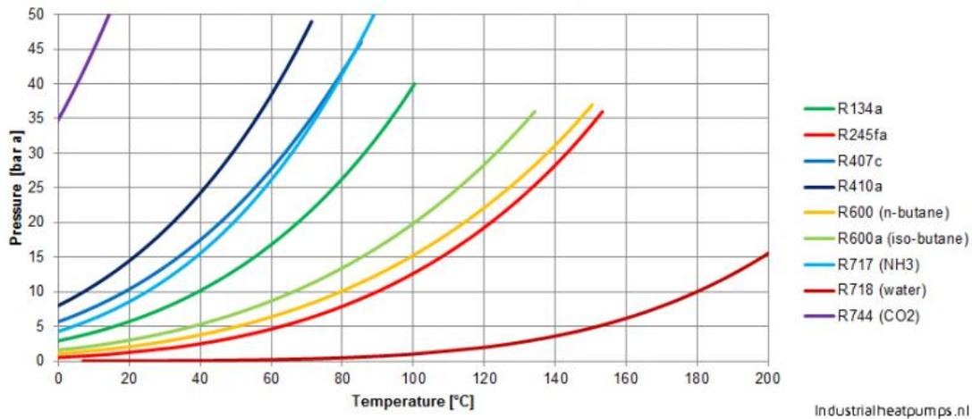
Figure 6: Comparison of refrigerants (*IndustrialHeatPumps, 2012*)
