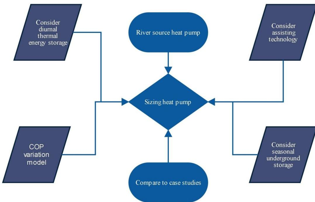
*Figure 18: River source heat pump flow diagram*
