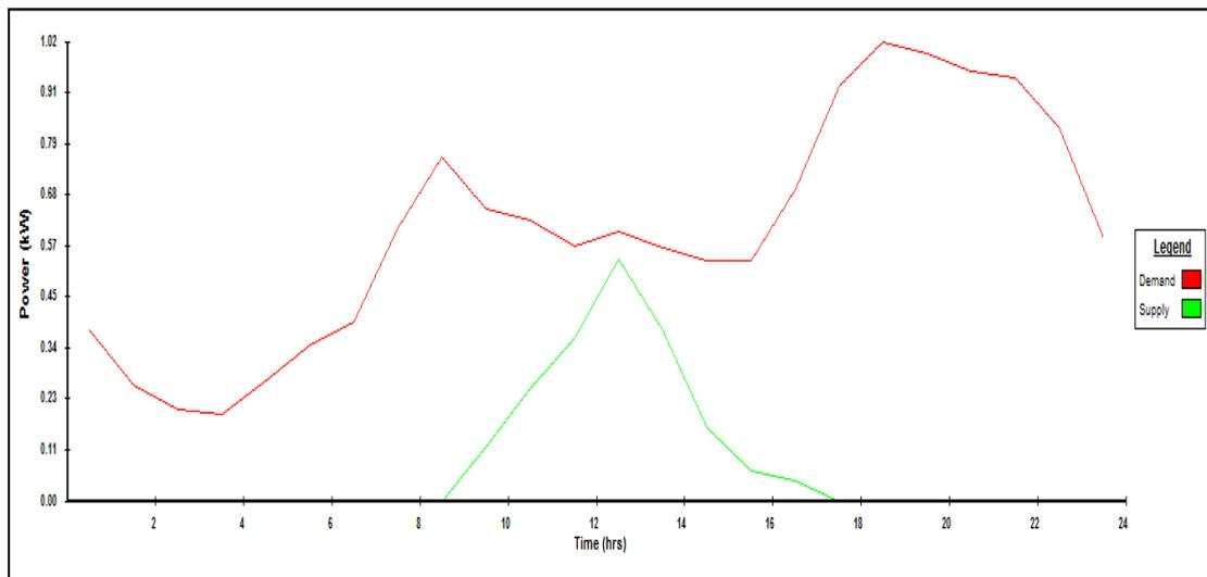
Graph 13: DSM simulation during 1<sup>st</sup> of February (35 panels, 0.130kW BP)
