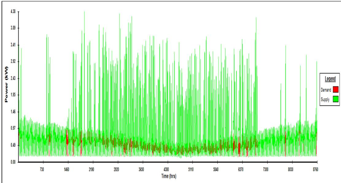
Graph 21: DSM simulation (30 panels, 0.130kW BP @ 60° plus 32 Batteries plus Generic 1kW WT)
