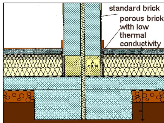
Figure 6: Thermal bridge free construction in slab on grade
