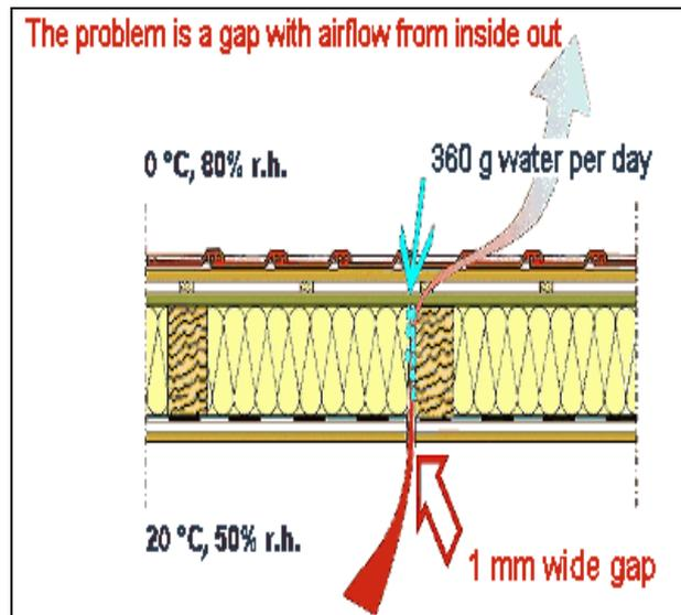
Figure 7: Water condensation at the coldest part of the construction material
