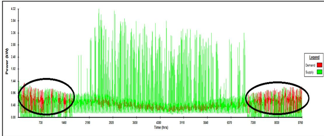
Graph 12: DSM simulation (35 panels, 0.130kW BP plus 16 Batteries)
