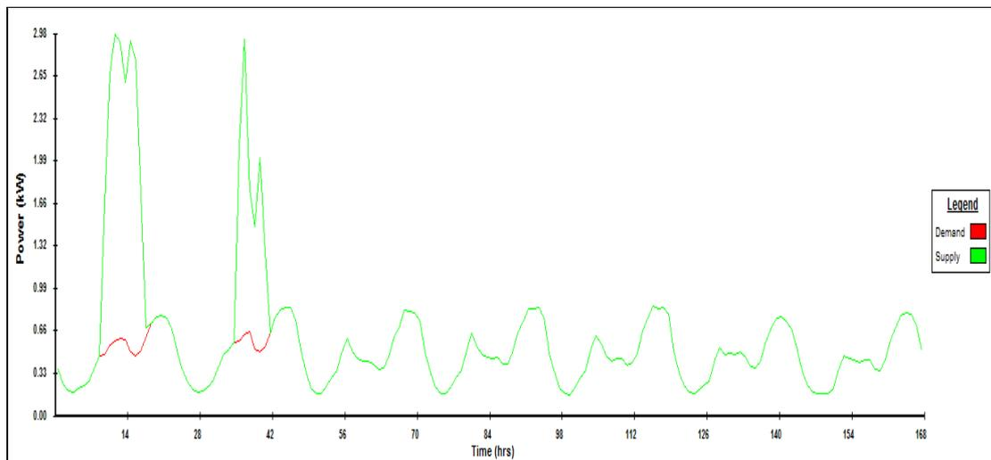
Graph 17: DSM simulation during 1st week of October (35 panels, 0.130kW BP plus 16 Batteries)
