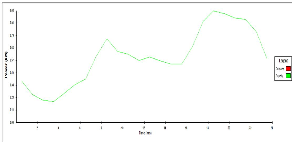
Graph 14: DSM simulation during 1st day of February (35 panels, 0.130kW BP plus 16 Batteries)
