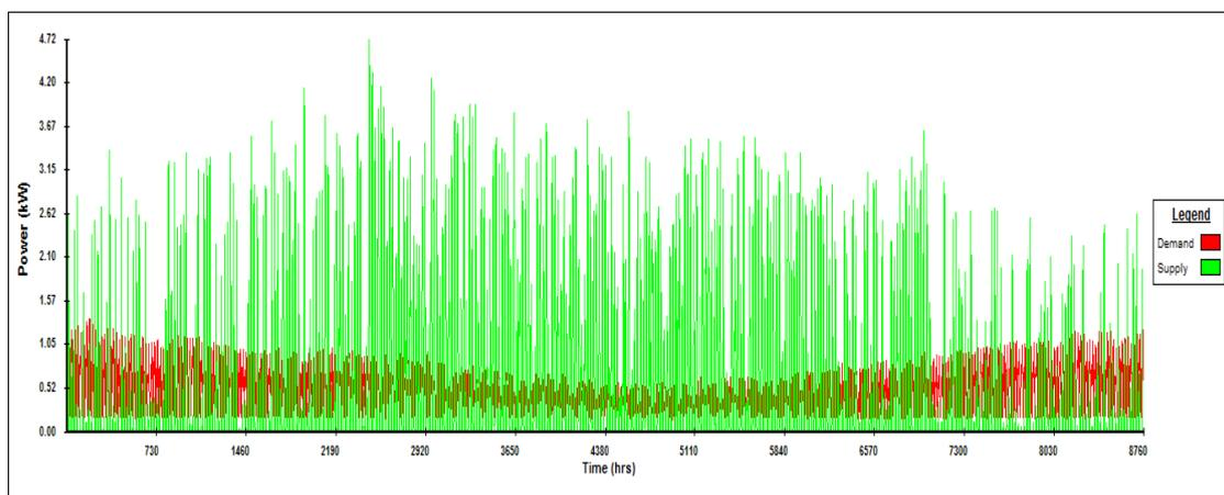
Graph 11: DSM simulation (35 panels, 0.130kW BP)
