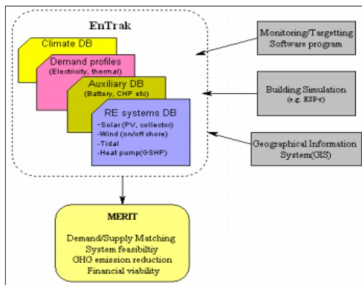
Figure 18: Merit's simulation procedure
