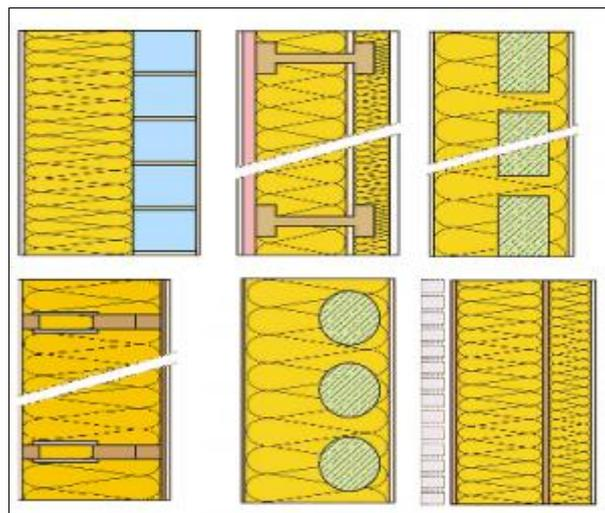
Figure 4: Super insulated walls suitable for passive houses.
