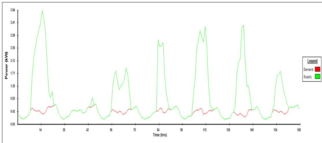
Graph 16: DSM simulation during 1st week of June (35 panels, 0.130kW BP plus 16 Batteries)
