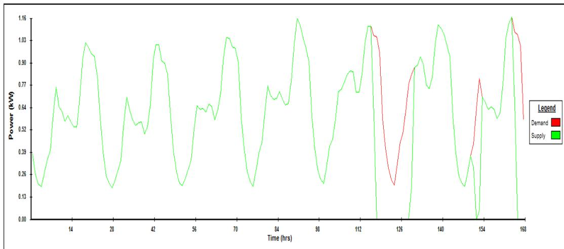
Graph 15: DSM simulation during 1st week of February (35 panels, 0.130kW BP plus 16 Batteries)
