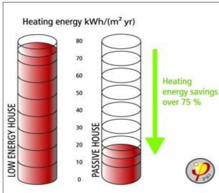
Figure 1: Reduction on energy demand due to passive house standards construction.
