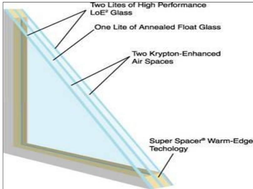
Figure 11: Window with multiple panes, Gas fill and warm spacer
