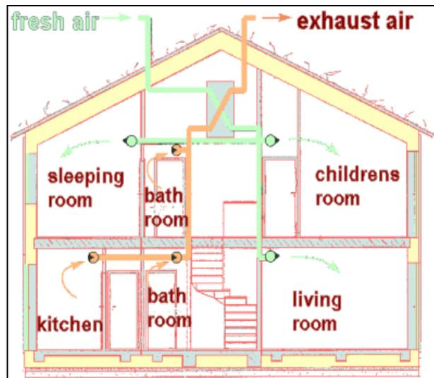
Figure 10: Ventilation system with heat recovery
