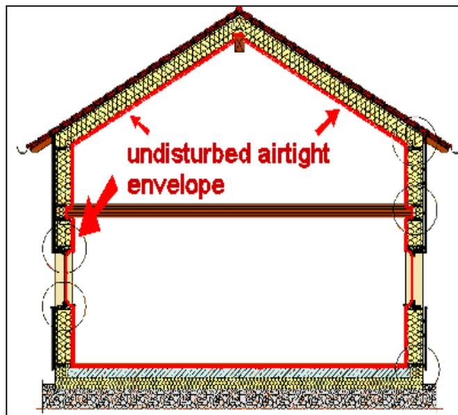
Figure 8: Air tight construction
