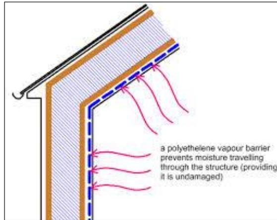
Figure 9: Vapour barrier
