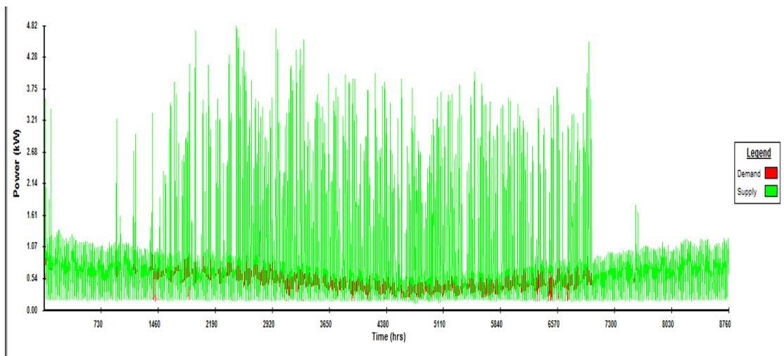
Graph 20: DSM simulation (36 panels, 0.130kW BP @ 60° plus 40 Batteries plus Generic 0.6kW WT)
