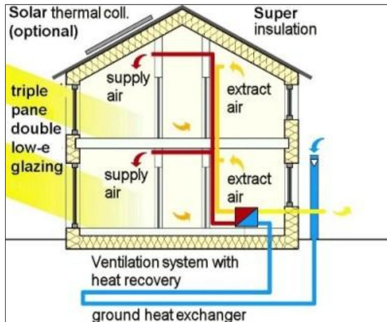
Figure 2: Typical passive house arrangement.
