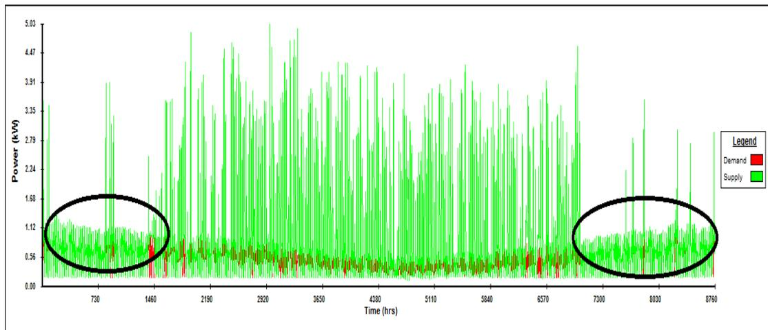
Graph 18: DSM simulation (35 panels, 0.130kW BP plus 36 Batteries plus Generic 1kW WT)
