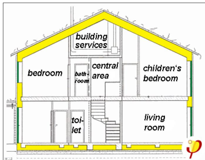
Figure 5: Thermal bridge free design
