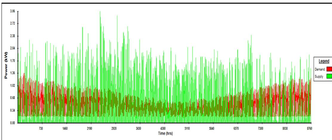
Graph 10: DSM simulation results (31 panels 0.110kW Mono)
