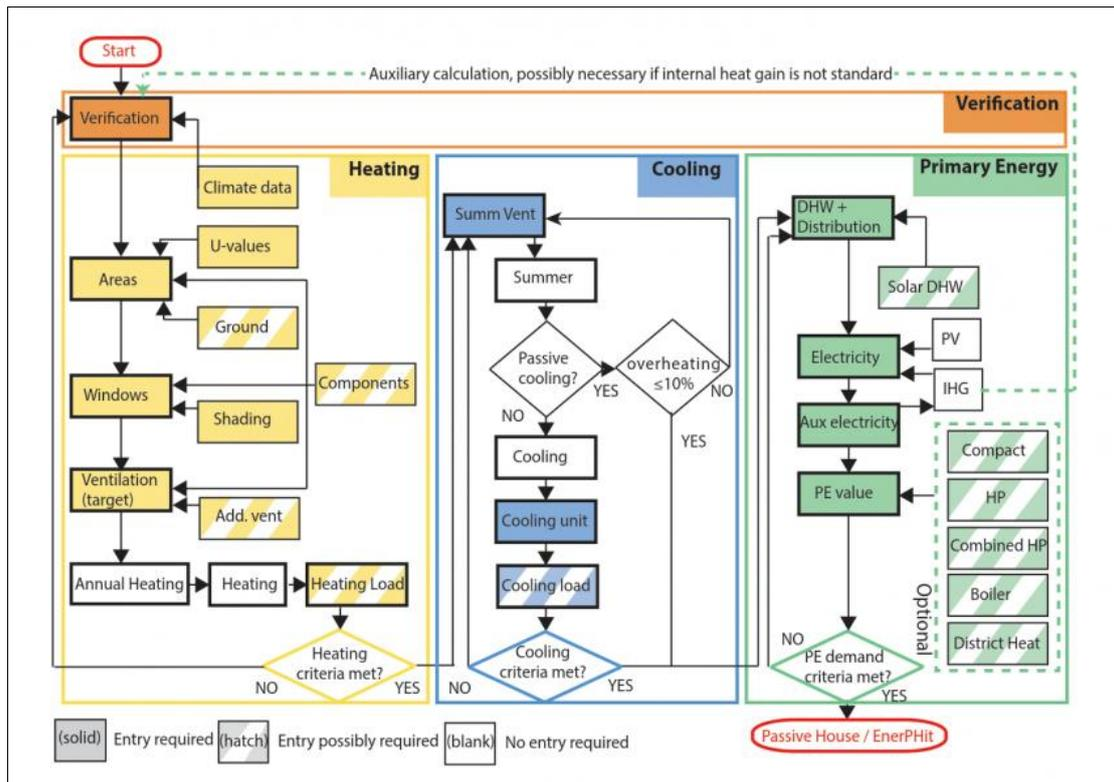
Figure 13: PHPP verification process flow chart
