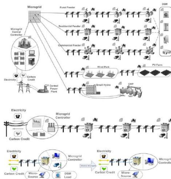
Figure 1.1 (a) Microgrid as a LV grid; (b) Microgrid as a LV feeder; (c) Microgrid as a LV house
