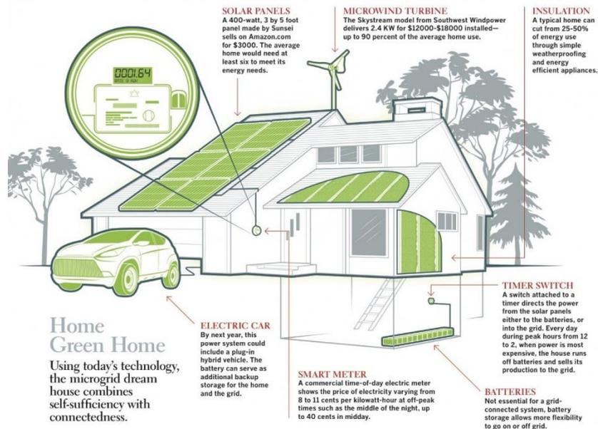
Figure 2 Example of a Single house microgrid (Fast Company, 2011)
