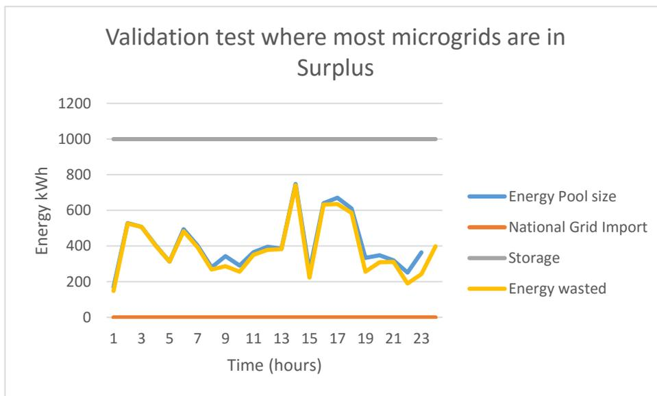
Figure 15 - Extreme Case 2 Pool size, grid import, storage and energy wasted
