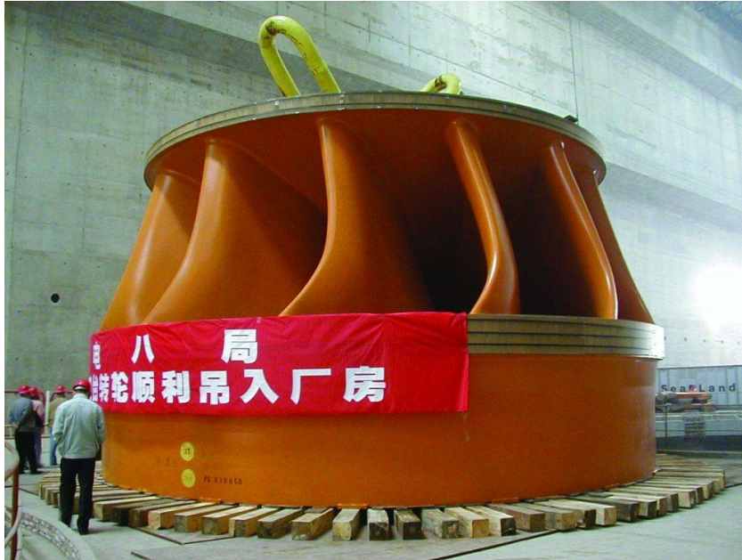
Figure 4 Photograph of Large Francis Turbine
