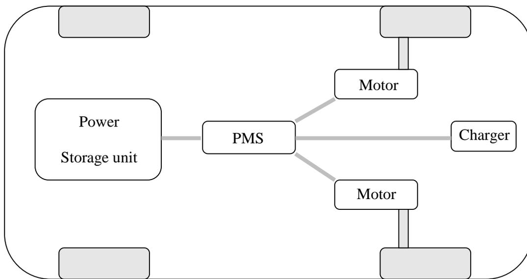
**Figure 4.** Basic EV powertrain with key components.
