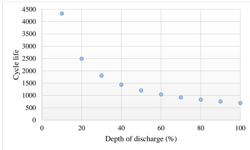
**Figure 7.** Li ion cycle life as a function of depth of discharge (Zhou 2011).
