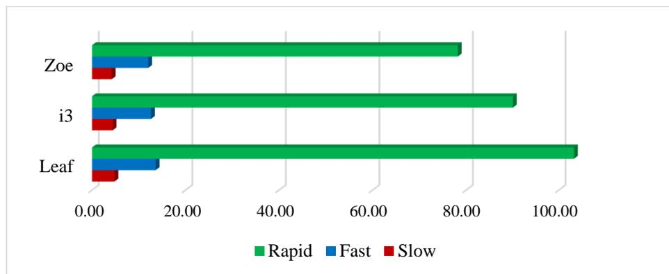
**Figure 8.** Electric range achieved in thirty minute charge at different recharge speeds.
