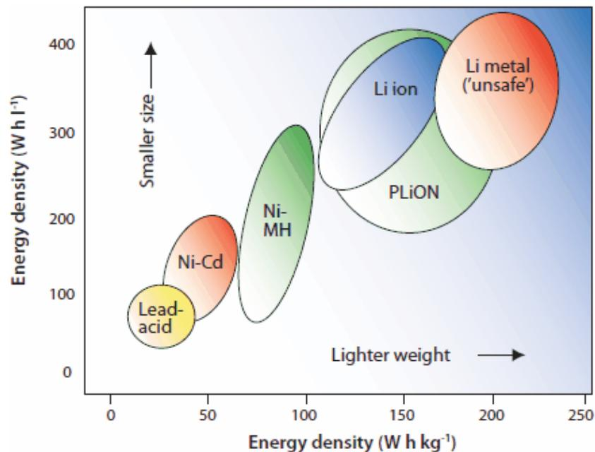
**Figure 5.** Energy density of battery chemistries, both volumetric and mass.
