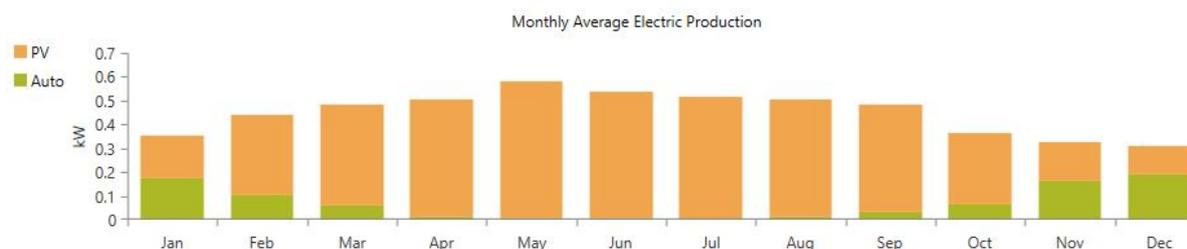
Figure 54 – Electricity Production for Trojan IND29-4V with PV (stand-alone) System in Aberdeen
