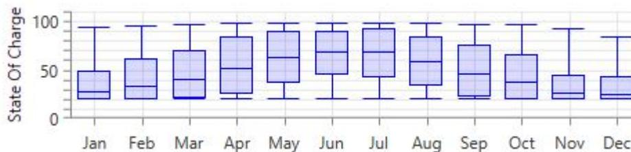
Figure 58 – Discover 6VRE-2400TG SOC for PV (stand-alone) System in Aberdeen
