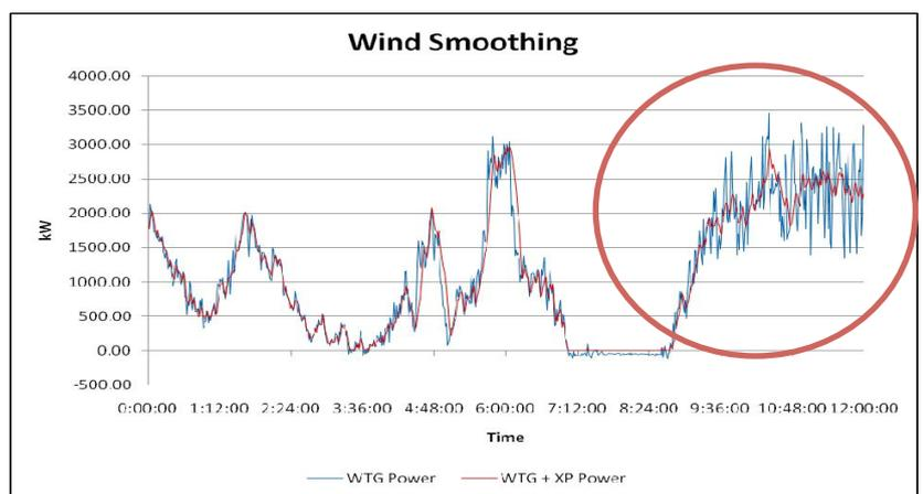
Figure 4 – Energy Storage capabilities of smoothing wind output. (Such & Hill, 2012, p .3)
