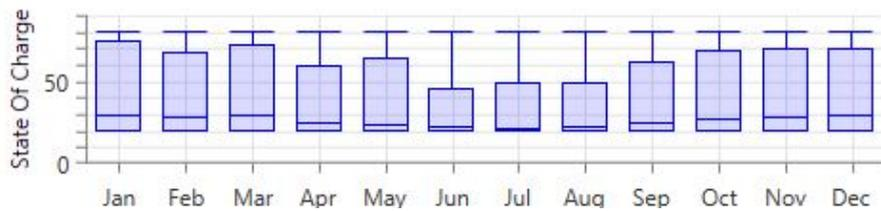
Figure 36 – SAFT Intensium Home SOC for Wind (grid-connected) System in Aberdeen
