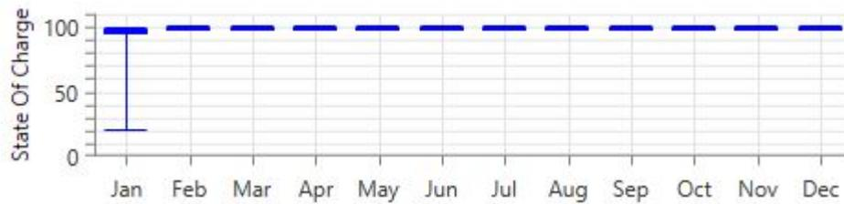
Figure 14 – Trojan IND29-4V SOC for PV (grid-connected) System in San Francisco
