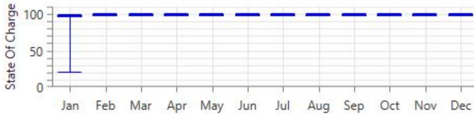
Figure 13 – Trojan IND17-6V SOC for PV (grid-connected) System in San Francisco
