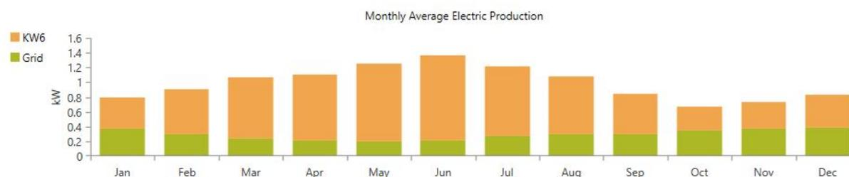
Figure 19 – Electricity Production for Discover 6VRE-2400TG with Wind (grid-connected) System in San Francisco
