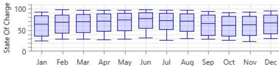
Figure 46 – Trojan IND29-4V SOC for Wind (stand-alone) System in San Francisco
