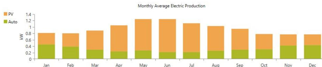
Figure 40 – Electricity Production for Trojan IND29-4V with PV (stand-alone) System in San Francisco
