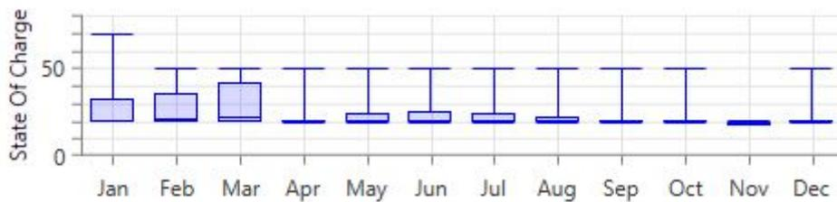
Figure 23 – LG Chem SOC for Wind (grid-connected) System in San Francisco
