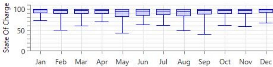
Figure 64 – Juicebox SOC for Wind (stand-alone) System in Aberdeen
