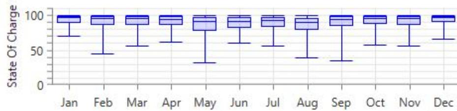
Figure 35 – Trojan IND29-4V SOC for Wind (grid-connected) System in Aberdeen
