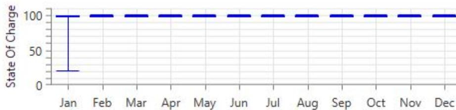
Figure 24 – Juicebox Energy SOC for Wind (grid-connected) System in San Francisco
