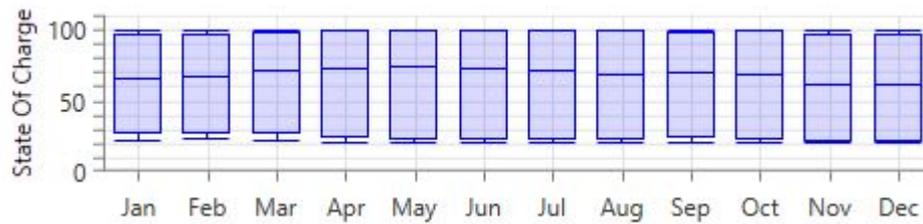
Figure 41 – SAFT Intensium Home SOC for PV (stand-alone) System in San Francisco
