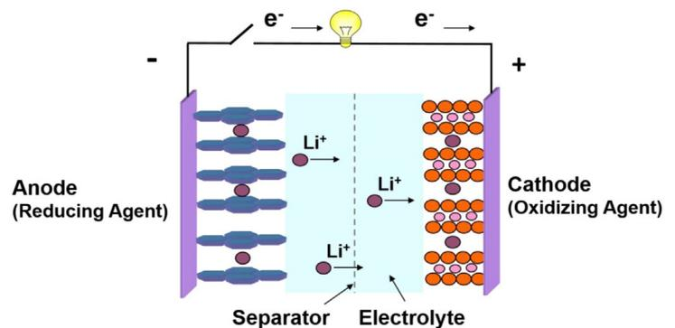
an electrochemical cell, lithium-ion for example, contains an anode, a cathode and an electrolyte. During charging, the anode oxidises, and electrons are given off, through the electrolyte, to the cathode, as shown above, in Figure 2.
