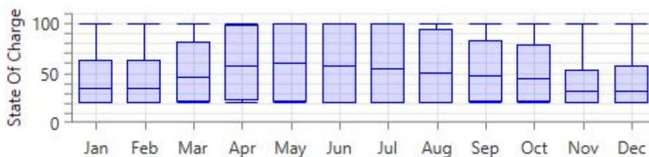
Figure 45 – LG Chem SOC for PV (stand-alone) System in San Francisco
