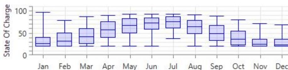
Figure 53 – Trojan IND29-4V SOC for PV (stand-alone) System in Aberdeen
