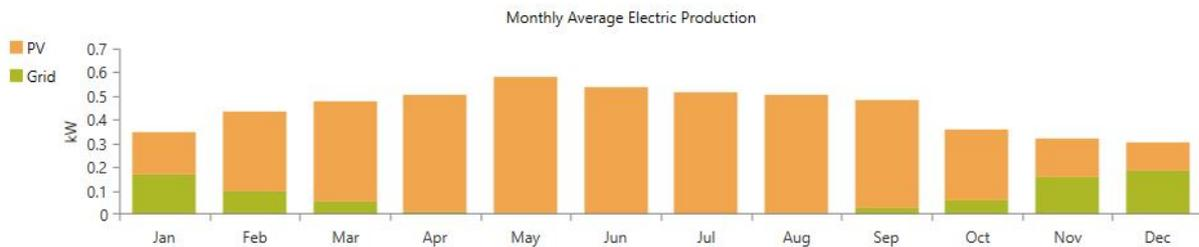
Figure 26 – Electricity Production for Trojan IND29-4V with PV (grid-connected) System in Aberdeen
