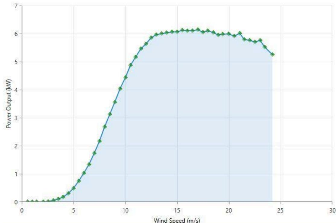
Figure 10 - KW6 Wind Turbine Power curve (data courtesy of Kingspan Wind)
