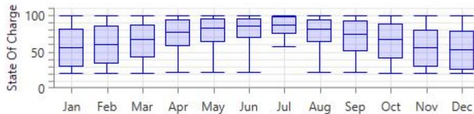
Figure 57 – Juicebox Energy SOC for PV (stand-alone) System in Aberdeen
