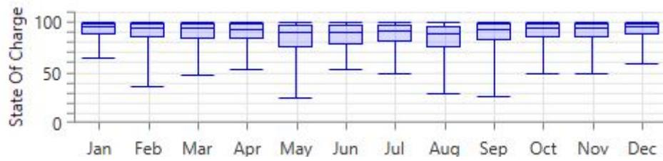
Figure 34 – Trojan IND17-6V SOC for Wind (grid-connected) System in Aberdeen
