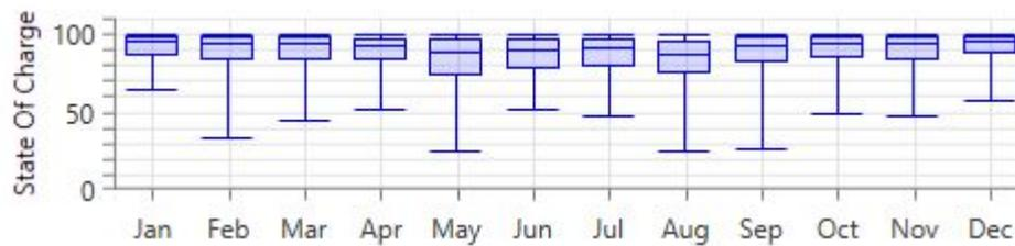
Figure 60– Trojan IND17-6V SOC for Wind (stand-alone) System in Aberdeen
