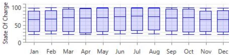
Figure 44 – Discover 6VRE-2400TG SOC for PV (stand-alone) System in San Francisco
