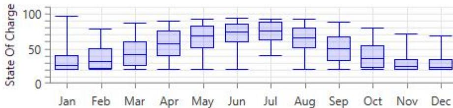
Figure 25 – Trojan IND29-4V SOC for PV (grid-connected) System in Aberdeen
