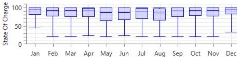
Figure 32 – Discover 6VRE-2400TG SOC for Wind (grid-connected) System in Aberdeen
