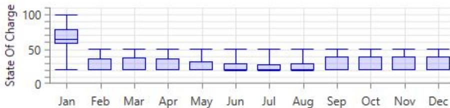
Figure 37 – LG Chem SOC for Wind (grid-connected) System in Aberdeen
