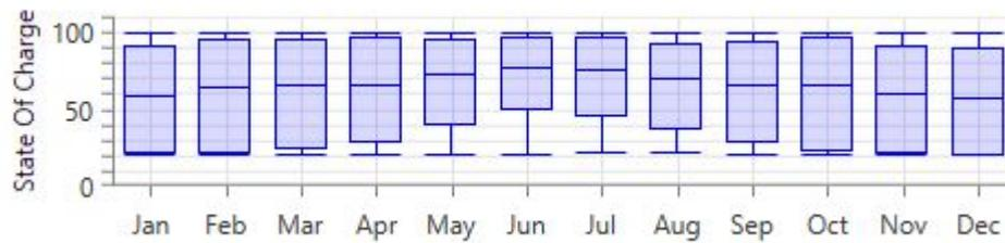
Figure 55 – SAFT Intensium Home SOC for PV (stand-alone) System in Aberdeen
