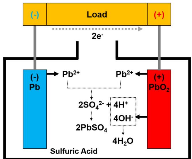
Figure 3 – Lead-Acid Battery (Cho et al. 2015, p.88)
