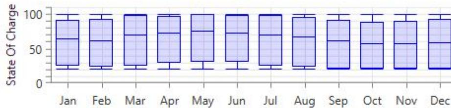
Figure 22 – SAFT Intensium Home SOC for Wind (grid-connected) System in San Francisco
