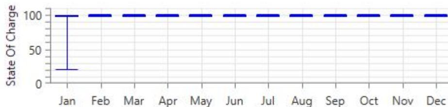
Figure 31 – Juicebox Energy SOC for PV (grid-connected) System in Aberdeen
