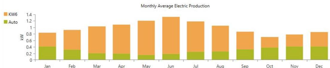
Figure 47 – Electricity Production for Trojan IND29-4V with Wind (stand-alone) System in San Francisco
