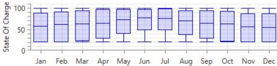
Figure 29 – SAFT Intensium Home SOC for PV (grid-connected) System in Aberdeen
