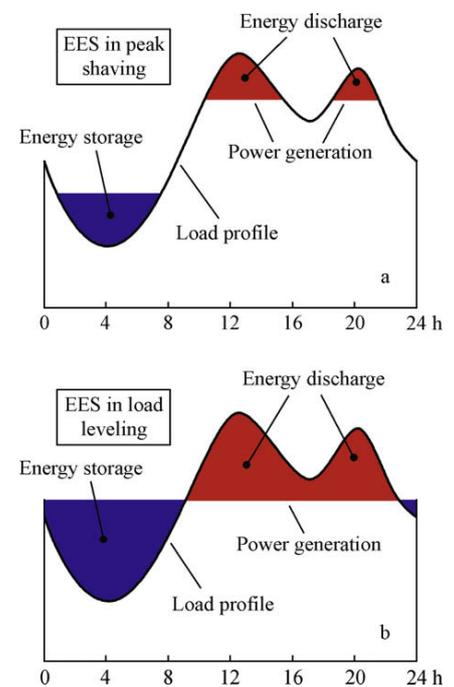
Figure 1 – Peak shaving and load levelling capabilities of energy storage system. (Chen et al. 2009, p. 292)
