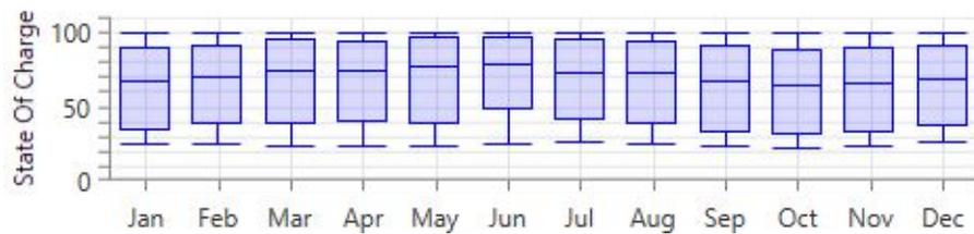
**Figure 51 – Discover 6VRE-2400TG SOC for Wind (stand-alone) System in San Francisco**
