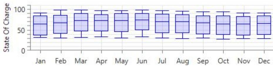
**Figure 49 – Trojan IND17-6V SOC for Wind (stand-alone) System in San Francisco**
