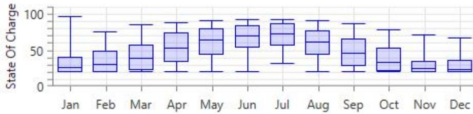
Figure 27 – Trojan IND17-6V SOC for PV (grid-connected) System in Aberdeen
