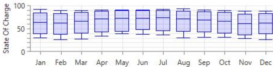
Figure 42 - Trojan IND17-6V SOC for PV (stand-alone) System in San Francisco
