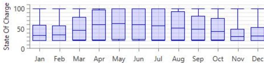
Figure 43 – Juicebox Energy SOC for PV (stand-alone) System in San Francisco
