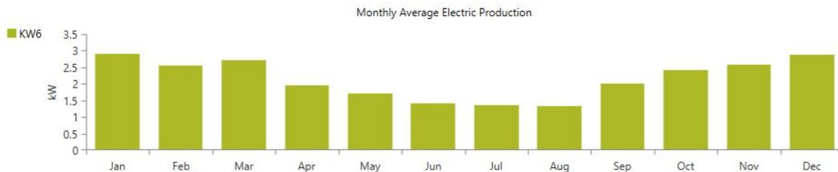
Figure 61 – Electricity Production for Trojan IND17-6V with Wind (stand-alone) System in Aberdeen
