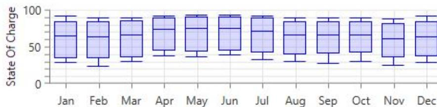
Figure 39 – Trojan IND29-4V SOC for PV (stand-alone) System in San Francisco
