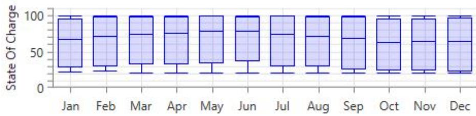
**Figure 48 – SAFT Intensium Home SOC for Wind (stand-alone) System in San Francisco**
