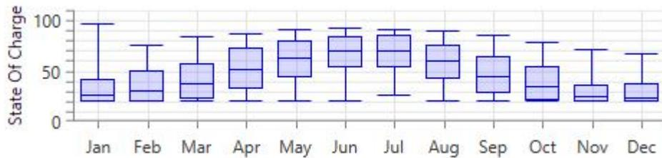
Figure 56 – Trojan IND17-6V SOC for PV (stand-alone) System in Aberdeen
