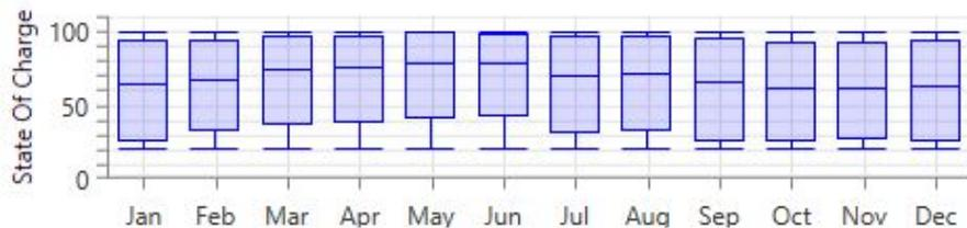
**Figure 52 – LG Chem SOC for Wind (stand-alone) System in San Francisco**
