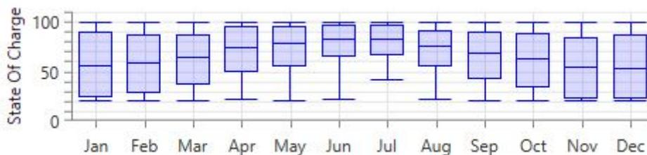
Figure 59 – LG Chem SOC for PV (stand-alone) System in Aberdeen
