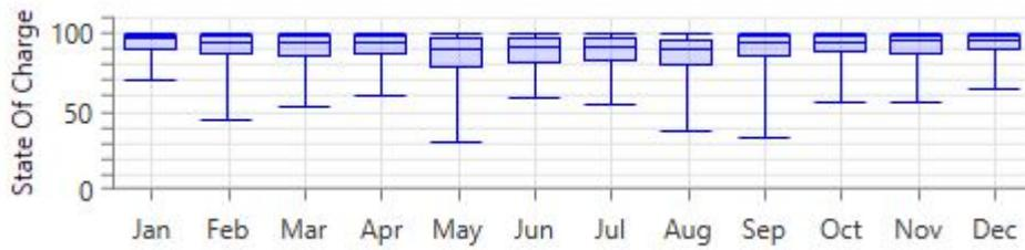
Figure 62 – Trojan IND29-4V SOC for Wind (stand-alone) System in Aberdeen
