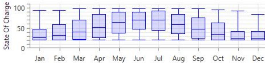
Figure 28 – Discover 6VRE-2400TG SOC for PV (grid-connected) System in Aberdeen
