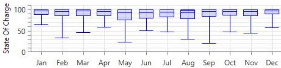
Figure 63 – LG Chem SOC for Wind (stand-alone) System in Aberdeen
