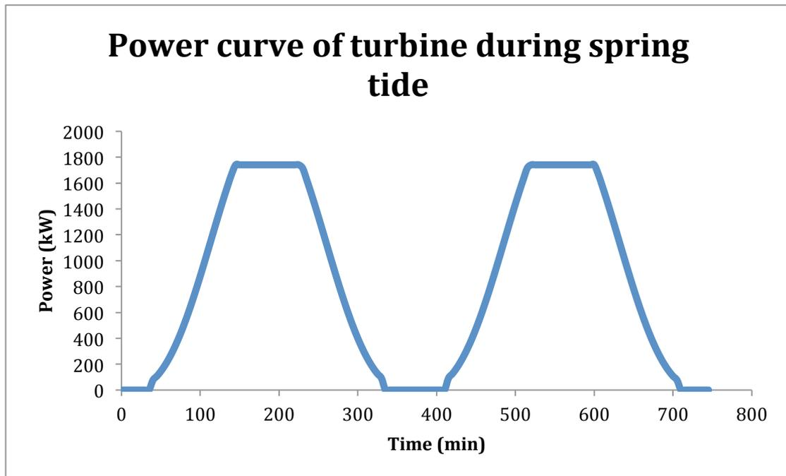
Figure 34 – Power obtained from 1 tidal turbine during spring tides
