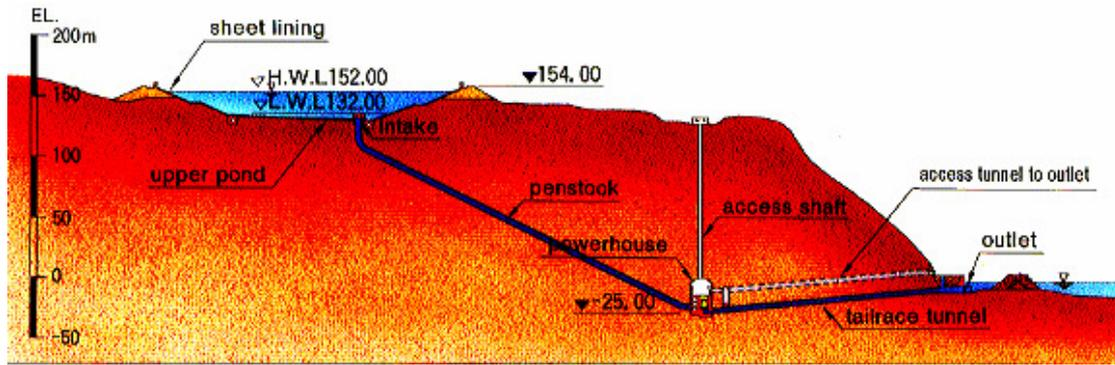
Figure 5 – Cross section of Okinawa PHS [12]
