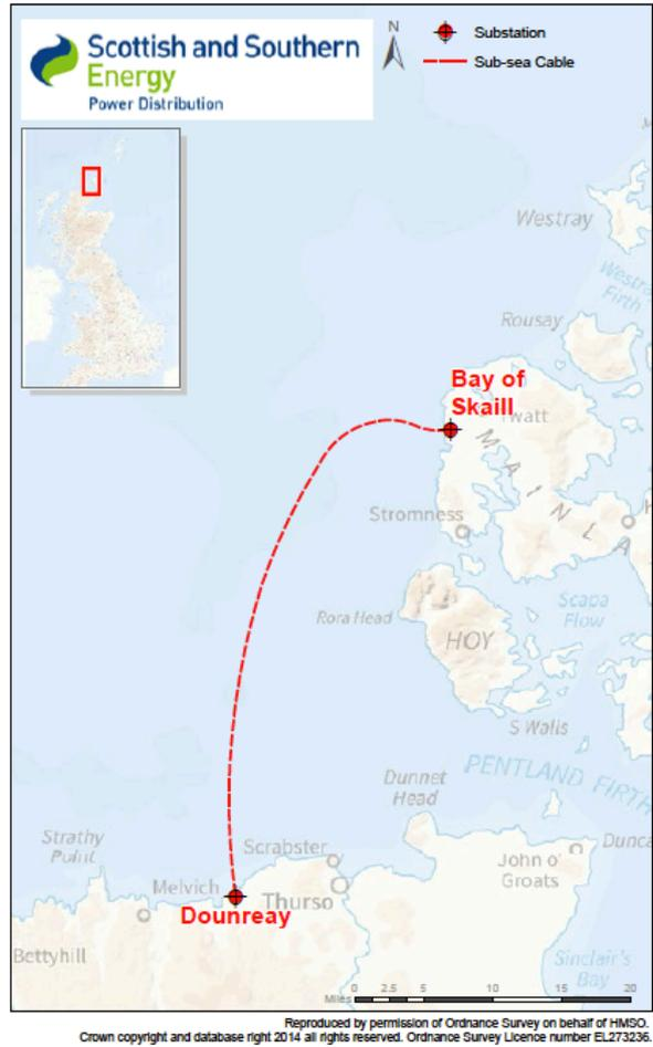
Figure 25 – Layout of proposed 180MW AC cable [25]
