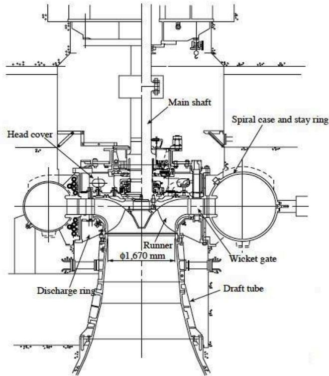
Figure 7 – Sectional view of pump turbine [13]
