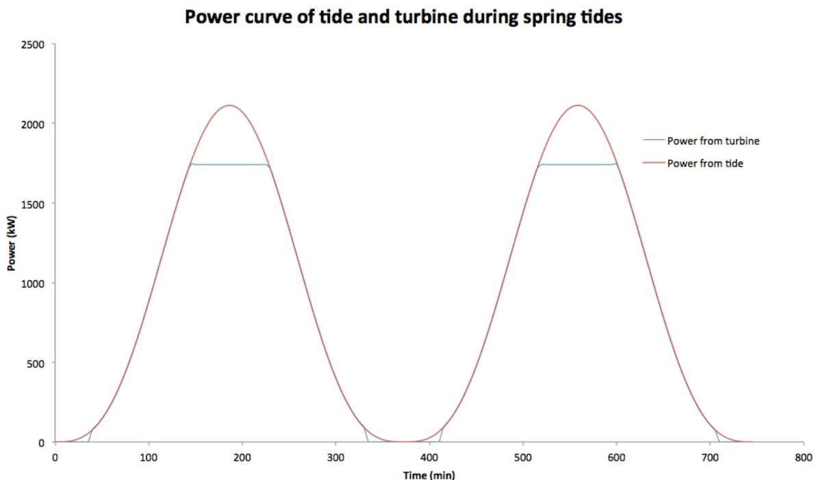
Figure 36 – Power curve of tide and turbine during spring tides
