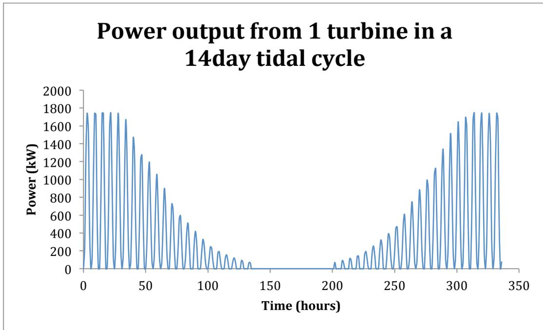
Figure 32 – Power output from 1 tidal turbine for the 14day tidal cycle used
