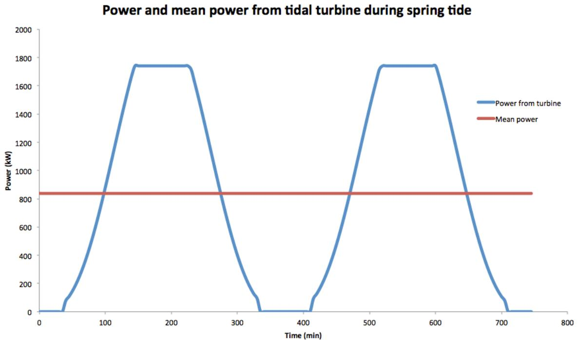
Figure 37 – Power and mean power from tidal turbine during spring tide
