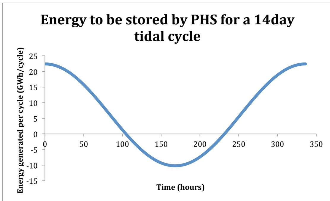
Figure 38 – Energy to be stored by PHS per cycle over time for a 14day tidal cycle
