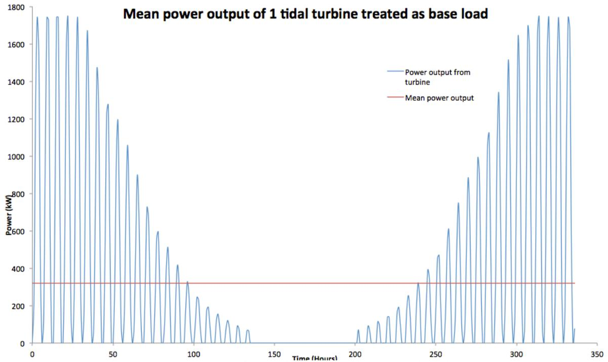
Figure 33 – Mean output from 1 tidal turbine if treated as base load
