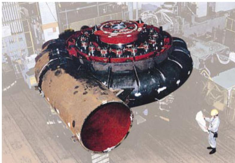
Figure 6 – Appearance of pump turbine during shop assembly [13]
