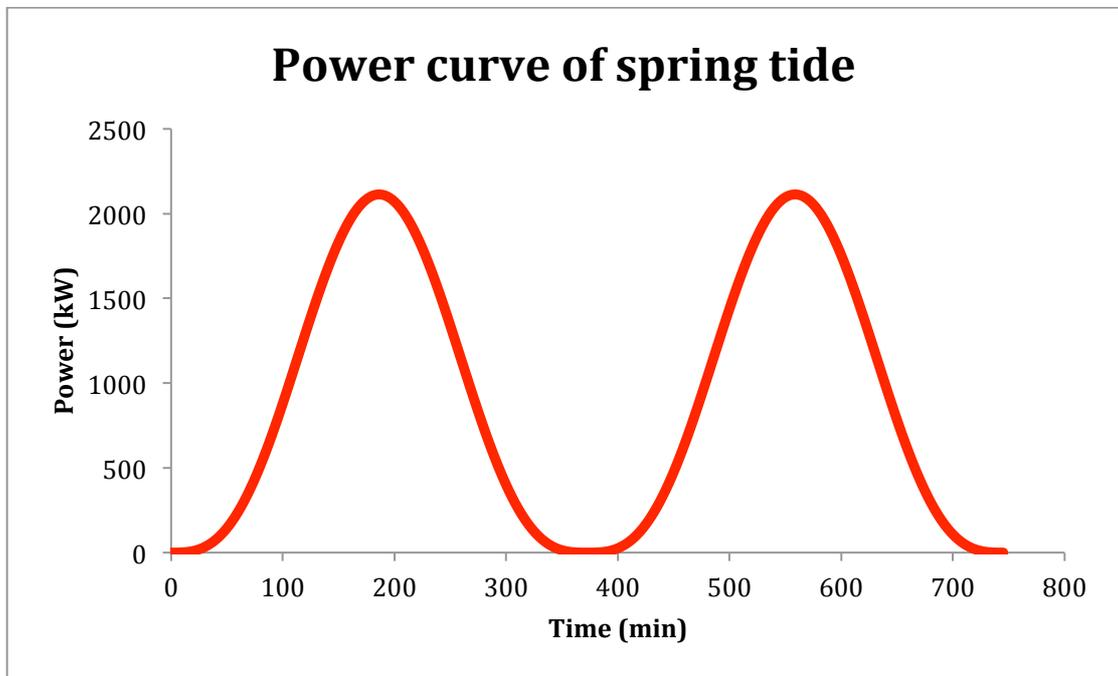
Figure 30 – Power curve of spring tide
