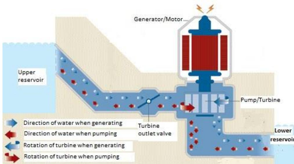
Figure 2 – Schematic of water flow through the pump turbine [6]
