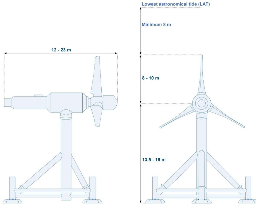
Figure 26 – Tidal stream turbine schematic [26]
