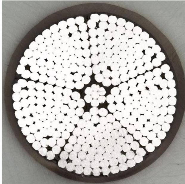
*Figure 3-2 Miliken Conductor cross section (associates)*
