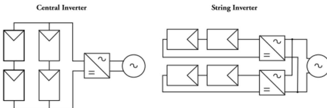
Figure 2-7 Inverter configurations (Alasdair Miller, 2010)
