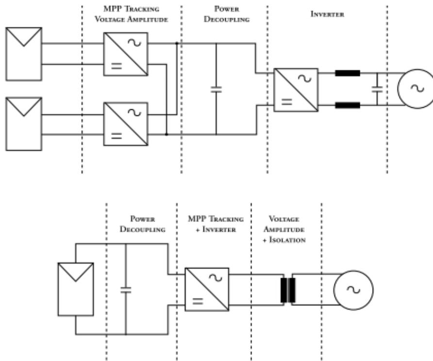
Figure 2-8 Transformer and transformerless inverter configuration (Alasdair Miller, 2010)
