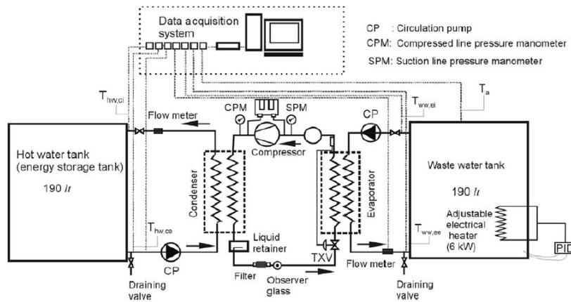
Figure 21: Heat Pump Hot Water System Set up (Kahraman, 2009)
