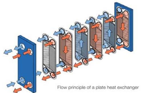
Figure 12: Flat Plate Heat Exchanger (Energy Today , 2012)
