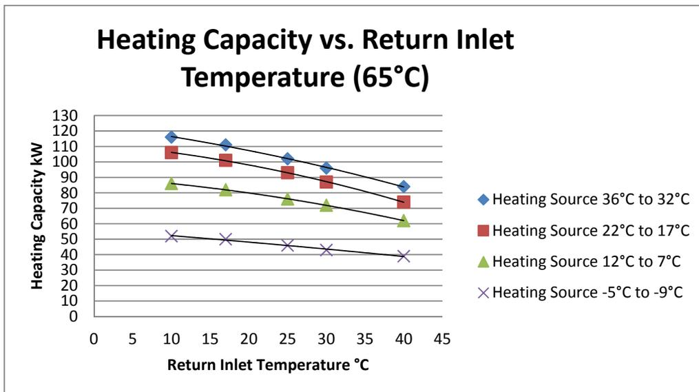
Figure 53: Heating Capacity vs. Return Inlet Temperature (65°C)
