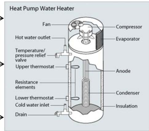
Figure 19: HPWH Tank (Energy, 2012)
