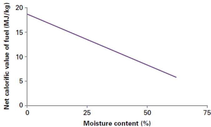
Figure 68: Moisture Content vs. NCV
