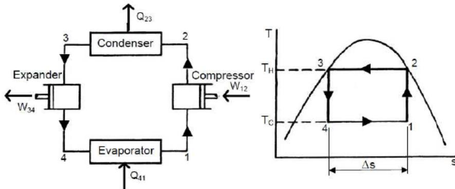
Figure 6: Carnot Vapour Refrigeration Cycle (Tuohy, 2013)
