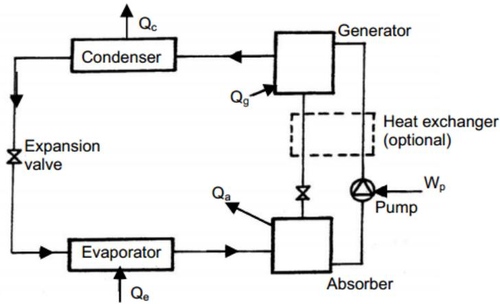
Figure 8: The Absorption Cycle (Tuohy, 2013)
