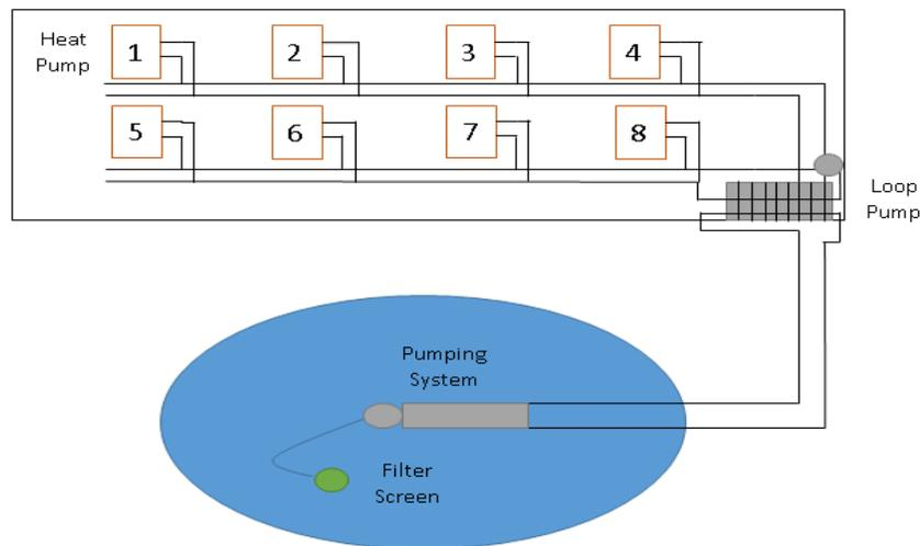
Figure 16: Surface Water Heat Pumps - Open Loop
