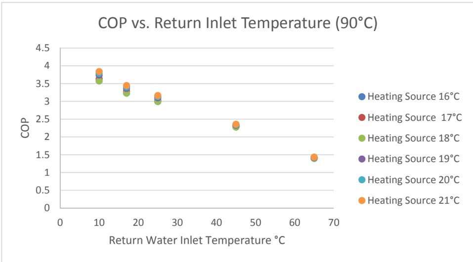
Figure 63: COP vs. Return Inlet Temperature (90°C)
