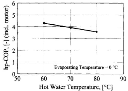
Figure 30: COP vs. Varying Hot Water Temperature
