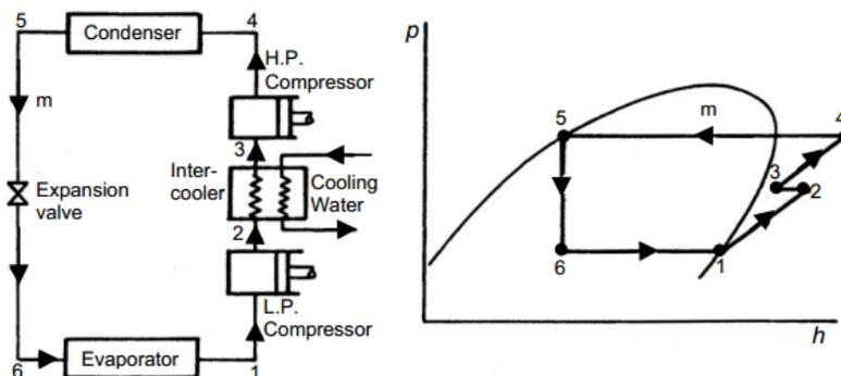
Figure 9: Multi-stage Heat Pump (Compound)
