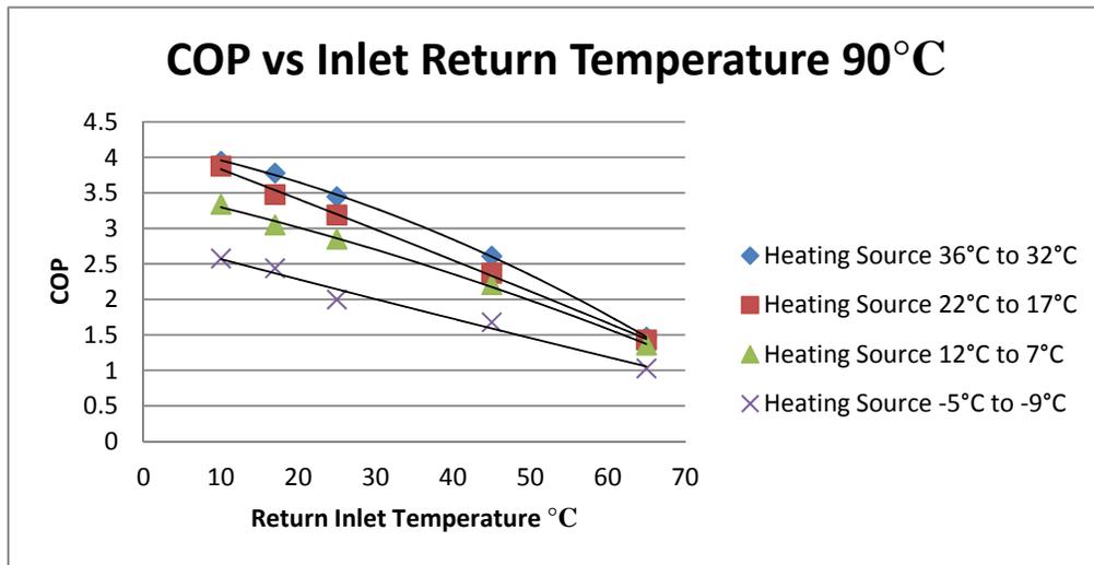
Figure 60: COP vs Return Inlet Water Temperature (90°C)
