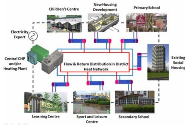
Figure 39: District Heating Network (Energy Saving Trust, 2013)
