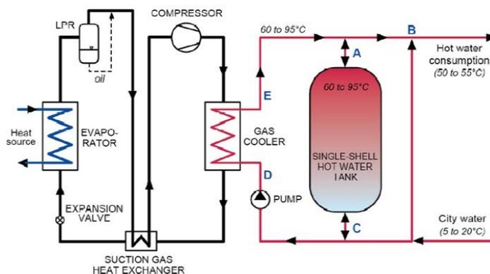
Figure 28: Simple Heat Pump Water Heater with Single Tank (Hjerkin, 2007)
