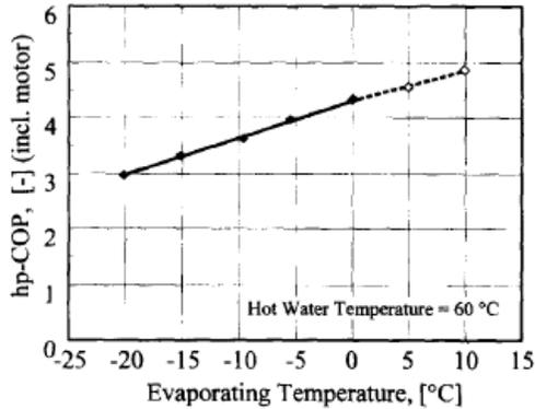
Figure 31: COP vs. Varying Evaporator Temperature
