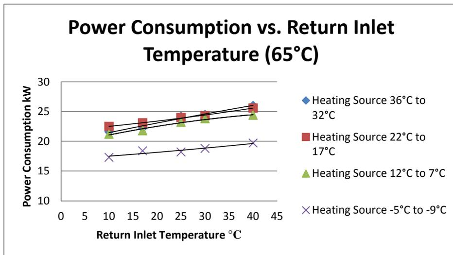
Figure 57: Power Consumption vs. Return Inlet Temperature (65°C)
