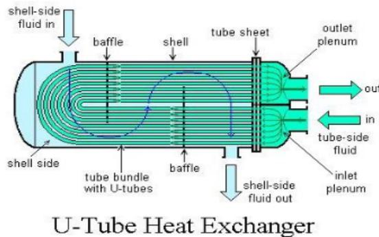
Figure 11: U-Tube Shell and Tube Exchanger (Bengston, 2010)
