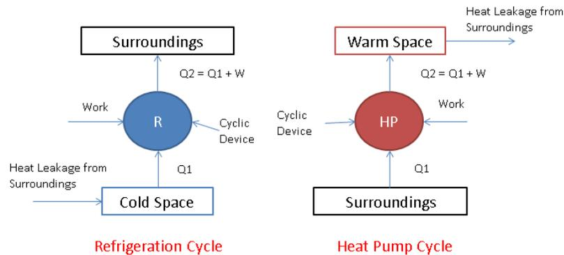
Figure 5: Refrigeration vs. Heat pump cycles
