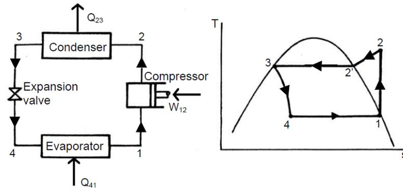
Figure 7: Vapour Compression Refrigeration System (Tuohy, 2013)
