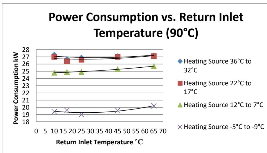
Figure 58: Power Consumption vs. Return Inlet Temperature (90°C)
