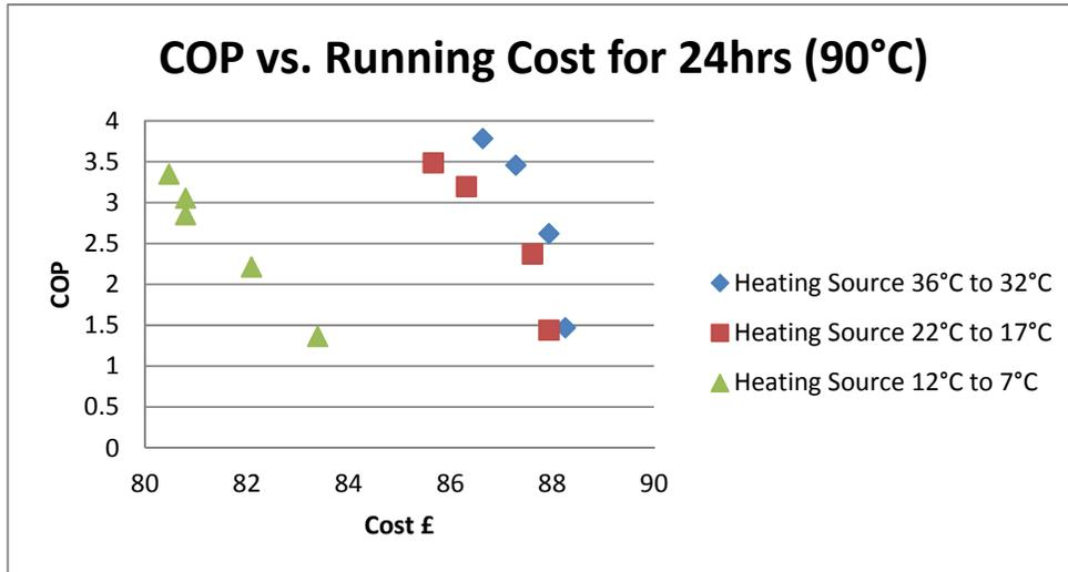
Figure 62: COP vs. Running Cost for 24hrs (90°C)
