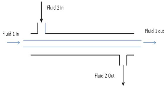
Figure 10: Double pipe Heat Exchanger
