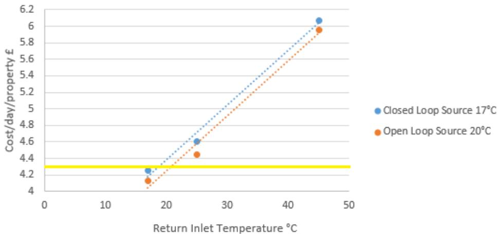
Figure 67: Cost/Day per Property vs. Return Inlet Temperature
