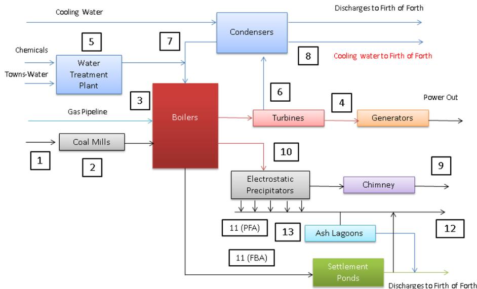
Figure 2: Diagram showing Longannet System
