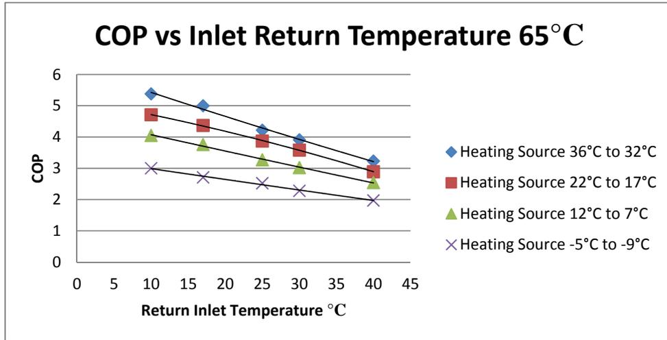
Figure 59: COP vs Return Inlet Water Temperature (65°C)
