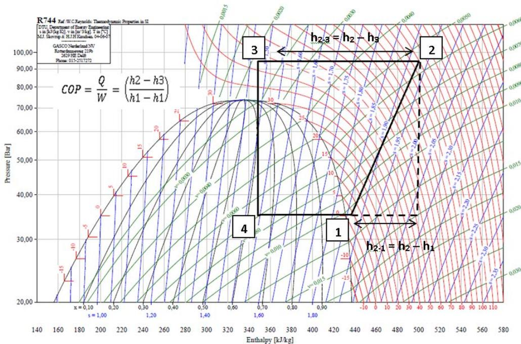
Figure 32: P-h Chart for simple CO<sup>2</sup> Transcritical cycle (DTU, 2007)
