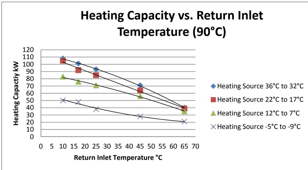
Figure 54: Heating Capacity vs. Return Inlet Temperature (90°C)
