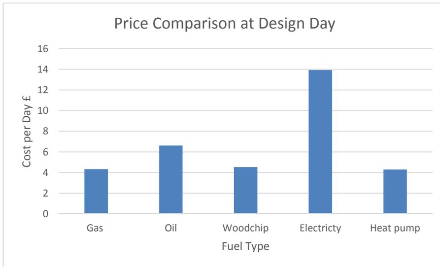
Figure 66: Price Comparison for Different Fuel Types
