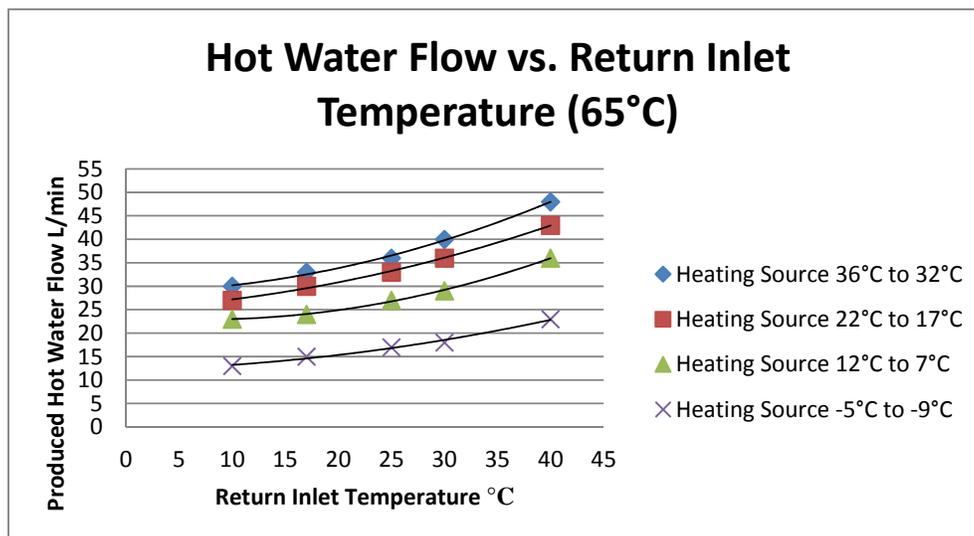
Figure 56: Hot Water Flow vs. Return Inlet Temperature (65°C)
