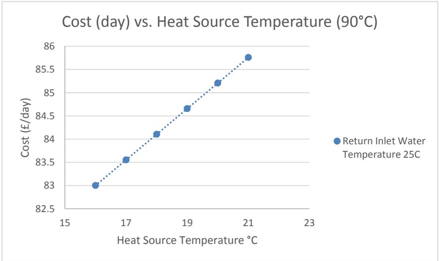
Figure 64: Cost per Day vs. Heat Source Temperature (90°C)
