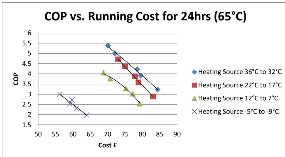
Figure 61: COP vs. Running Cost for 24hrs (65°C)
