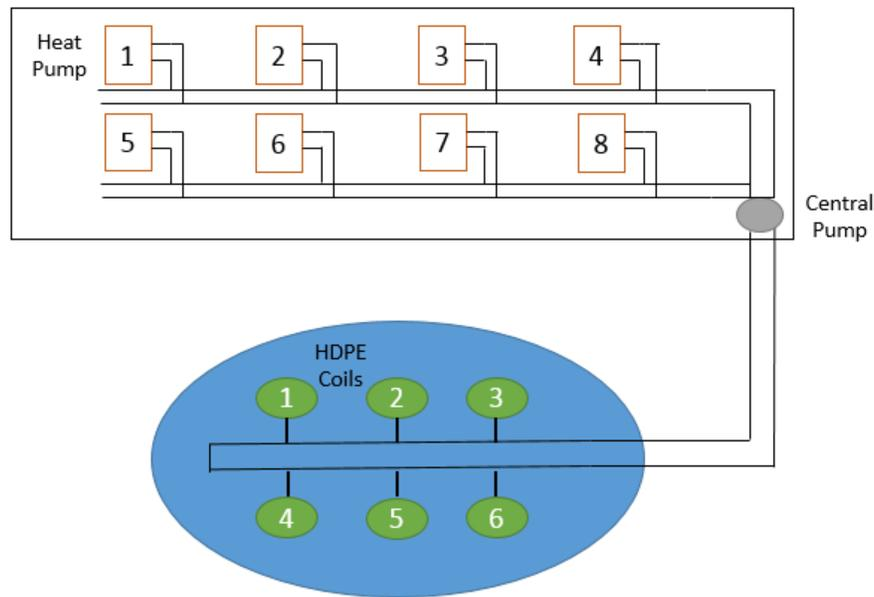
Figure 13: Closed Loop Surface Water System
