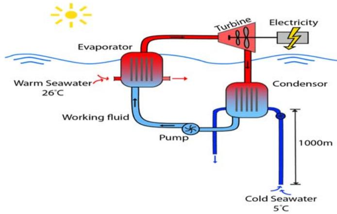
Figure 17: Closed loop OTEC Technology (Delft University of Technology , 2014)
