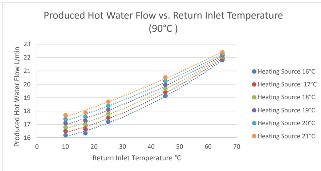
Figure 65: Produced Hot Water Flow vs. Return Inlet Temperature (90°C)
