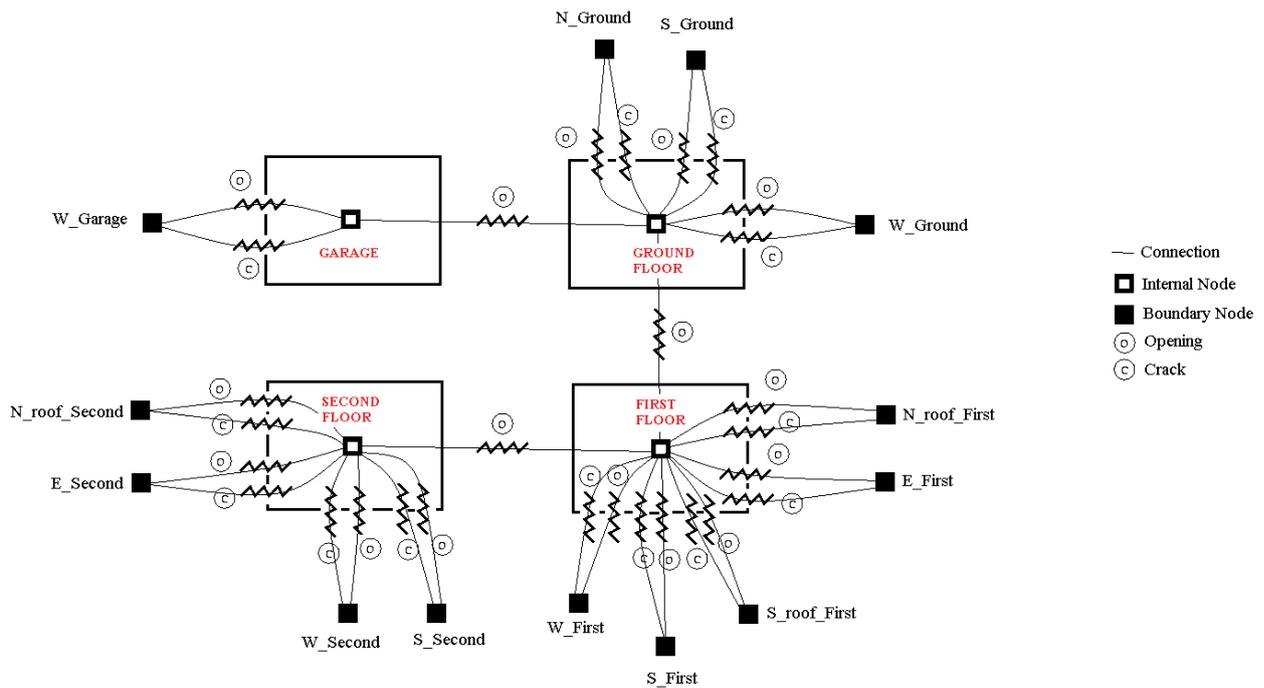
Figure 20. Air flow network for the low energy house in Cornwall
