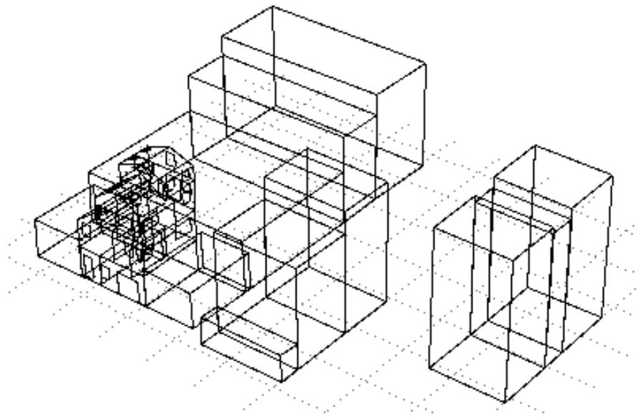
Figure 12. Model of the house including the shading from other houses and the valley
