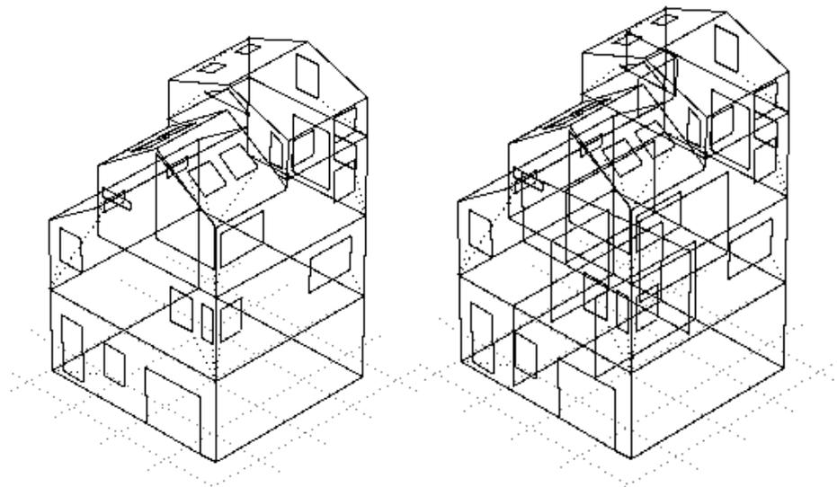
Figure 11. Base model without internal walls (left) and with them (right)
