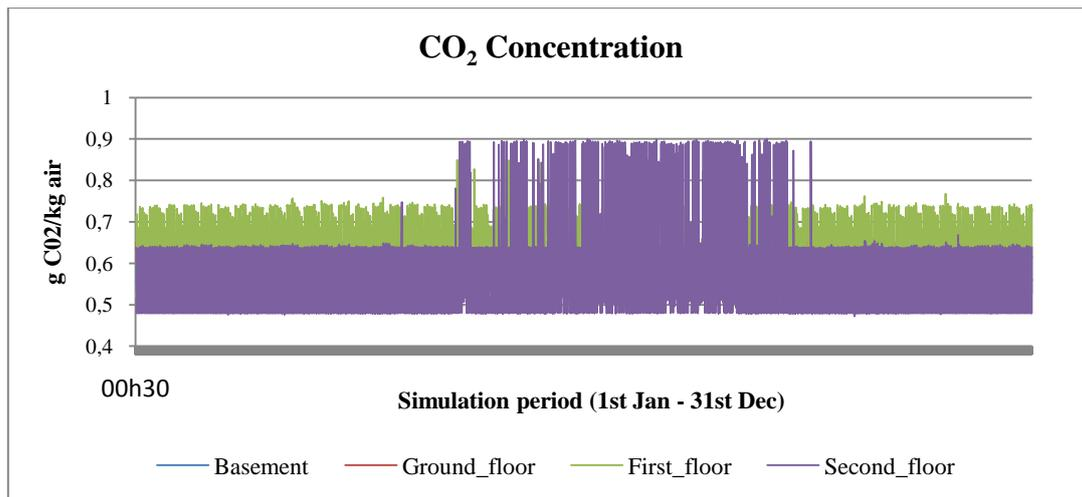
Figure 26. CO<sub>2</sub> concentration inside zones for Mechanical Ventilation
