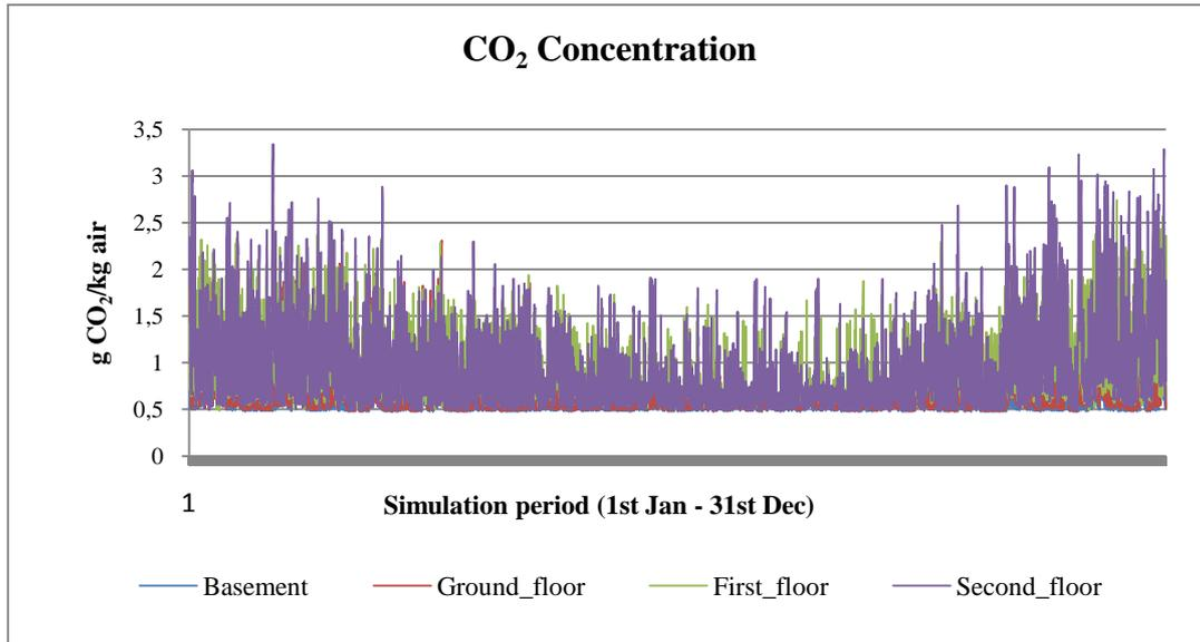
Figure 25. CO<sub>2</sub> concentration inside zones for Natural Ventilation
