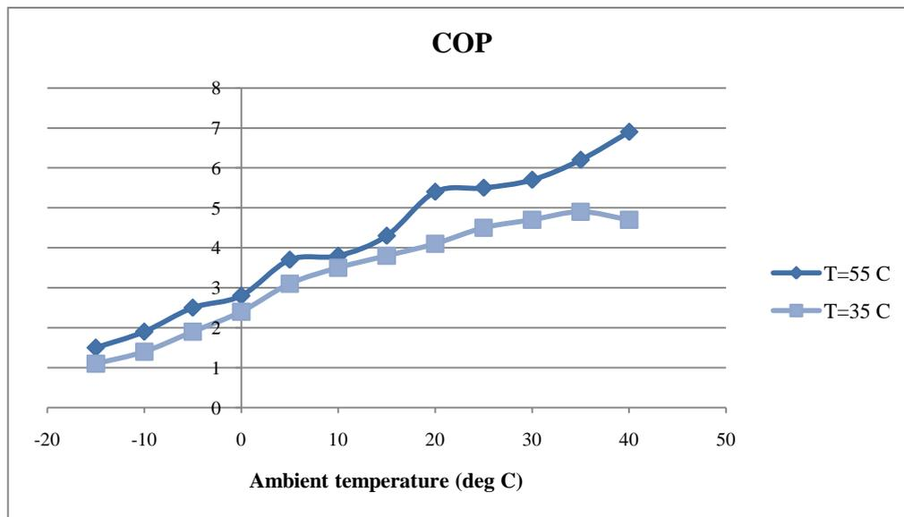
Figure 24. COP Curve for the ASHP STÜHMR AXHW-05
