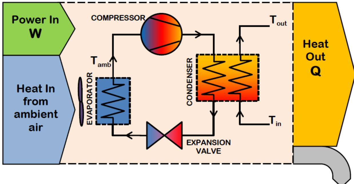
*Fig: 2.1.4 Heat pump vapour compression cycle*
