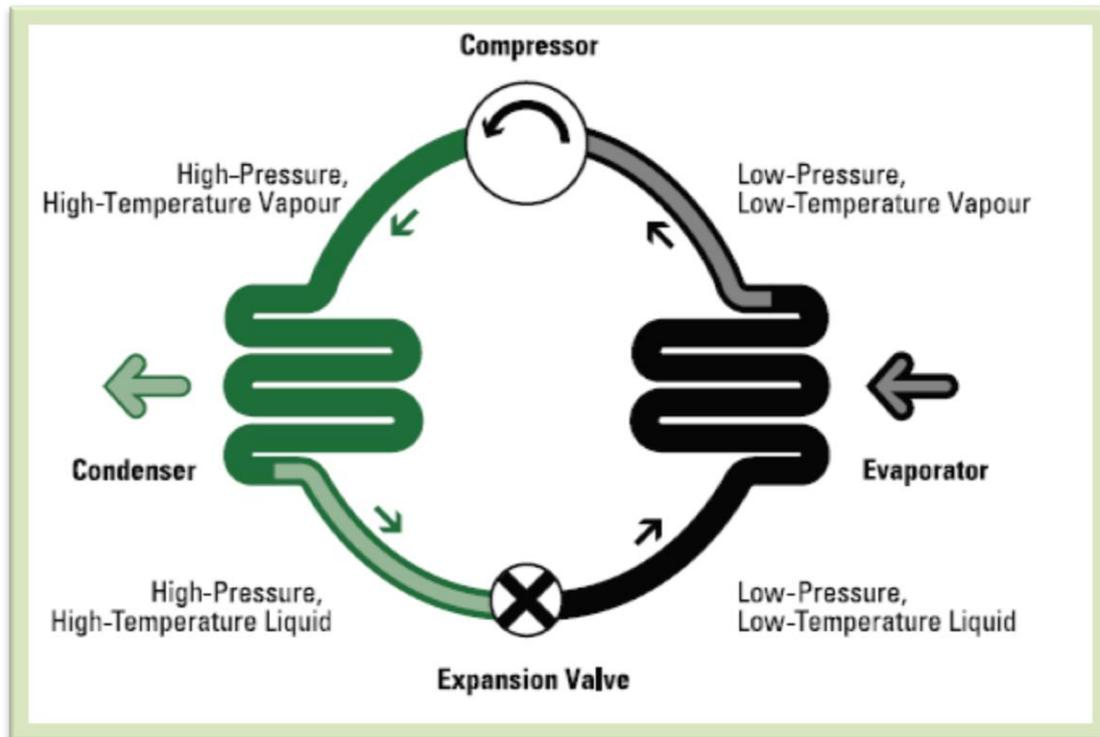
*Fig: 2.1.3 Basic heat pump cycle*
