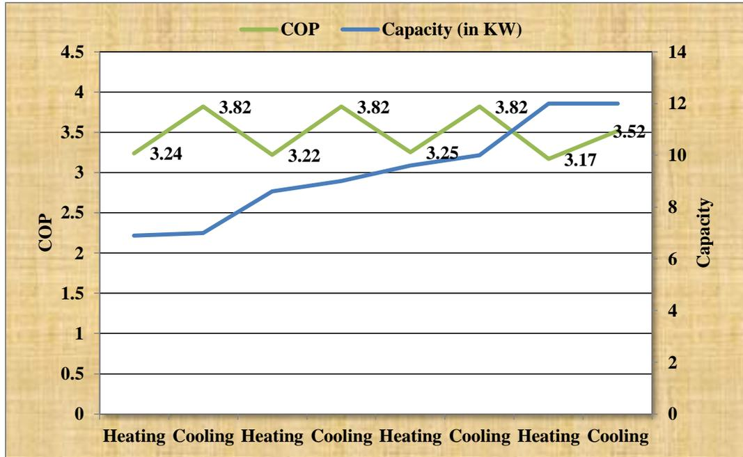
**Fig 4.2: GSHP Heating & cooling Capacity against its COP in cold region**
