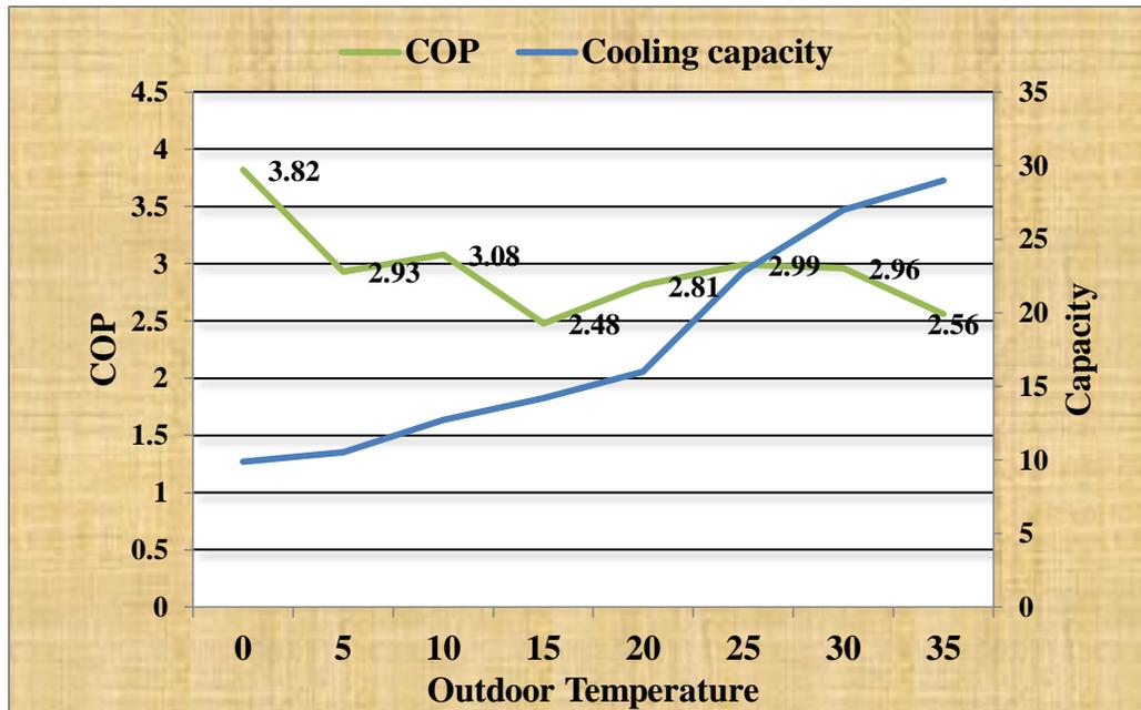
Similar analysis is carried out with the help of RETScreen for Ground source heat pumps. Using the database for Ground source heat pump, different models, their heating and cooling capacities are matched with the corresponding heating & cooling COP's to find out the efficiency of GSHP in both the climates.
