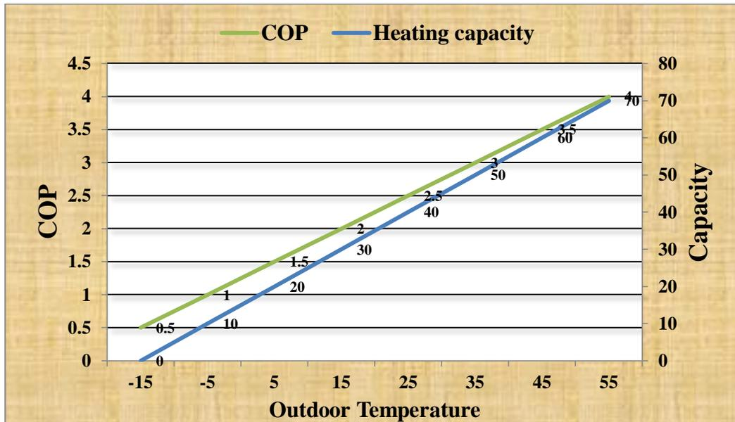
Also the cooling capacities and COP for each of the models used above were noted. Heating capacity is of more importance in this case, due to the behavior and performance of the system in the house located in a cold region.
