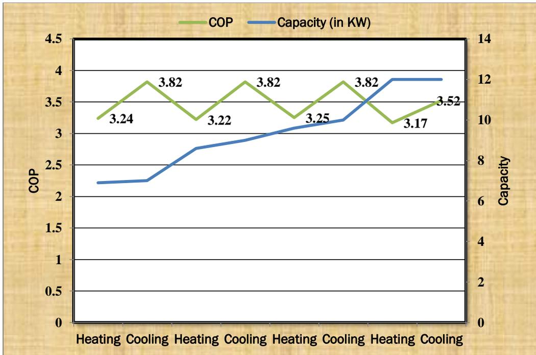
**Fig 4.1: ASHP Heating & cooling Capacity against its COP in cold region**
