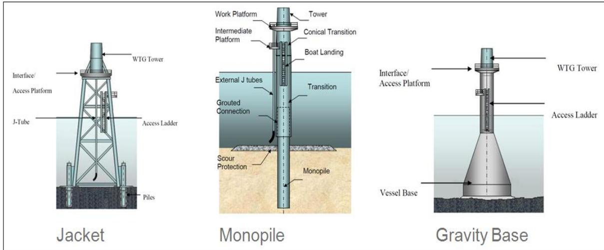
**Figure 7:** Base foundations used in this investigation (adapted from IMECHE, 2010)
