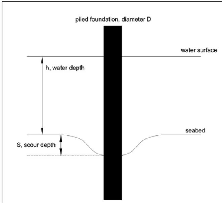
**Figure 17:** Scour cross section (Whitehouse et al., 2007)
