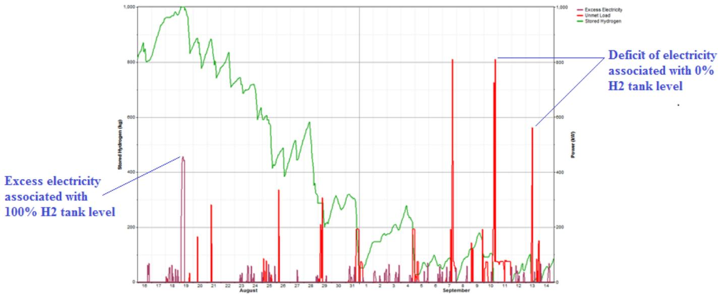
Graph 9. Evolution of power deviations incurred by a Wind-H<sub>2</sub> system and the H<sub>2</sub> storage (16 August-14 September)
