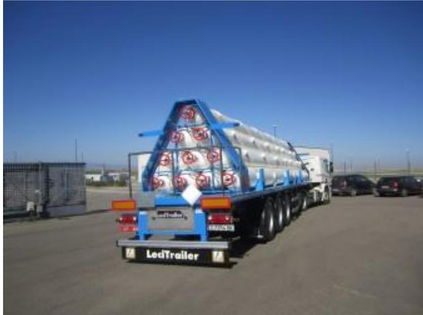
Figure 19. Compressed hydrogen transportation (Calvera, n.d.)
