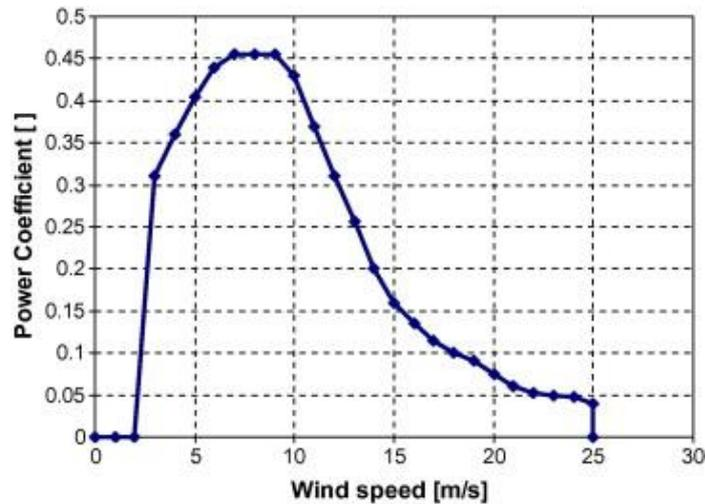
Table 2:  $C_p$  vs wind speed (Basbous, et al., 2012)
