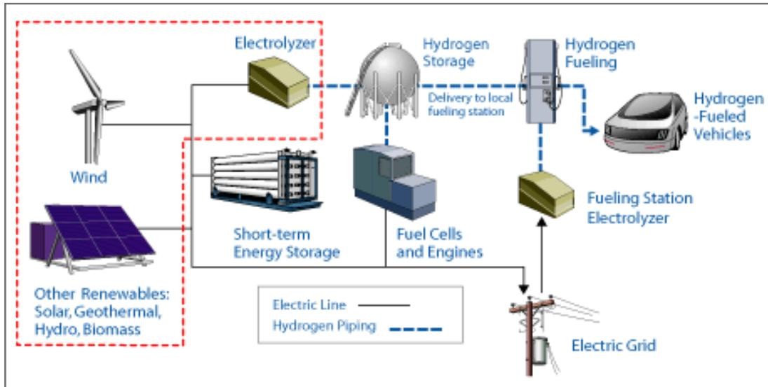
Figure 7: Configuration of a Wind-H<sub>2</sub> energy system (Www1.eere.energy.gov, 2011)
