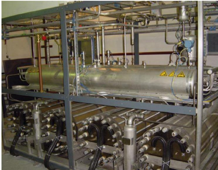
Figure 15. Alkaline electrolyser installed in the experimental Wind-H<sub>2</sub> farm "Sotavento" (Rey, 2008)
