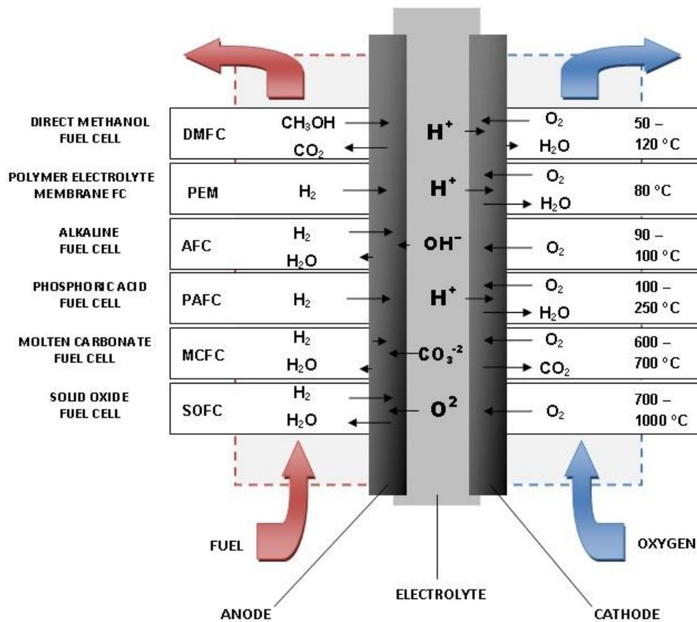
Figure 6. Operating principle of the different types of fuel cell (Fuelcells.org, 2013)
