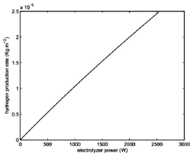
Figure 5: Relation between hydrogen production and power consumption of the electrolyser (Mengfbar, 2011)
