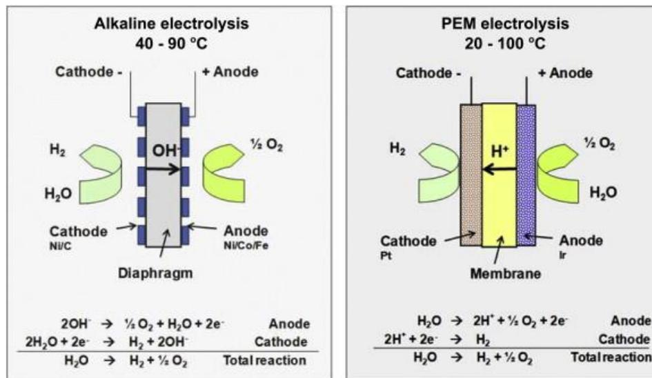
Figure 4. Schematic of the operating principle of an alkaline and PEM water electrolysis cell (Carmo, M; Fritz, D; Mergel, J et al.; 2013)
