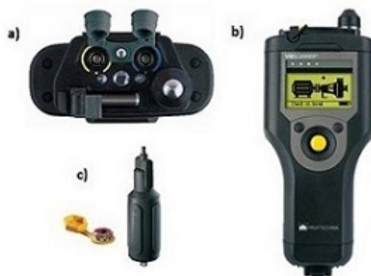
**Figure 3.10:** Example vibration measuring instrument (VIBSCANNER), a) built sensor on the top of the data collector, b) data collector, c) transducer with coded measurement location [18].
