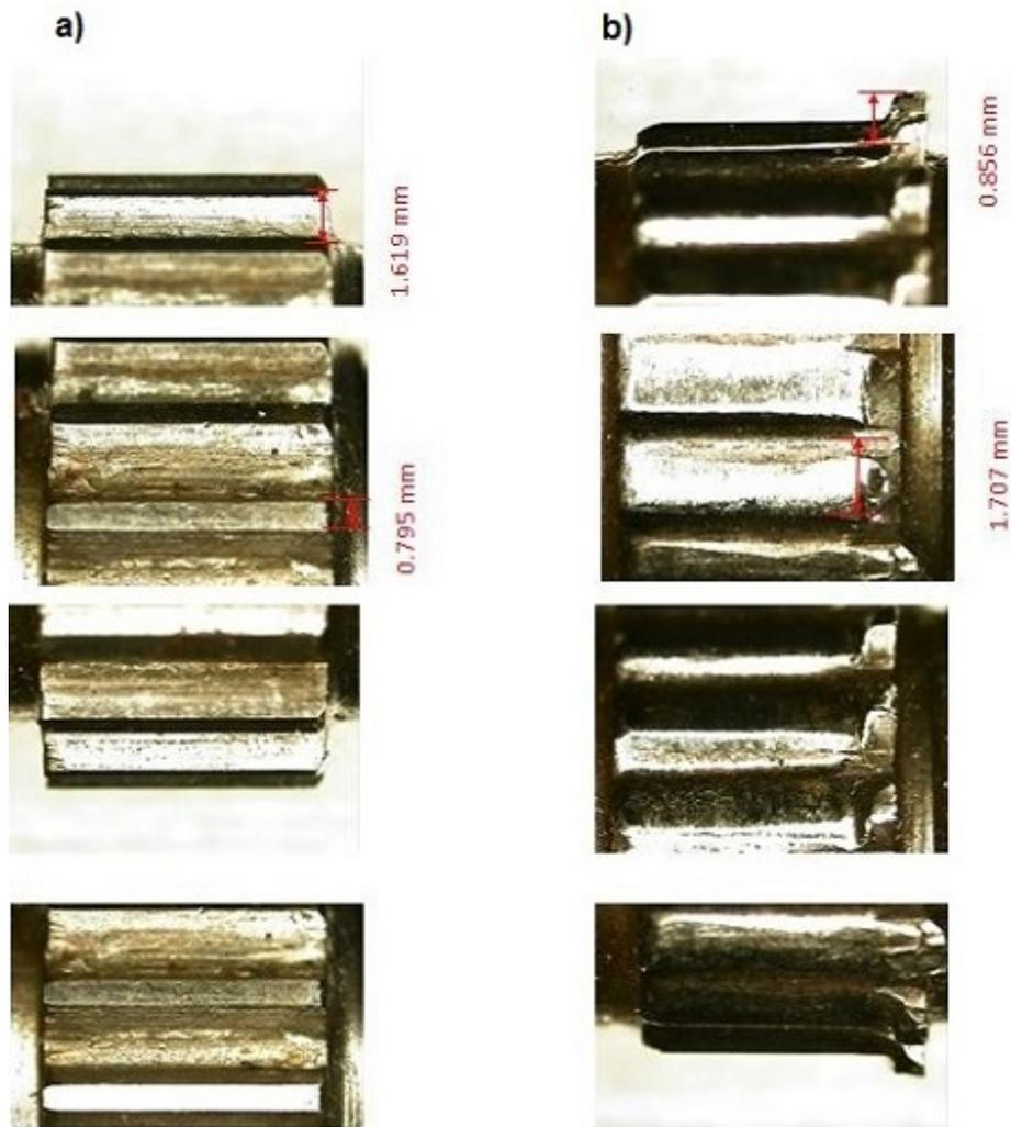
**Figure 5.3:** Optical analysis of motorcycle main shaft, a) 2,000 mile b) 10,000 mile.
