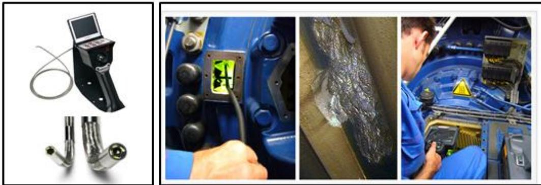
**Figure 3.16:** Example of a videoscope instrument for visual inspection of wind turbines components, as well a technician inspecting the gearbox interior [68, 69].
