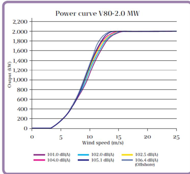
**Figure 10: Power curve at different sound levels for the V-80 2MW wind turbine (VESTAS, 2012)**
