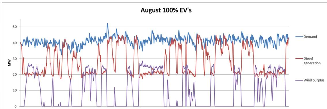
**Figure 28: Total electricity demand profile, electricity demand covered by diesel generation and wind surplus in Island H for the August month with a 0 and 100% *EV* penetration (own elaboration)**
