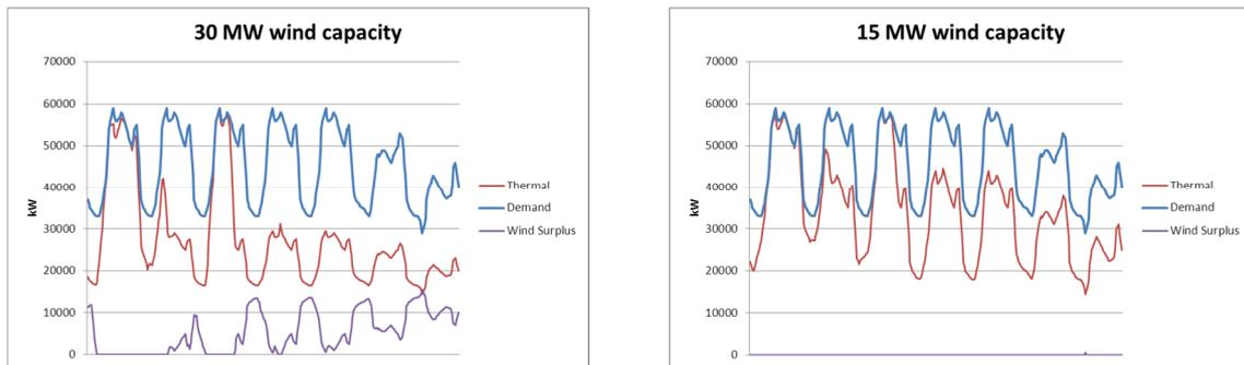
**Figure 13: Effect of different wind capacities in an electrical system with a 50% wind power penetration limit**
