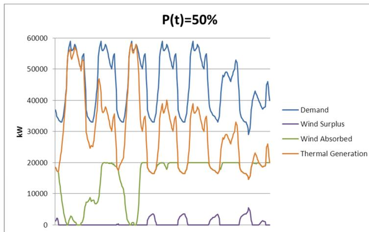
**Figure 12: Continuation of the example graph showing the calculation of the thermal generation required (own elaboration)**
