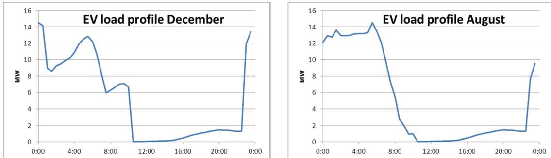
**Figure 23: Resulting *EV* charging load for the two months analyzed for a 100% *EV* penetration (own elaboration)**
