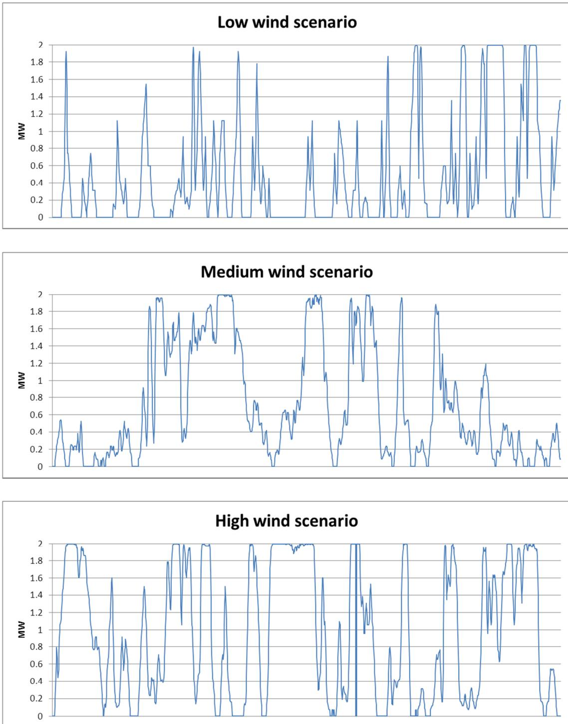
**Figure 24: Wind power generation of a V80-2MW turbine during a month in the three possible scenarios analysed. (own elaboration)**
