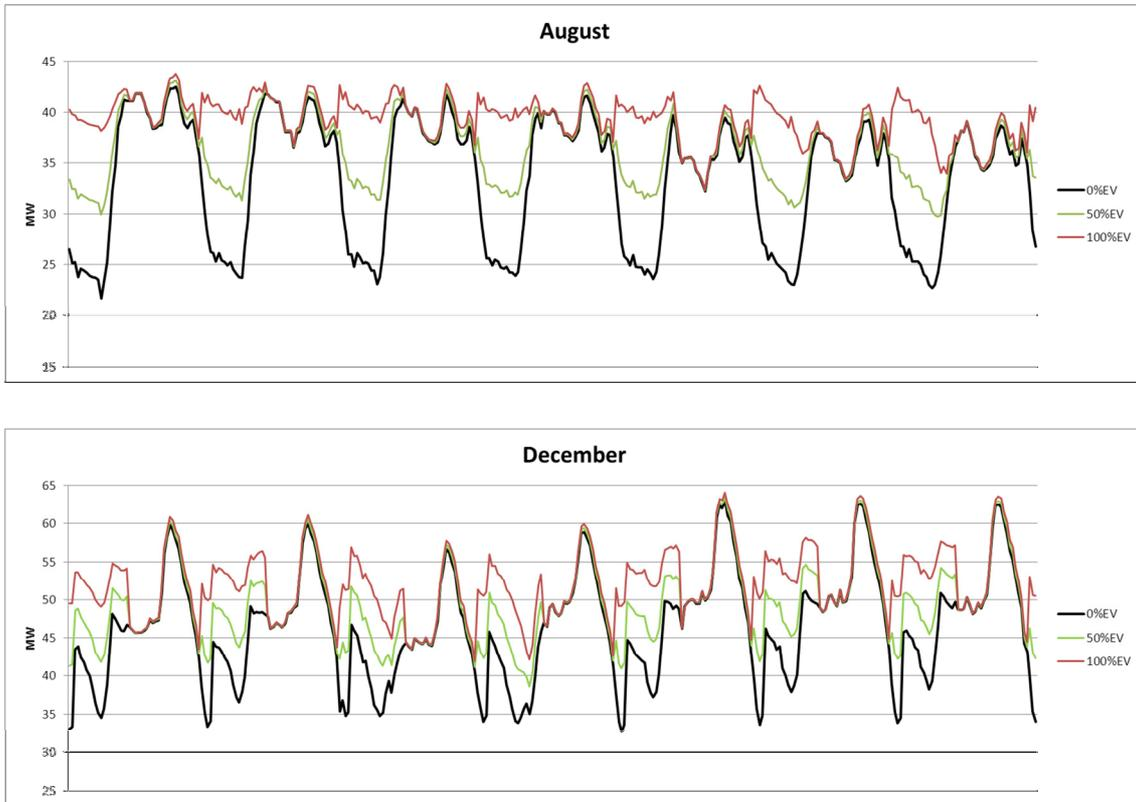
**Figure 25: Electricity demand profile for a sample week in the two different months analyzed for 0%, 50% and 100% *EV* penetration levels.(own elaboration)**
