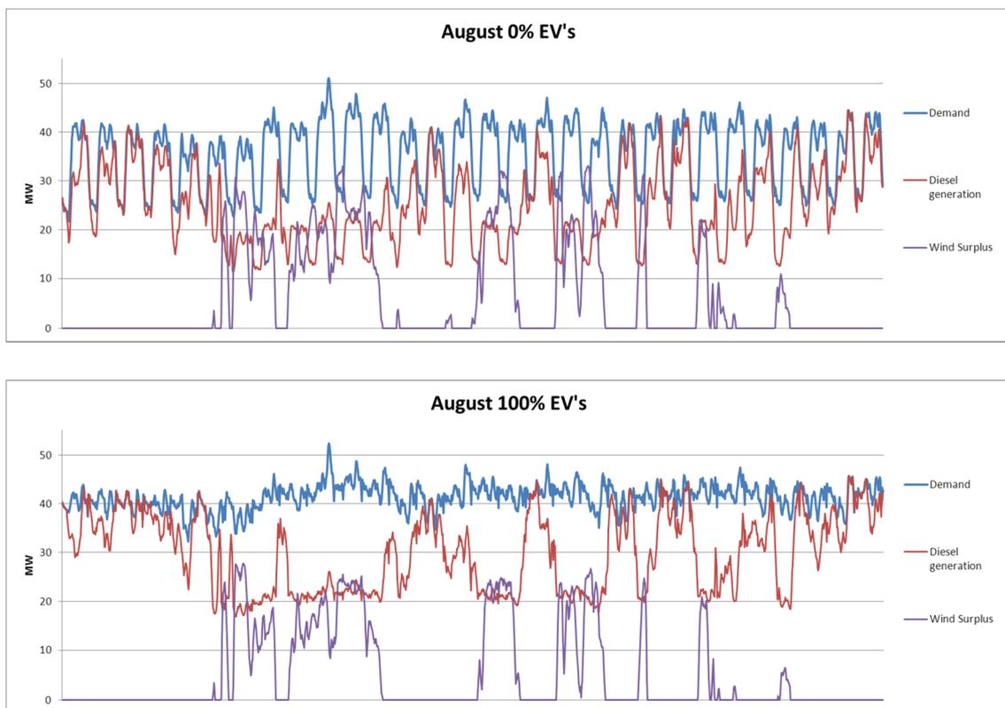
**Figure 27: Total electricity demand profile, electricity demand covered by diesel generation and wind surplus in Island M for the August month with a 0 and 100% *EV* penetration. (own elaboration)**
