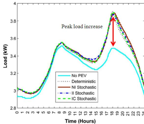
**Figure 16: Average load profile per person with 100% EV penetration with different estimation methods (Ashtari et al, 2012)**
