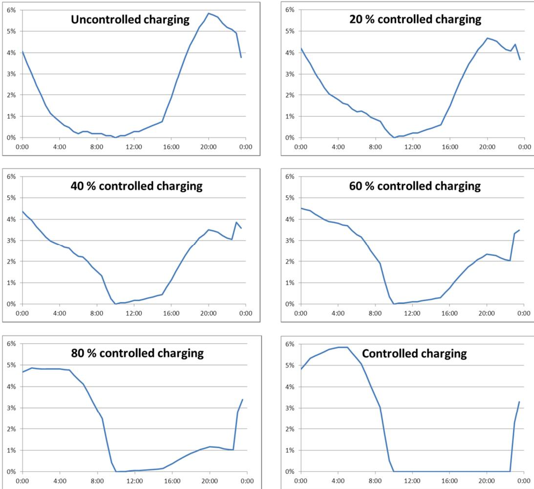
**Figure 20: Distribution of the EVs charging load depending on the percentage of EVs following the controlled charging (CC) (own elaboration).**
