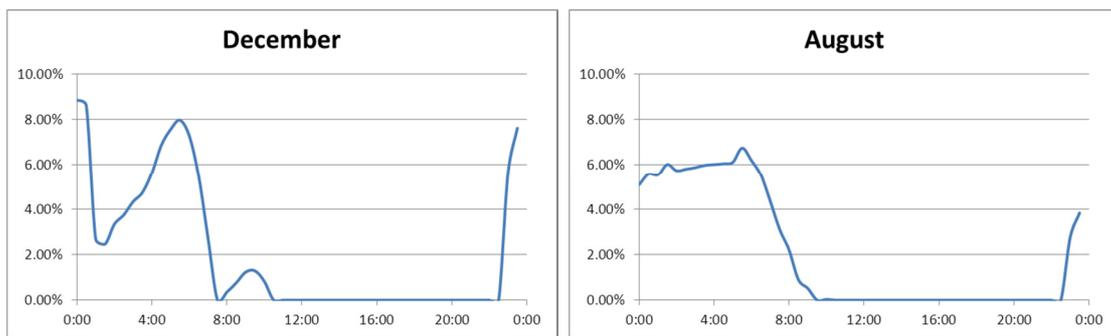
**Figure 22: Controlled *EV* charging load distribution (%<sub>c</sub>) for December and August**
