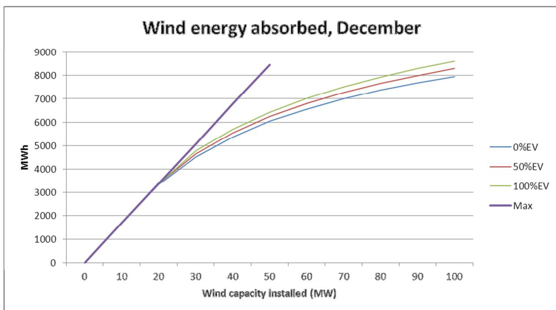
**Figure 29: Total wind energy absorbed in relation to the wind power capacity installed for different *EV* penetration levels. December month in Island L. (own elaboration)**
