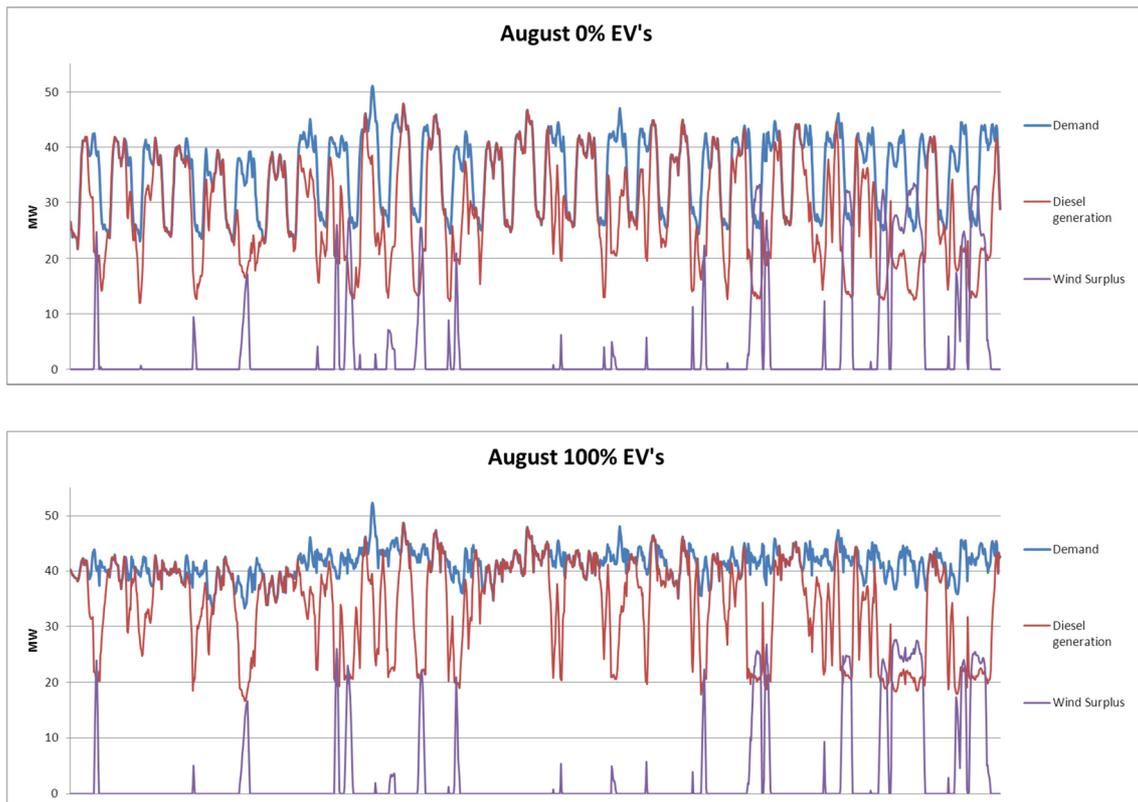
**Figure 26: Total electricity demand profile, electricity demand covered by diesel generation and wind surplus in Island L for the August month with a 0 and 100% EV penetration. (own elaboration)**
