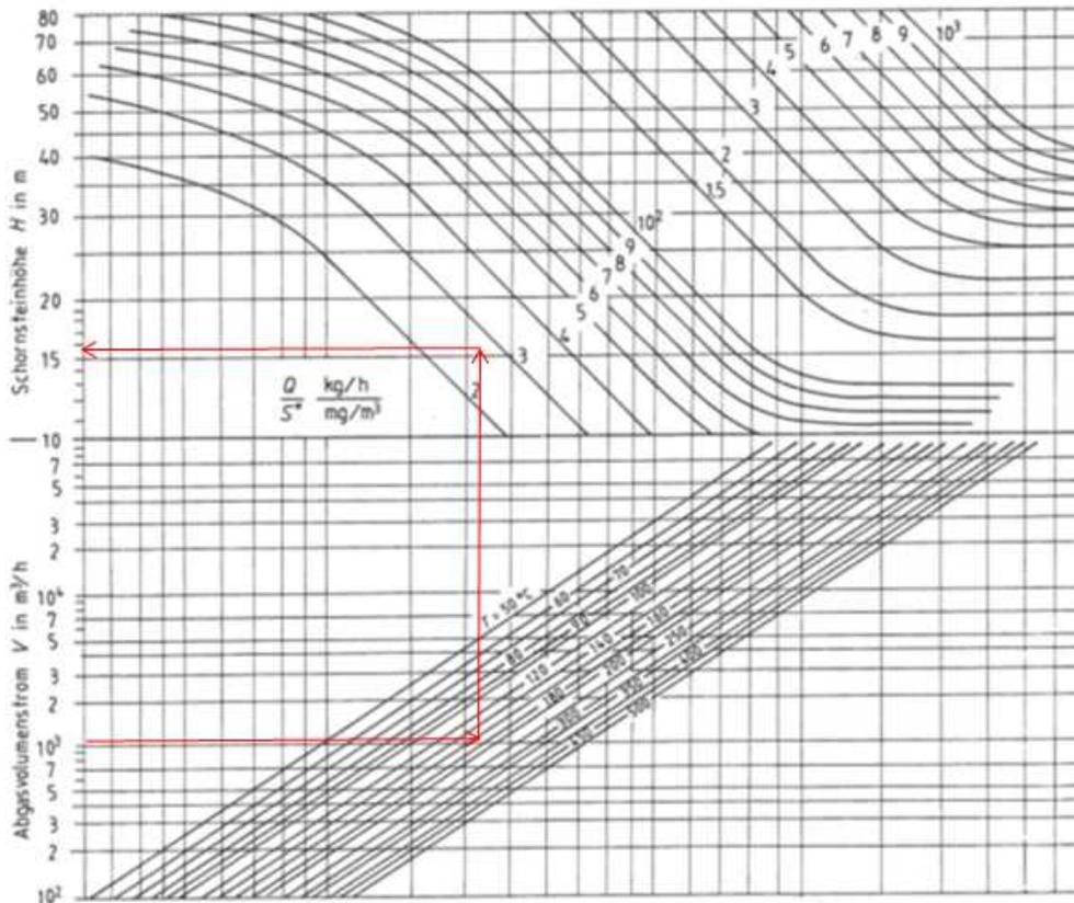
Figure 26: Diagram for chimney height calculation included in the Austrian regulation ÖNORM
