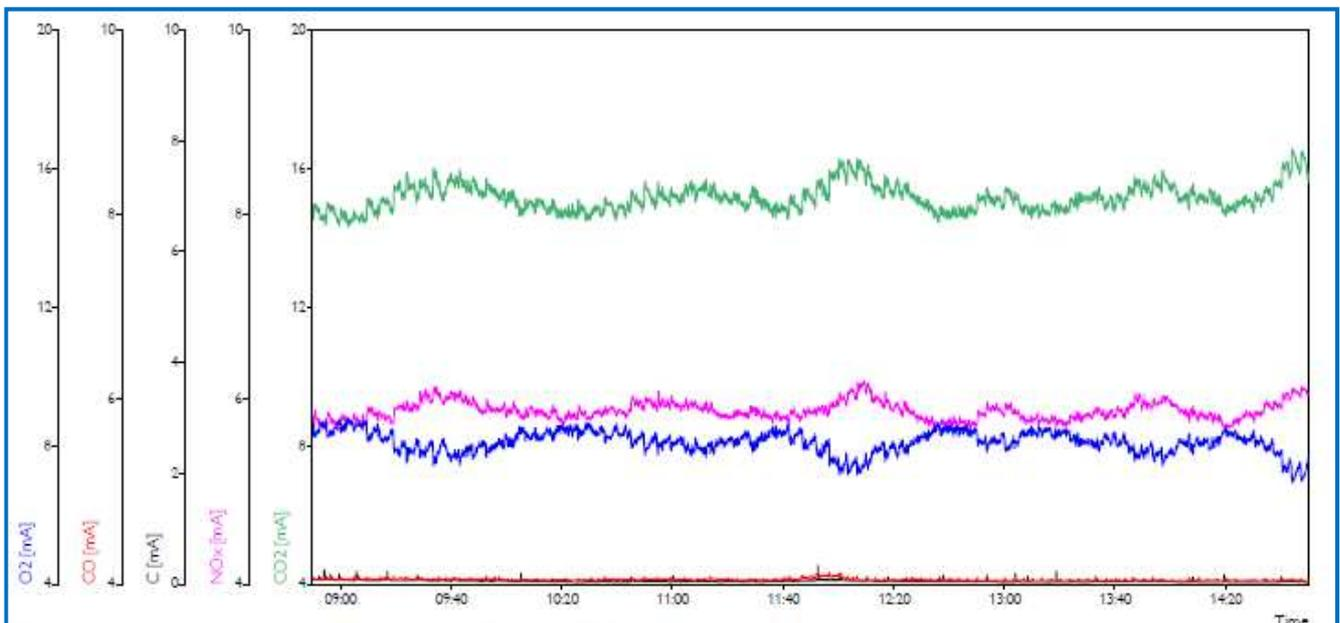
**Figure 16: Concentration of air pollutants versus time at nominal heat output. SOURCE: [Ref. 32]**
