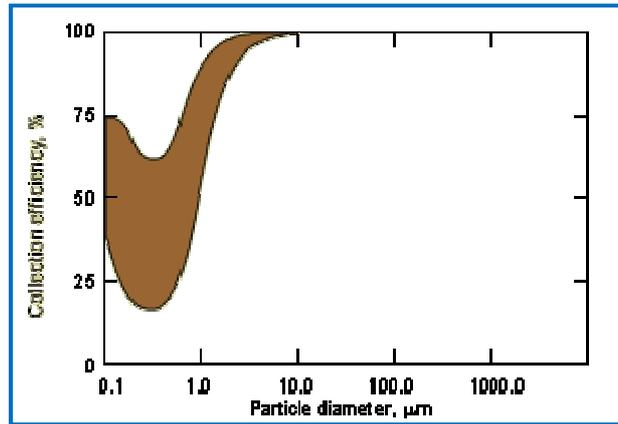
Figure 6: Particle size-Efficiency of wet scrubbers. SOURCE: US EPA [Ref.59].
