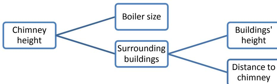
Figure 36: Diagram showing the relationship of the parameters influencing chimney height for the Swedish calculation procedure.
