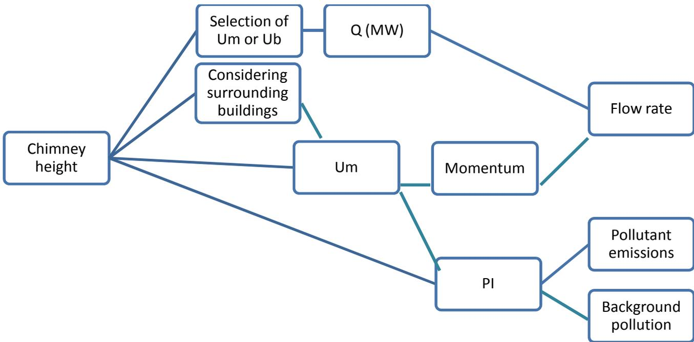
**Figure 32: Diagram showing the relationship of the parameters influencing chimney height for the UK calculation procedure.**
