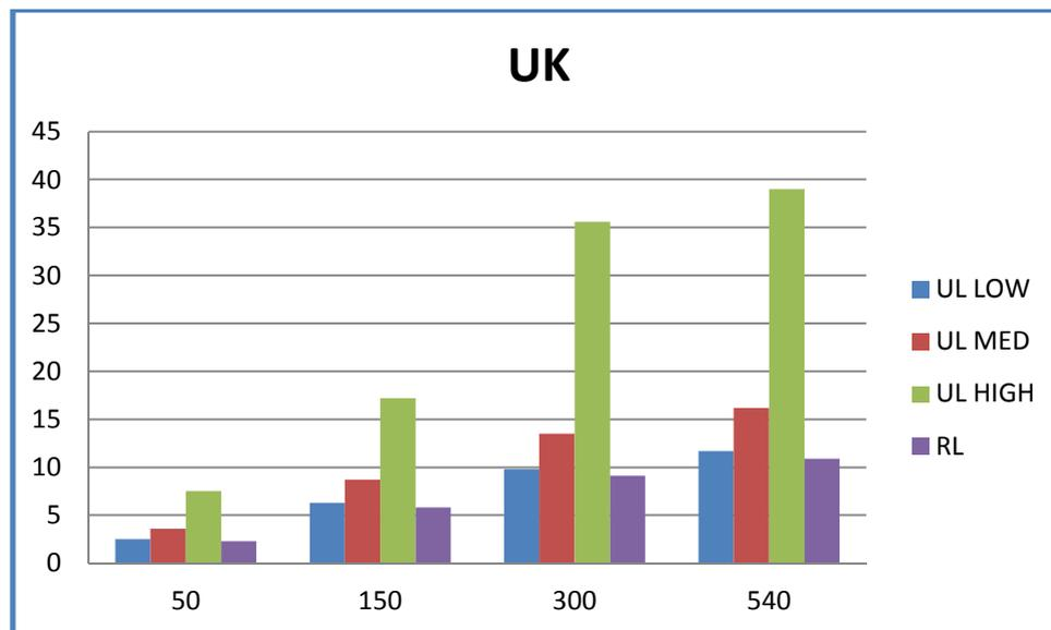
Figure 31: Chimney height calculation results for the created case studies following the UK methodology.
