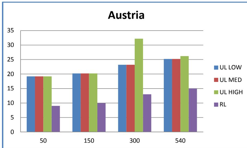
**Figure 37: Chimney height calculation results for the created case studies following the Austrian methodology.**
