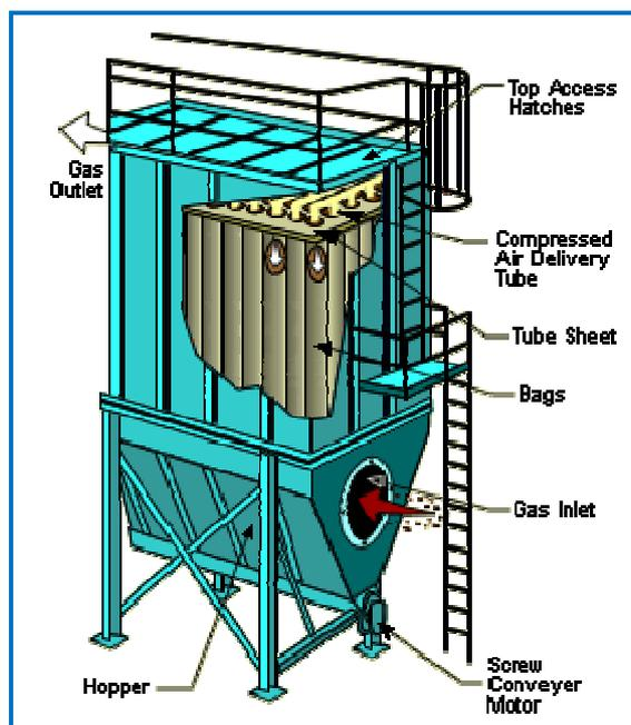
Figure 9: Pulse jet fabric filter. SOURCE: US EPA [Ref.59].
