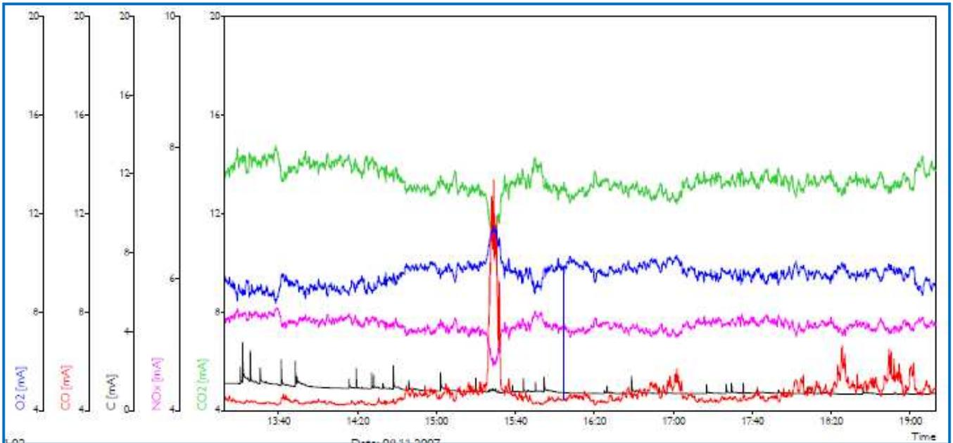
Figure 17: Concentration of air pollutants versus time at minimum heat output. *SOURCE: [Ref. 32]*
