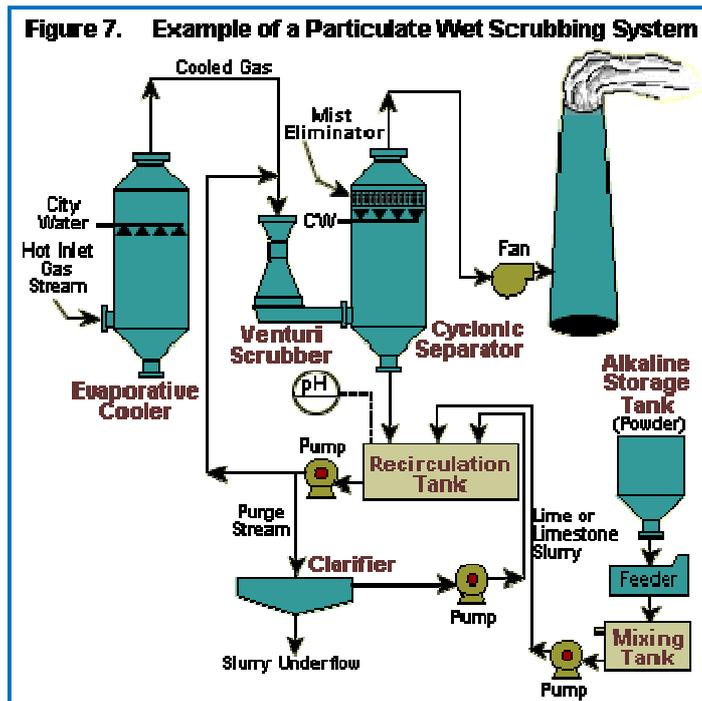
Figure A1: Example of a PM Wet Scrubbing system. SOURCE: US EPA
