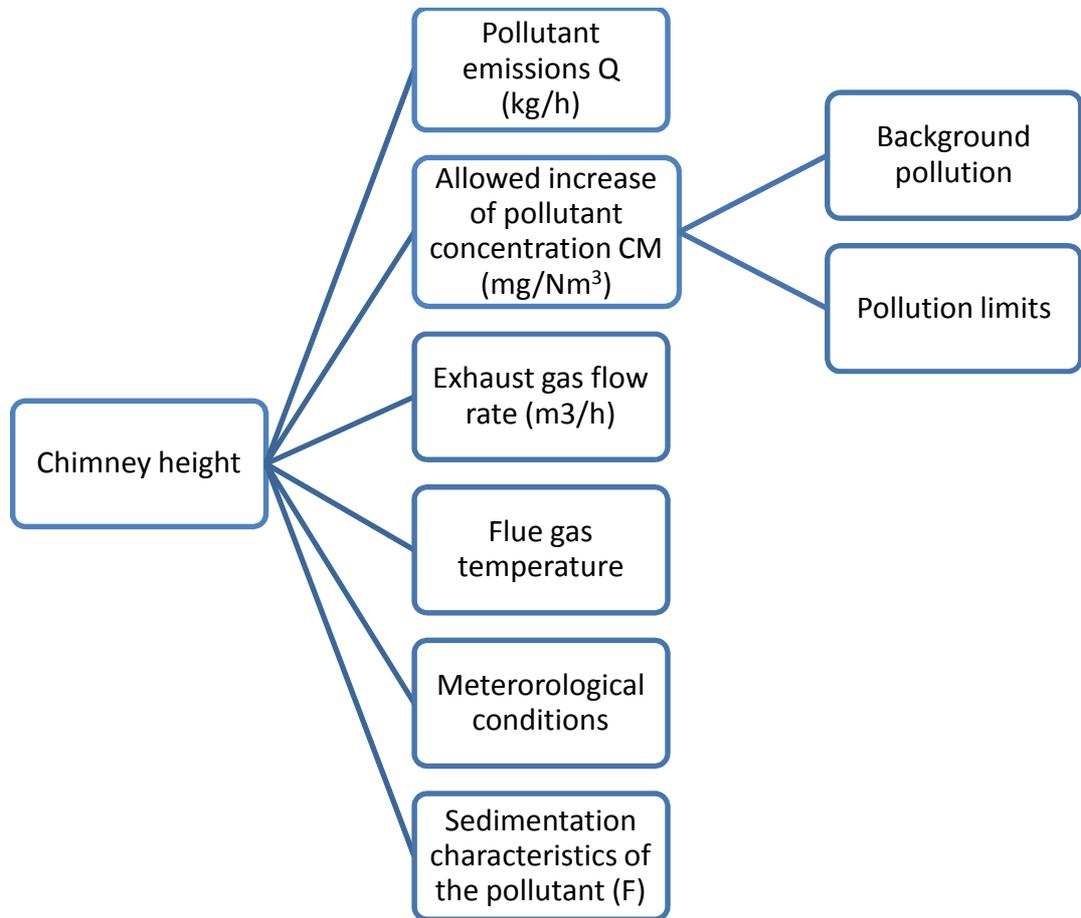
**Figure 34: Diagram showing the relationship of the parameters influencing chimney height for the Spanish calculation procedure.**
