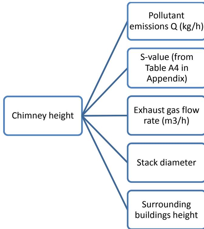
Figure 41: Diagram showing the relationship of the parameters influencing chimney height for the German calculation procedure (P&K software)
