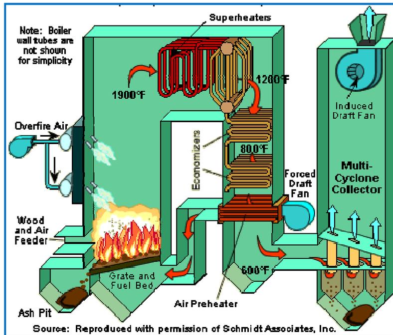
Figure 2: Multi-cyclone collector in a small wood fired boiler. SOURCE: US EPA [Ref.59]
