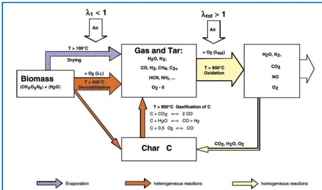
Figure 1: Main reactions during a two-stage biomass combustion process. SOURCE: [Ref.44]
