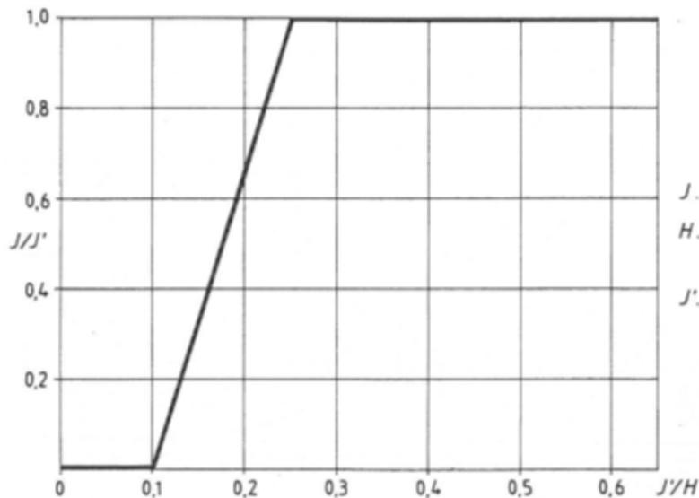
Figure 27: Diagram to include building influence in the Austrian calculation method
