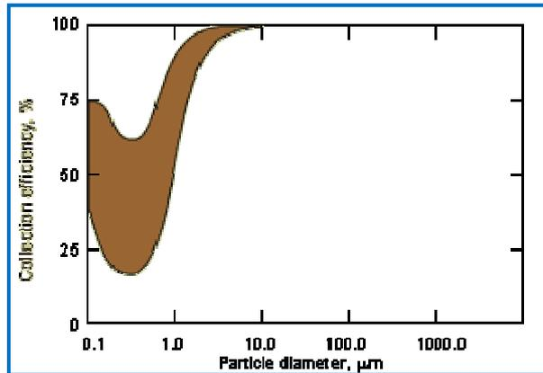
Figure 8: Particle size-Efficiency of electrostatic precipitators. SOURCE: US EPA [Ref.59].
