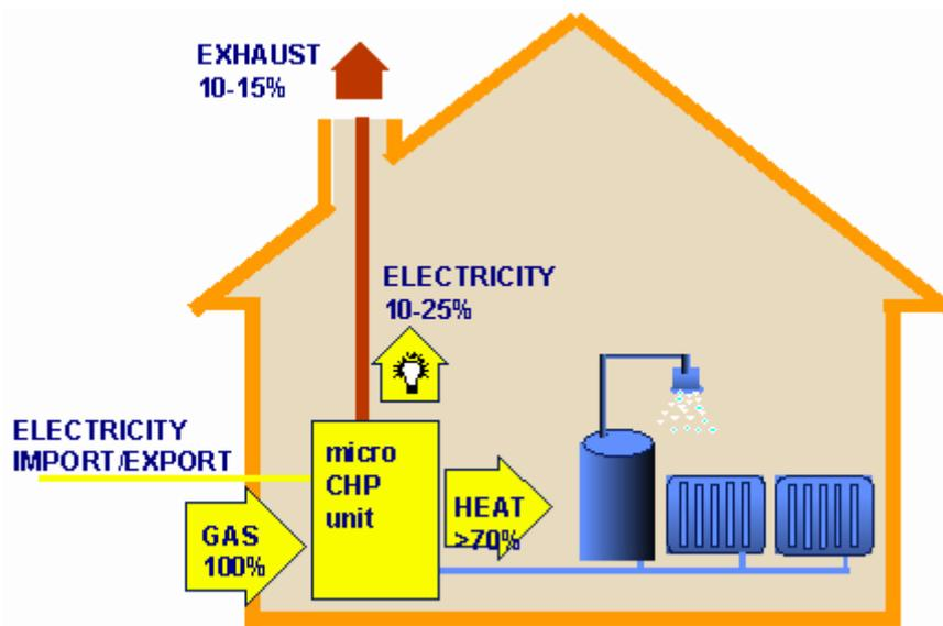
Figure 5: Micro-CHP process <sup>[22]</sup>
