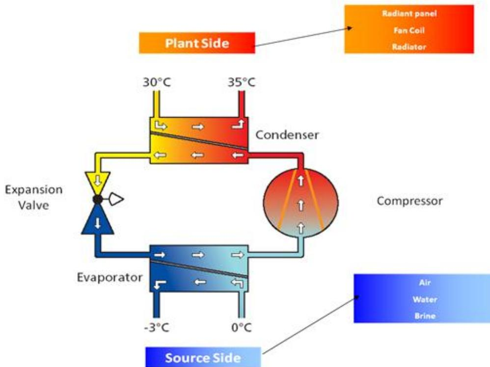
Figure 1: Components that make up a heat pump <sup>[5]</sup>
