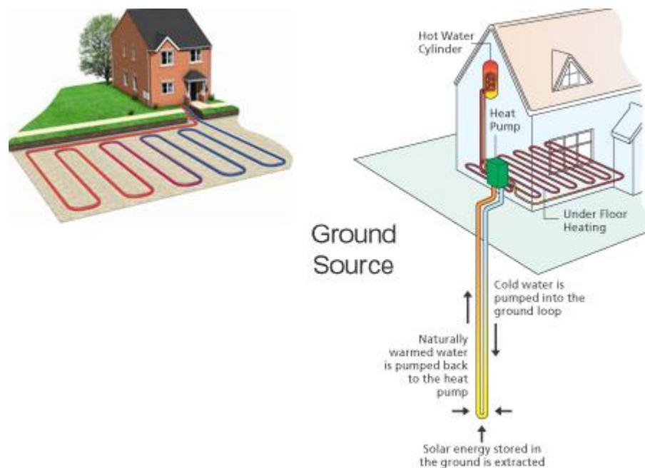
Figure 4: Horizontal and vertical loop configurations [13-14]
