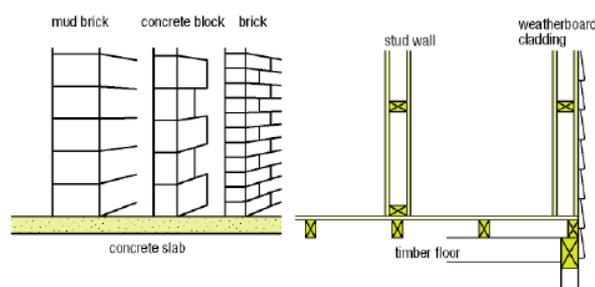
Figure 7: Materials with high and low thermal storage capacity<sup>[29]</sup>
