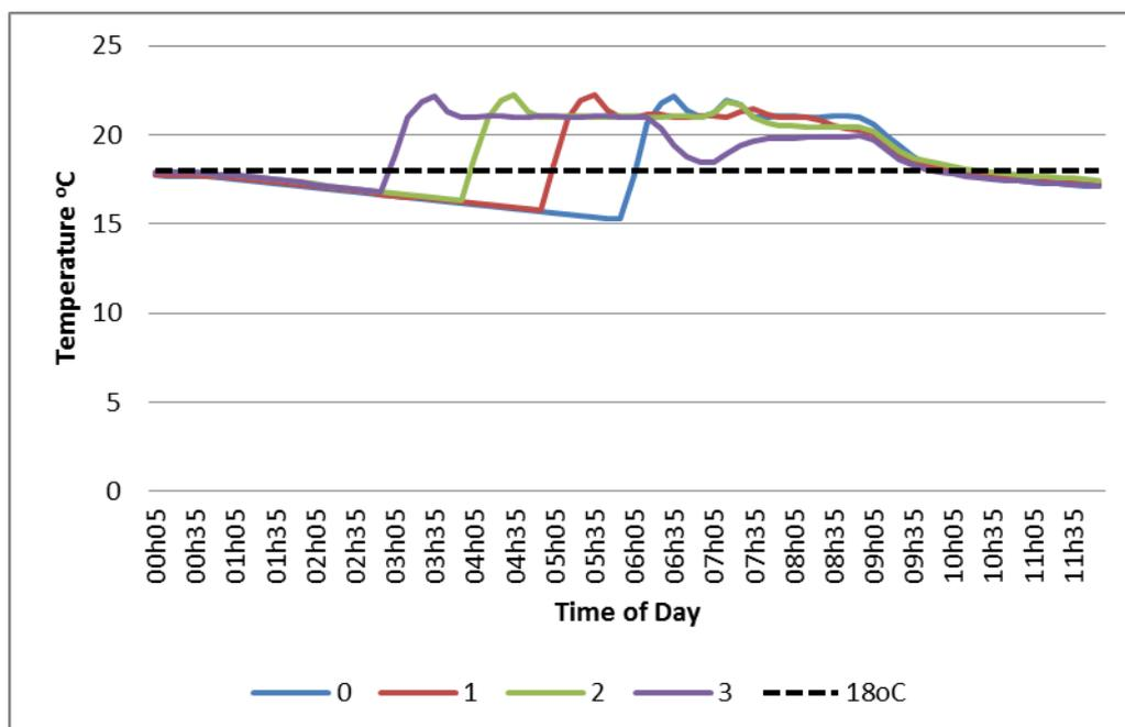
Figure 13: Effect of back-shifting the heat input for first half of the day (Passiv)
