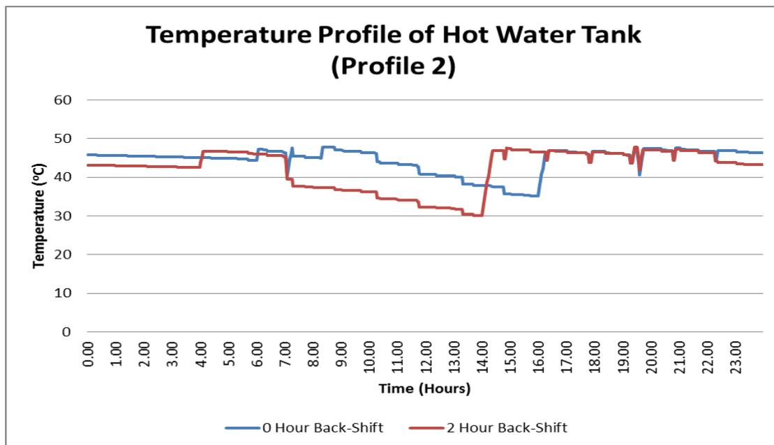
Figure 17: Temperature profile within hot water tank (profile 2)
