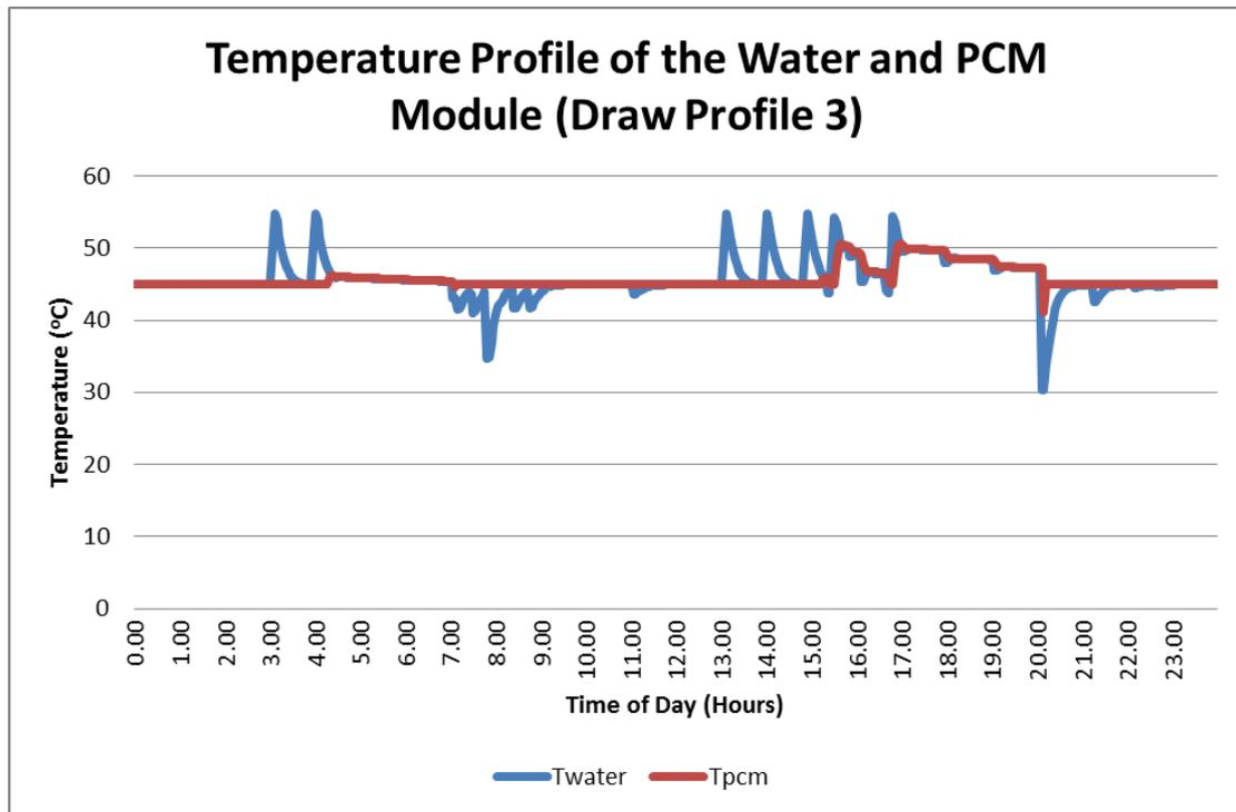
Figure 24: Temperature profile of the water and PCM module (Profile 3)
