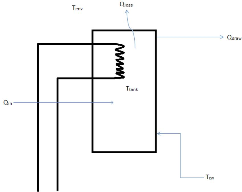
Figure 8: Schematic of a hot water tank
