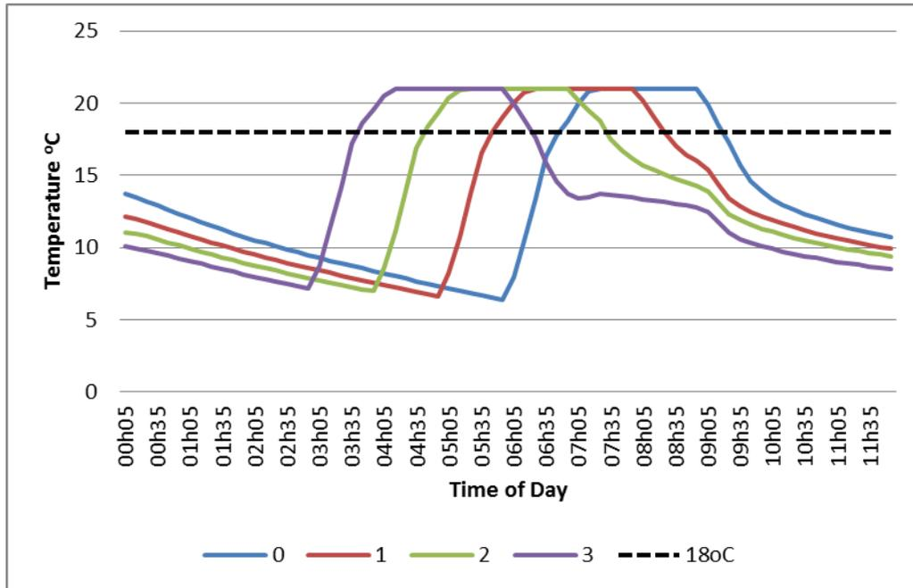
Figure 11: Effect of back-shifting the heat input for first half of the day
