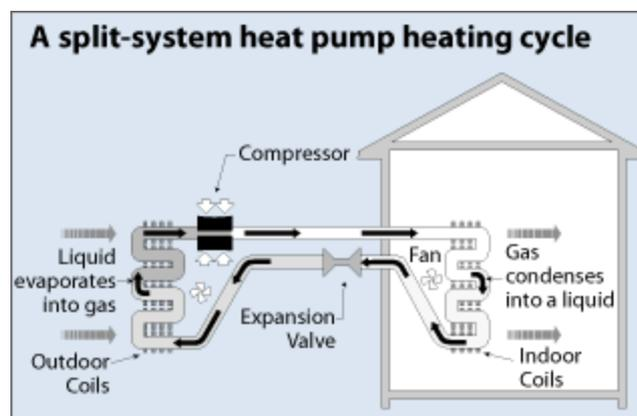
Figure 3: ASHP heating cycle <sup>[10]</sup>
