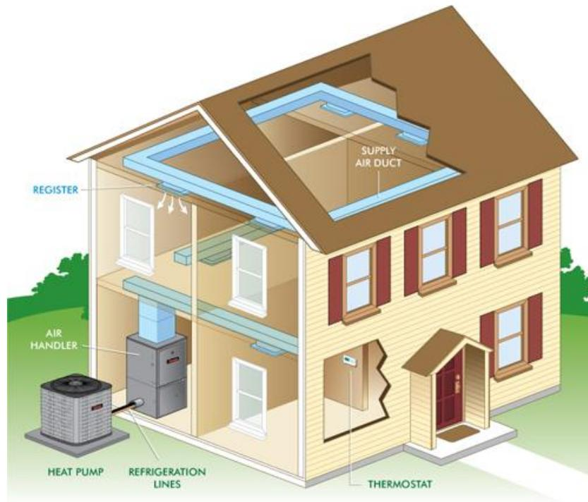
Figure 2: Air source heat pump installation <sup>[9]</sup>
