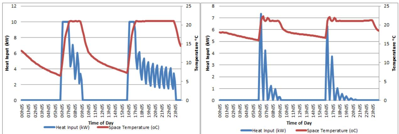
Figure 10: Graph showing temperature variation (Average and Passiv)
