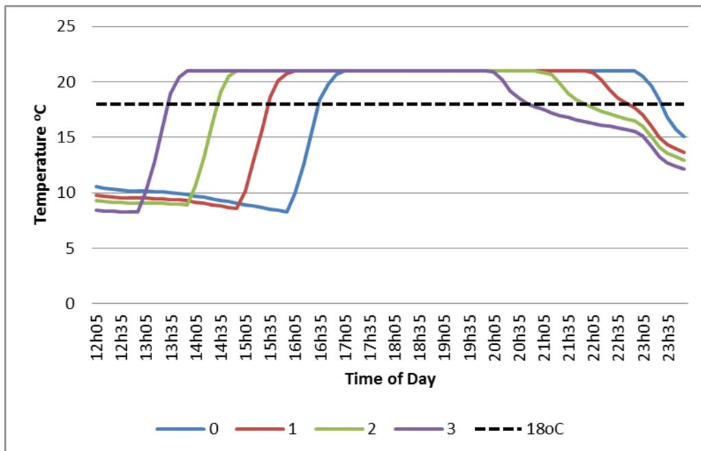
Figure 12: Effect of back-shifting the heat input for second half of the day
