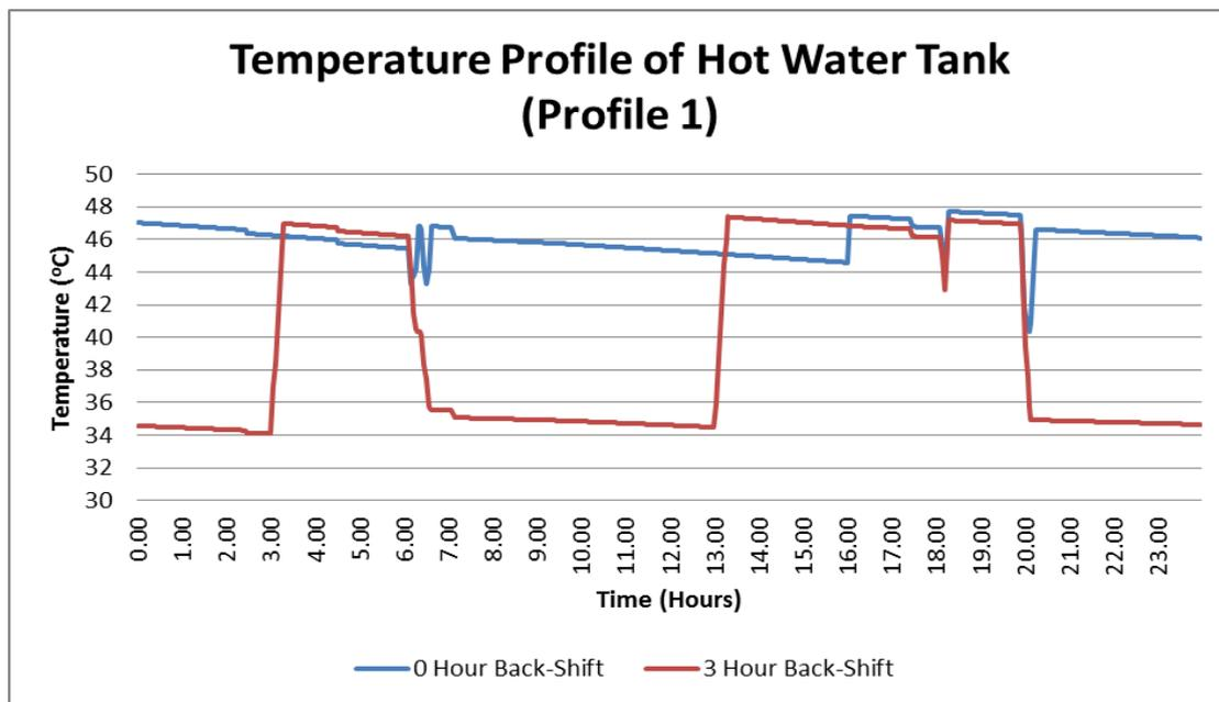
Figure 16: Temperature profile within hot water tank
