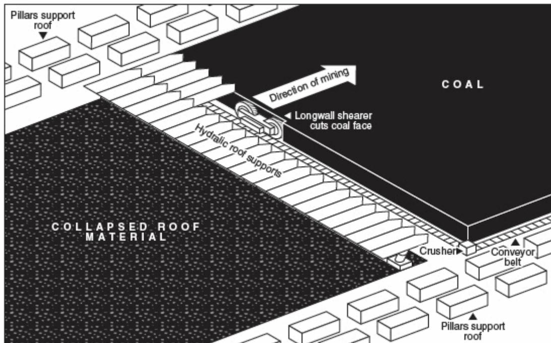
Fig 2.3.2. Longwall mining (taken from <http://rajikorba.blogspot.com/2011/06/long-wall-technology-in-coal-mines.html>)
