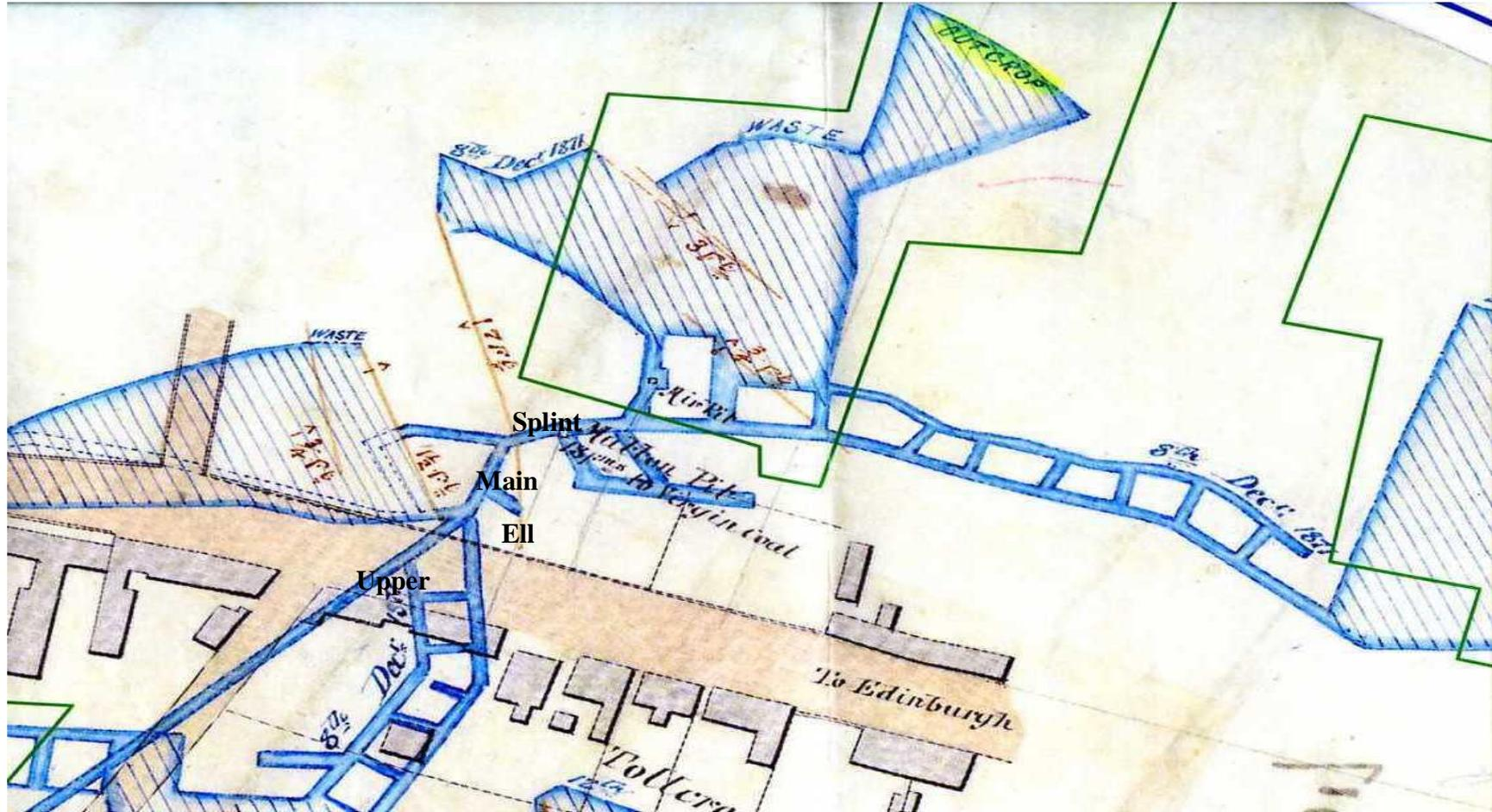
Fig 6.1.2, Abandonment plan for the Mutton pit Shaft, Tollcross colliery (Supplied by the BGS)
