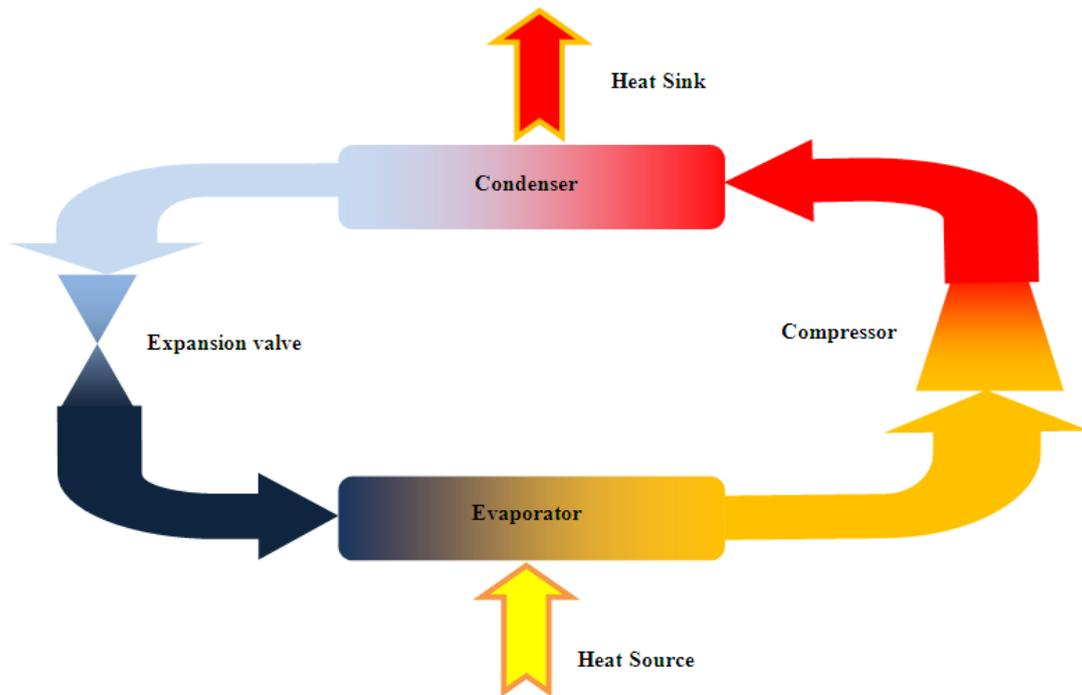
Fig 2.2.1. Components of a heat pump
