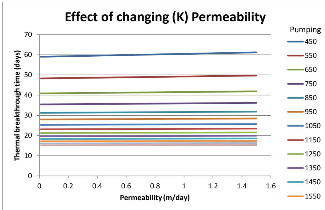
Fig 6.1.10 Effect of changing K and Z on thermal feedback times.
