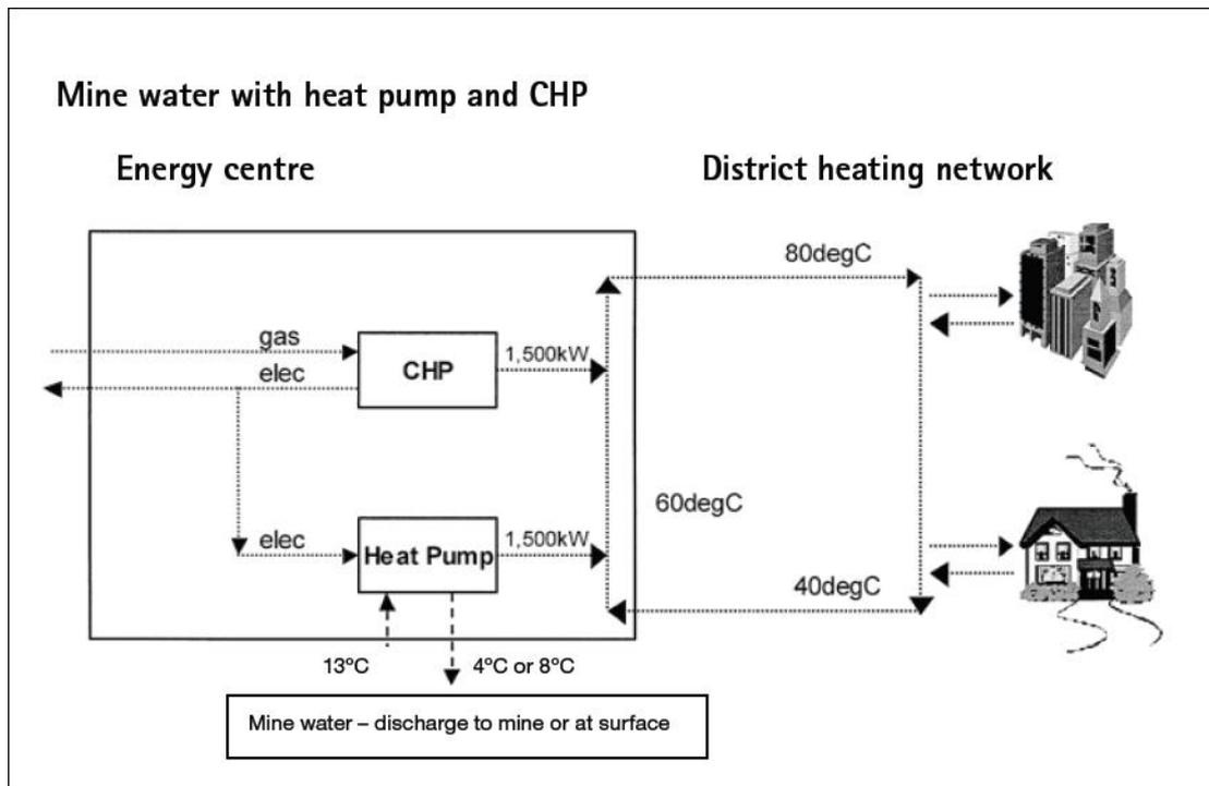
Fig 2.5.1. Heat pump and CHP heating system (taken from minewater project paper)
