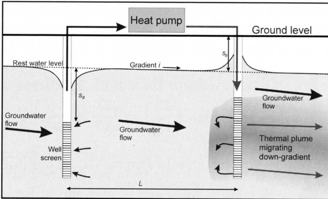
Fig 4.1. Well doublet with no thermal feedback (Banks 2008, p167)
