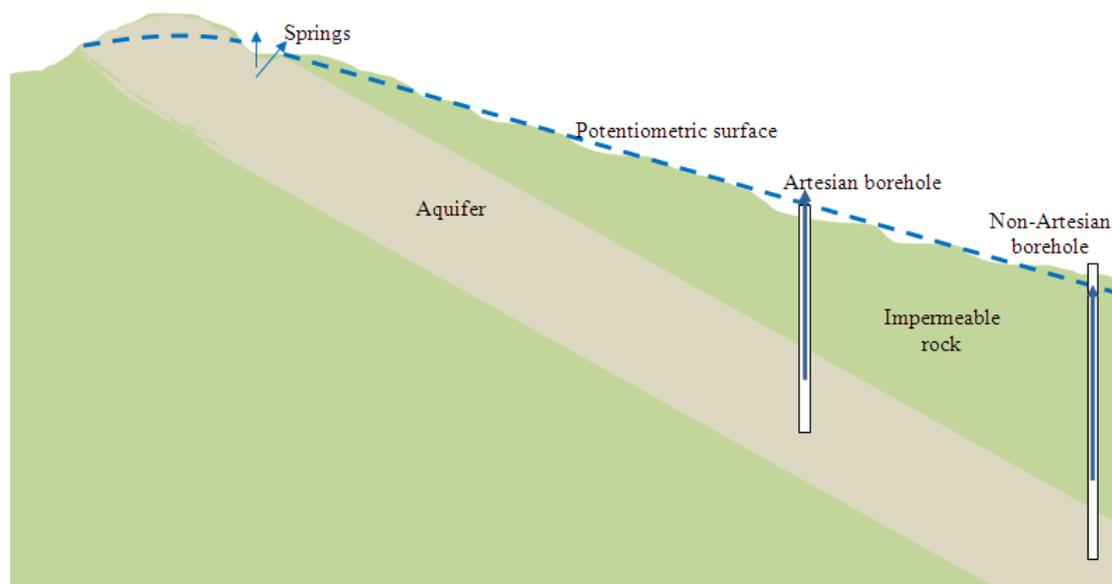
Fig 3.2.3.1 Artesian borehole
