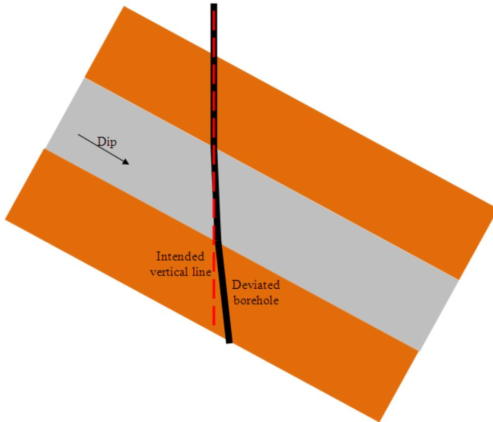
Fig 6.2.5. Red dotted line indicates the vertical borehole while the black line shows how the borehole can move each time it passes through a different horizon.
