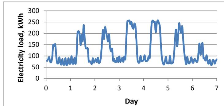
Figure 16 Typical summer week (1-7<sup>th</sup> August, 2010), electricity load, kWh
