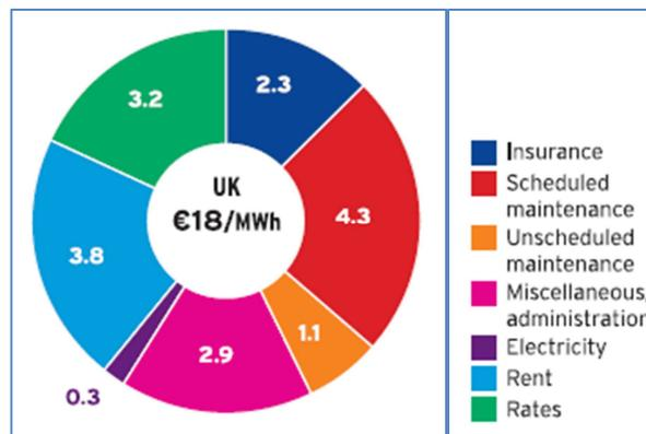
*Figure 31 Total operation and maintenance costs per MWh of wind energy
