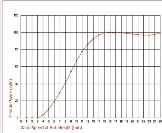
Annual Energy Production\*: 21-Meter Rotor Standard Air Density (1.225 kg/m<sup>3</sup>)
