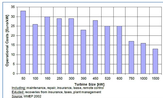
Figure 33 Operational costs as a function of the turbine size (WMEP, 2002 cited in (Wiggelinkhuizen, 2007))
