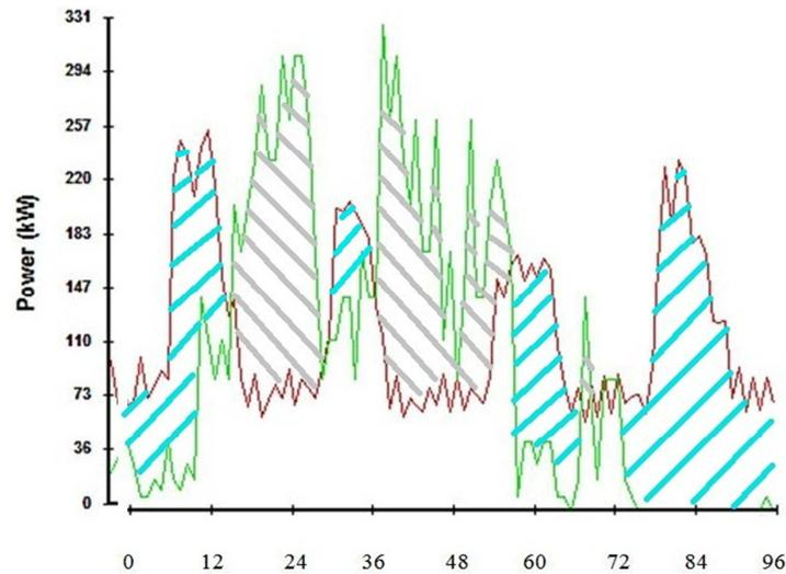
*Figure 28 Example of demand (red) supply (green) profile, 16/07-19/07 based on 330kW wind turbine energy output*
