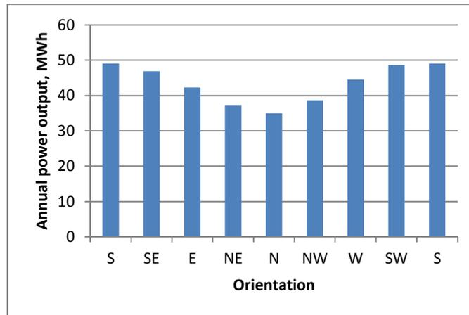
Figure 18 Annual power output at different orientations.
