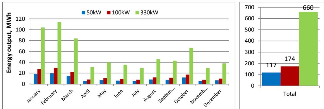
Figure 24 Energy generation by wind turbines 50kW, 100kW and 330kW of rated power
