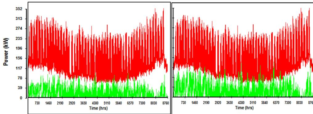
Figure 27 Power output profile for 50kW PV and 50kW wind turbine (left), and 50kW PV and 100kW wind turbine (right)
