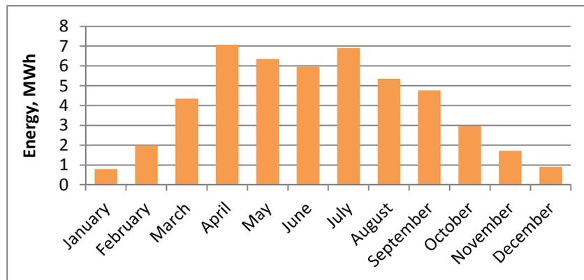
Figure 22 50kW solar PV energy generation, monthly distribution.
