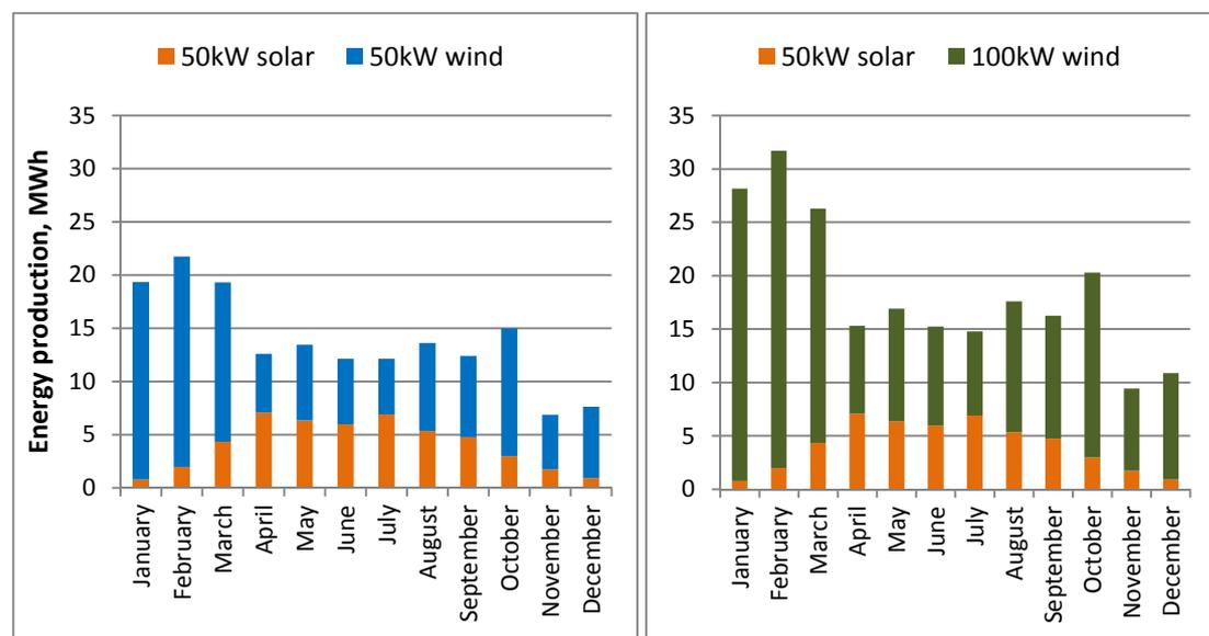
Figure 26 Energy production per month by two combinations of equipment
