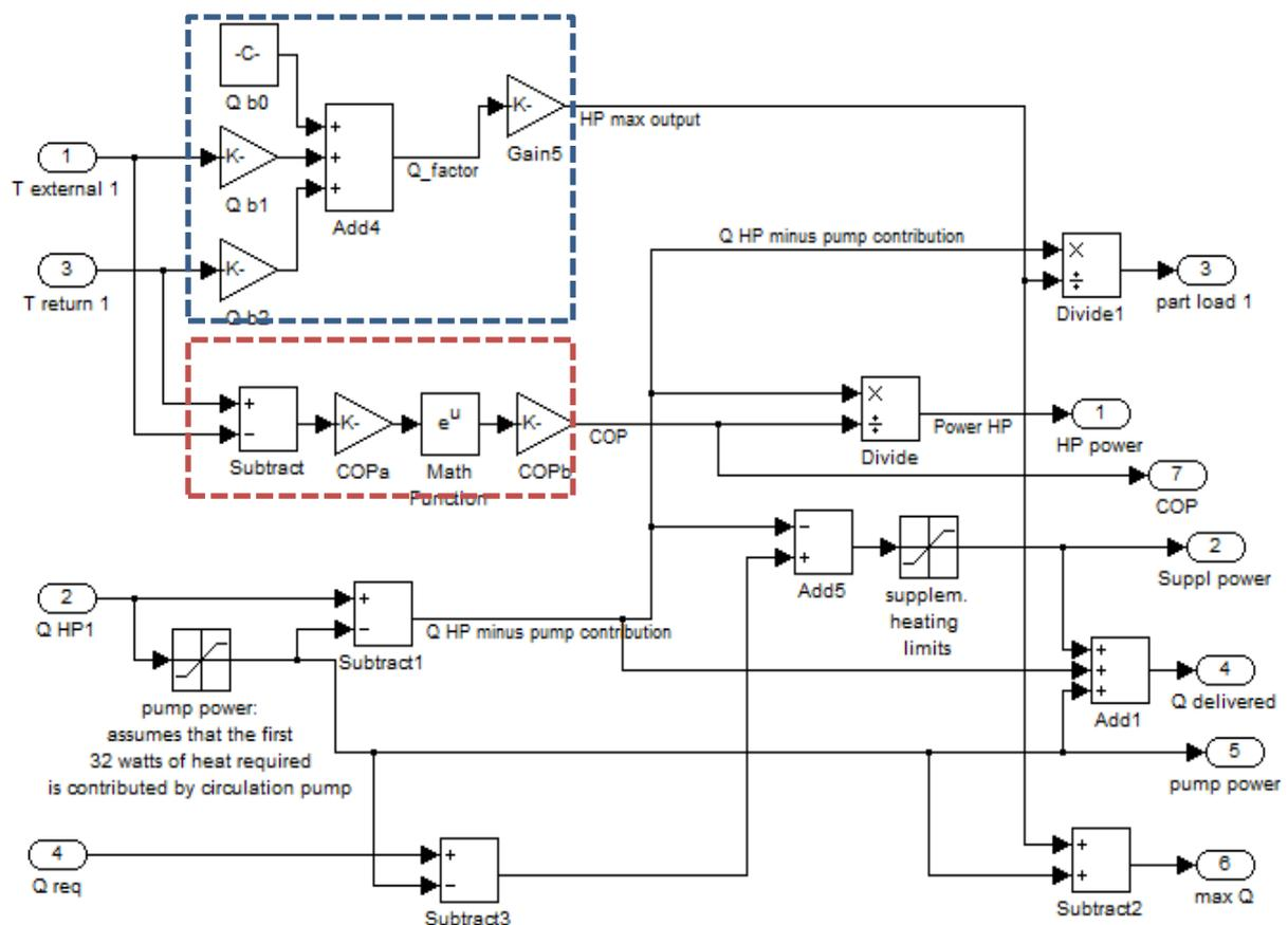
Figure A.3 depicts the heat pump subsystem for the case where supplementary heating is provided by a separate system. As the rate of heat output of the heat pump is already determined by the radiator subsystem, this serves two main functions: calculation of the heat pump's maximum output for the next timestep; and calculation of the power drawn by the heat pump.
