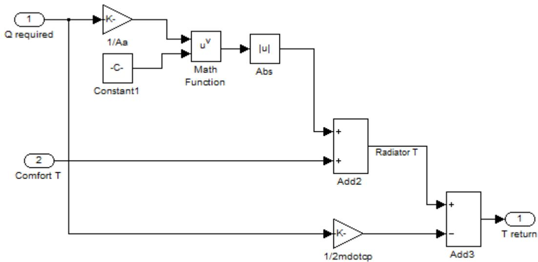
The version of the heat pump subsystem for the integrated supplementary heating case is similar to that for the separate supplementary heating case. It is depicted in figure A.5 below. A key difference is that the contribution of the heat pump to the heat output of the radiator system is limited by its maximum output. This is achieved by the block highlighted by a blue rectangle. Any deficit is assumed to be made up by the supplementary heater with 100% efficiency.
