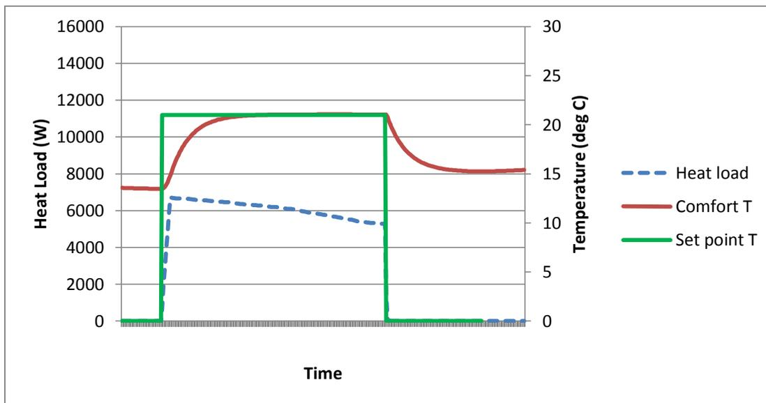
This approach to accounting for responsivity is necessarily an approximation in that, however low the temperature has dropped during a set back period, it recovers in the same amount of time. However it appears none the less to result in well-controlled heat demands, without excessively large spikes at the start of heating periods.
