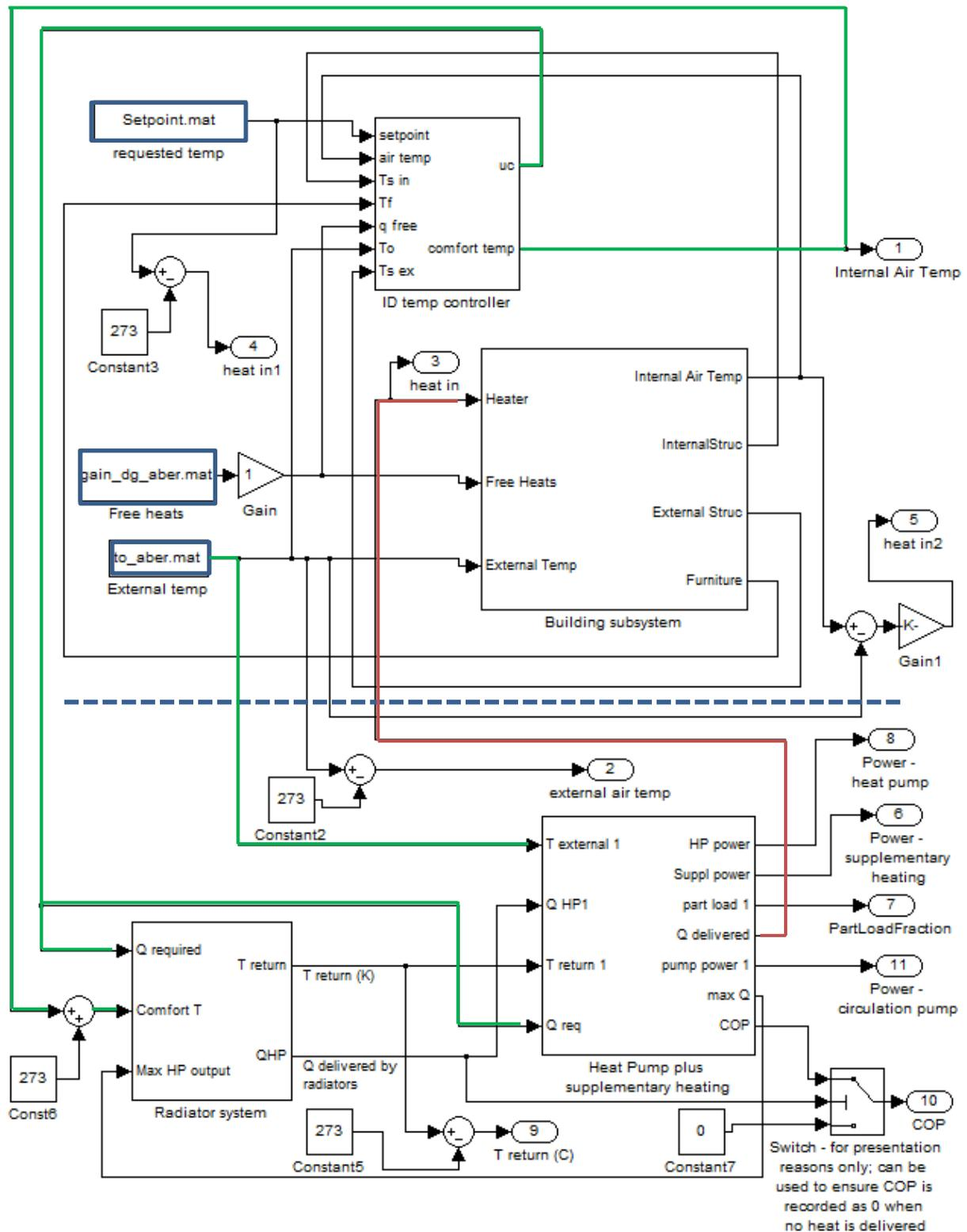
Figure A.2 depicts the version of the radiator subsystem relating to the case where supplementary heating is supplied separately from the heat pump system. The input signals from the top level of the model arrive at the oval blocks on the left.
