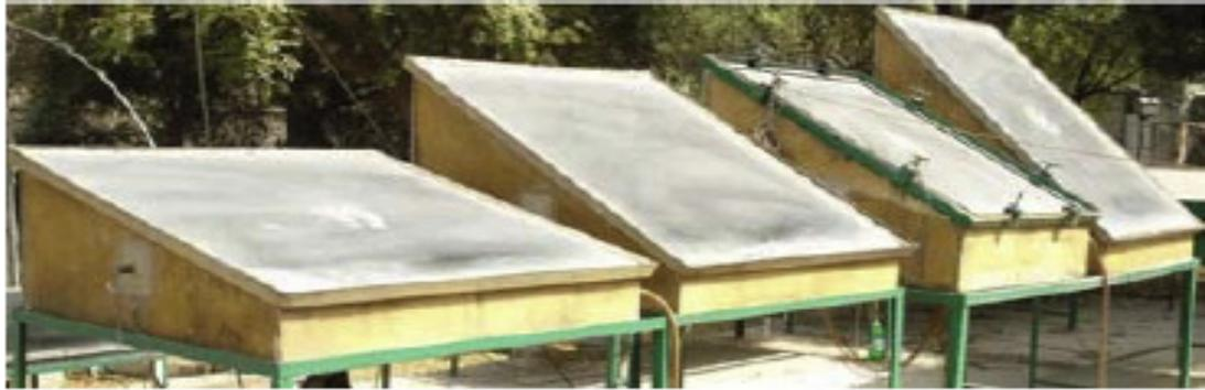
Figure 6: Basin-type Solar Stills having varying Angles of Inclination [18]
