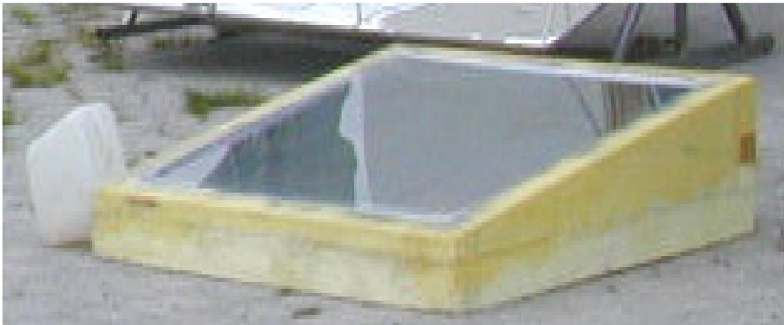
Figure 3: A typical basin-type solar still [9]
