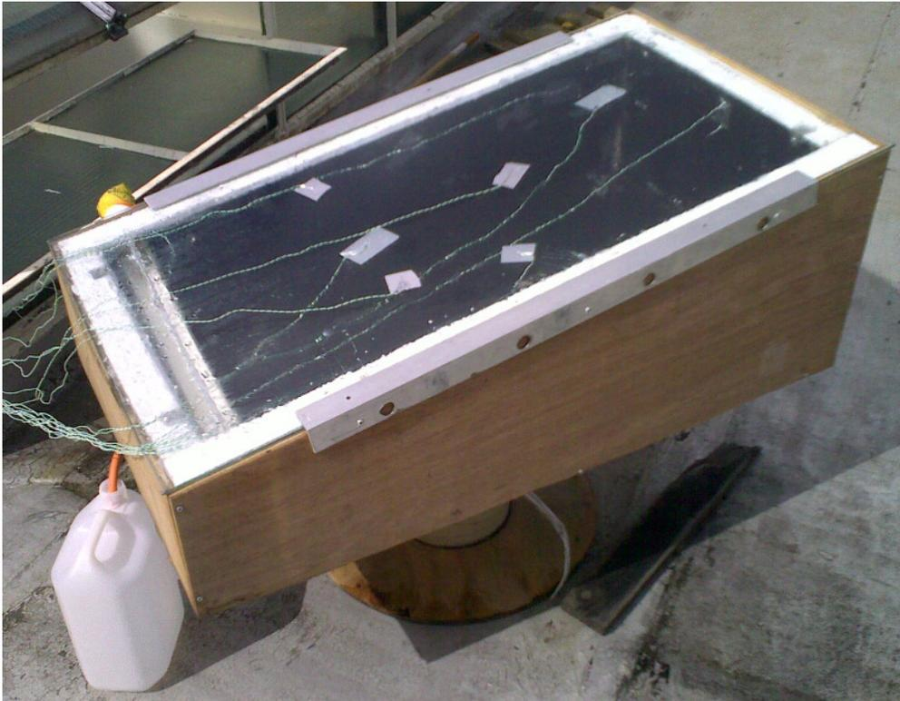
Figure 9: Showing the still and the attached type-K thermocouples
