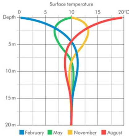
Figure 7: Ground Temperature throughout the year at different depths (Filterclean n.d.).
