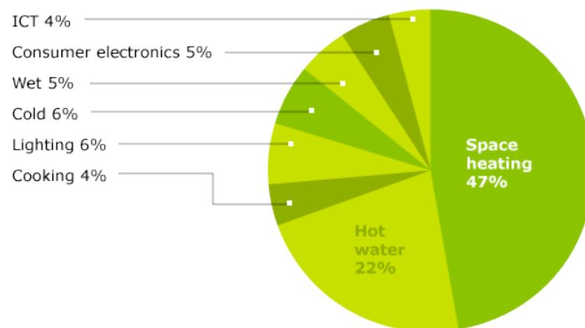
Figure 1: Domestic CO<sub>2</sub> emissions by end use in the UK (Guardian 2010)
