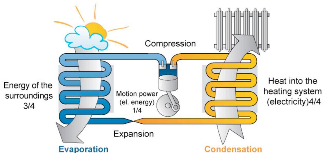
Figure 3: The heat pump cycle (Setrime n.d.)
