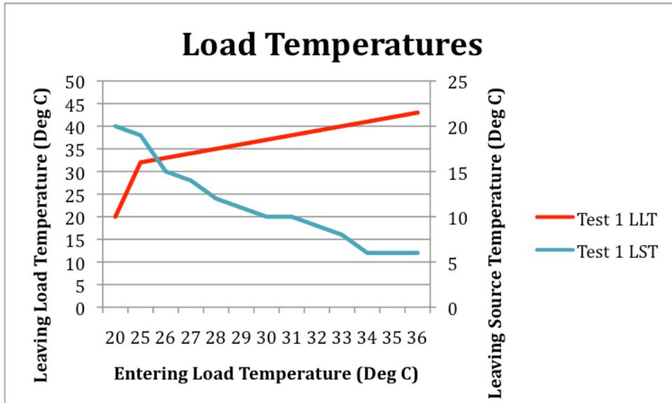
Figure 20: Load Temperature changes for experiment 2.
