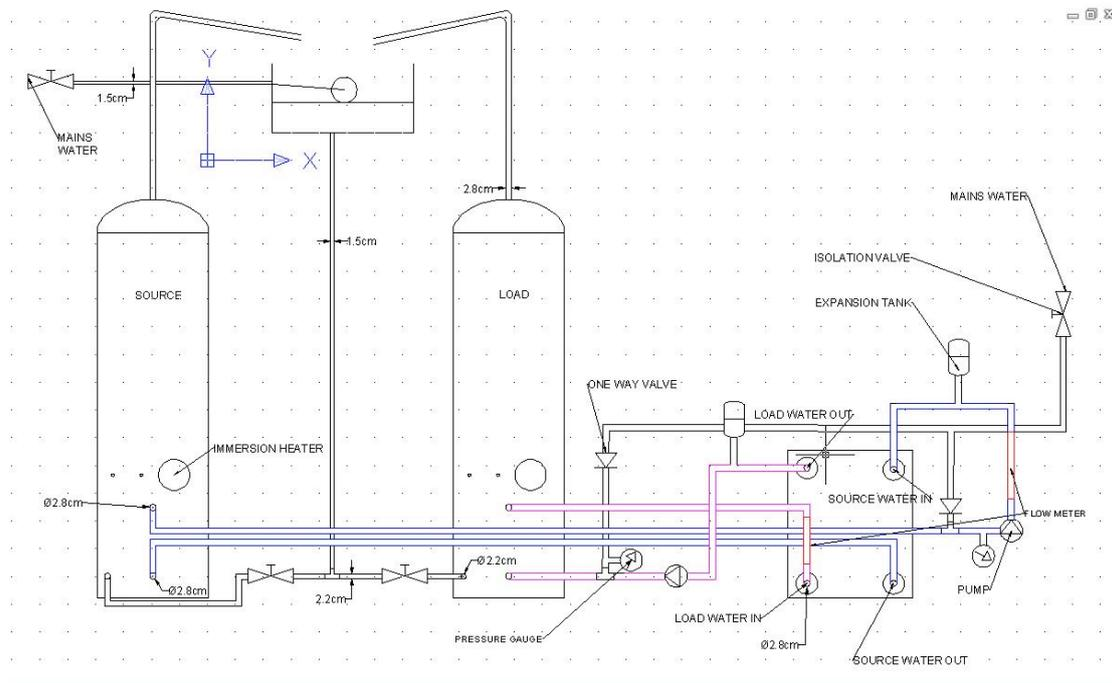
**Figure 16: Basic setup of the test rig.**
