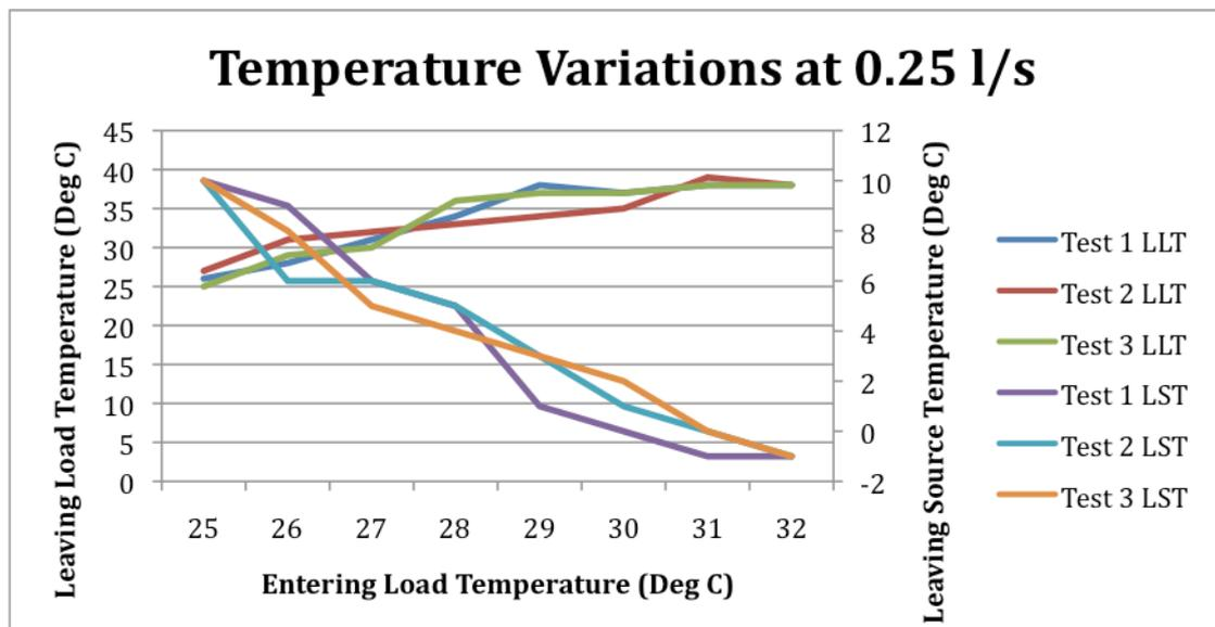
Figure 17: ELT, LLT and LST at a flowrate of 0.25 l/s for experiment 1.
