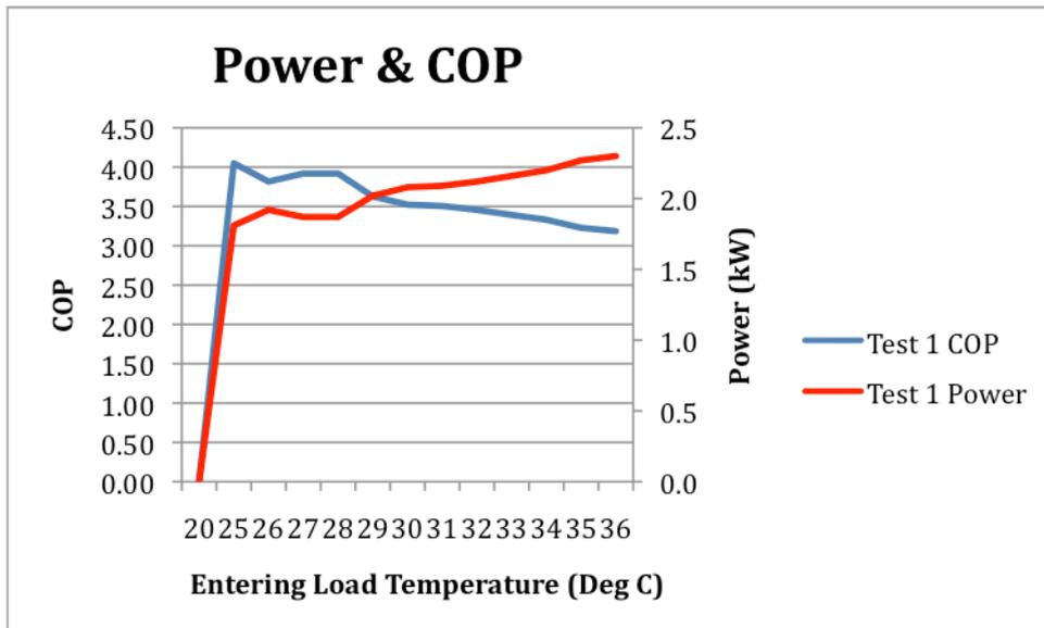
Figure 21: Power consumption and COP for experiment 2.
