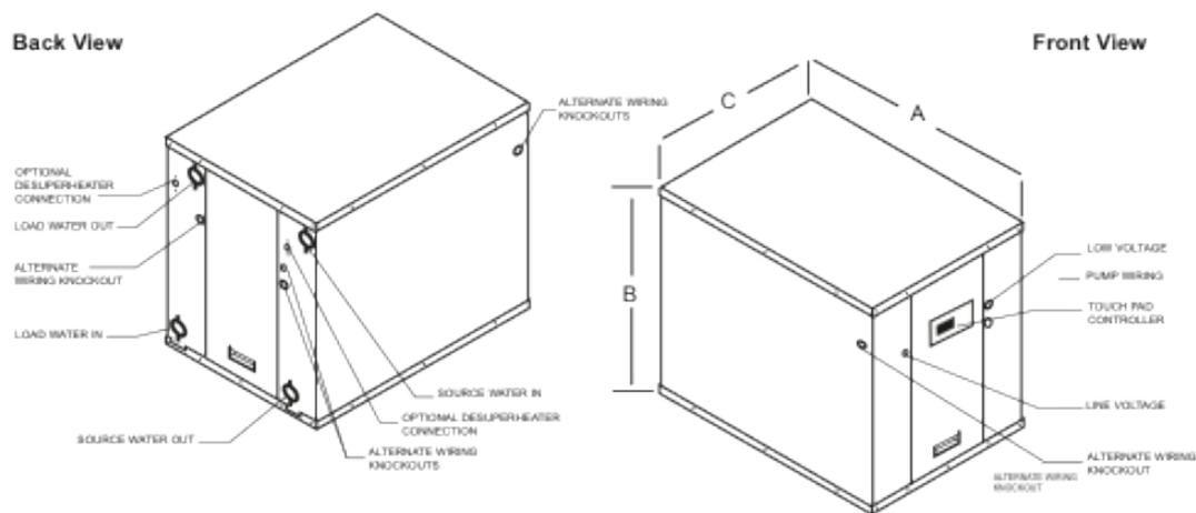
**Figure 14: Waterfurnace 8kW Hydronic Heat Pump**
