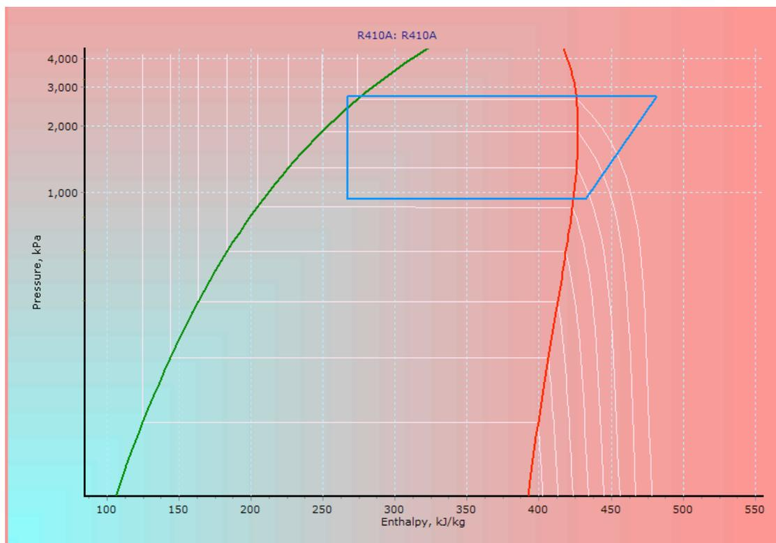
**Figure 25: Pressure Enthalpy diagram for Refrigerant R401a.**
