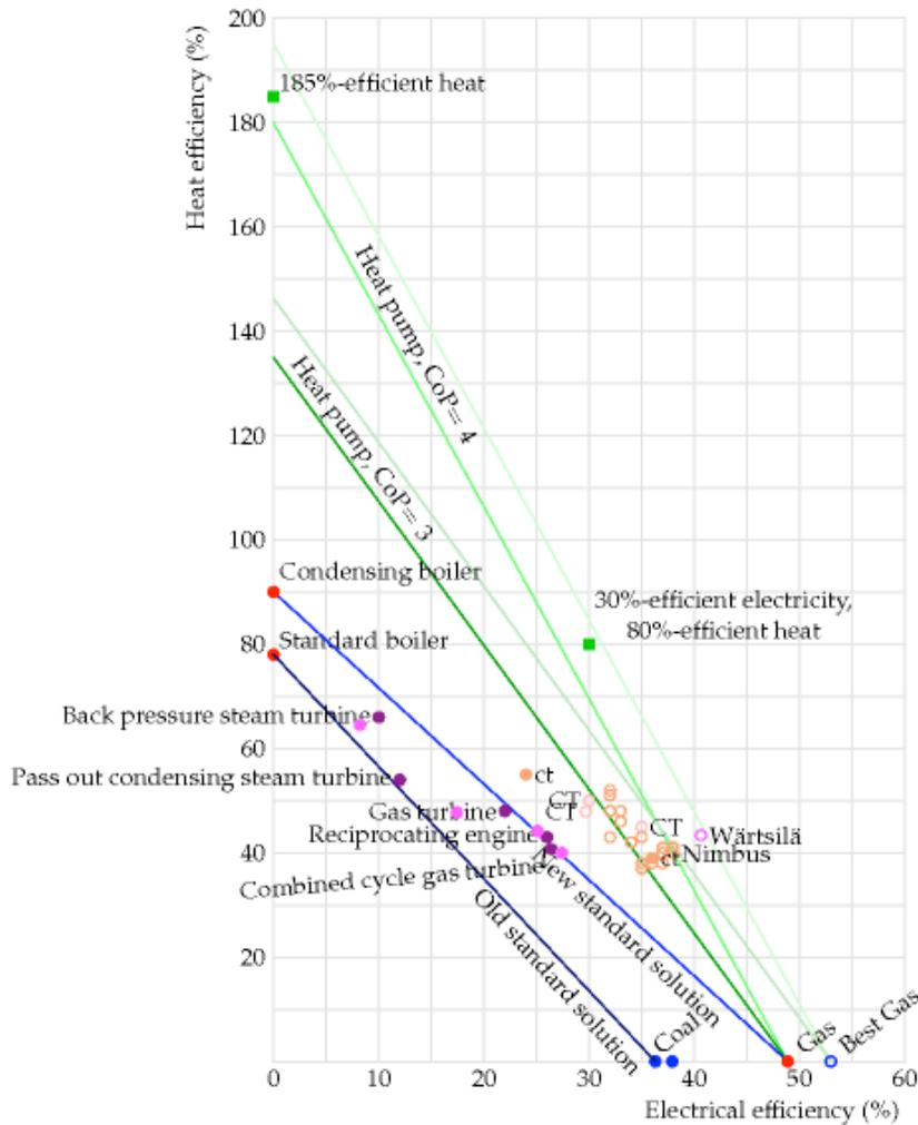
Figure 7: The Effectiveness of a heat pump compared to other technologies (MacKay 2009)
