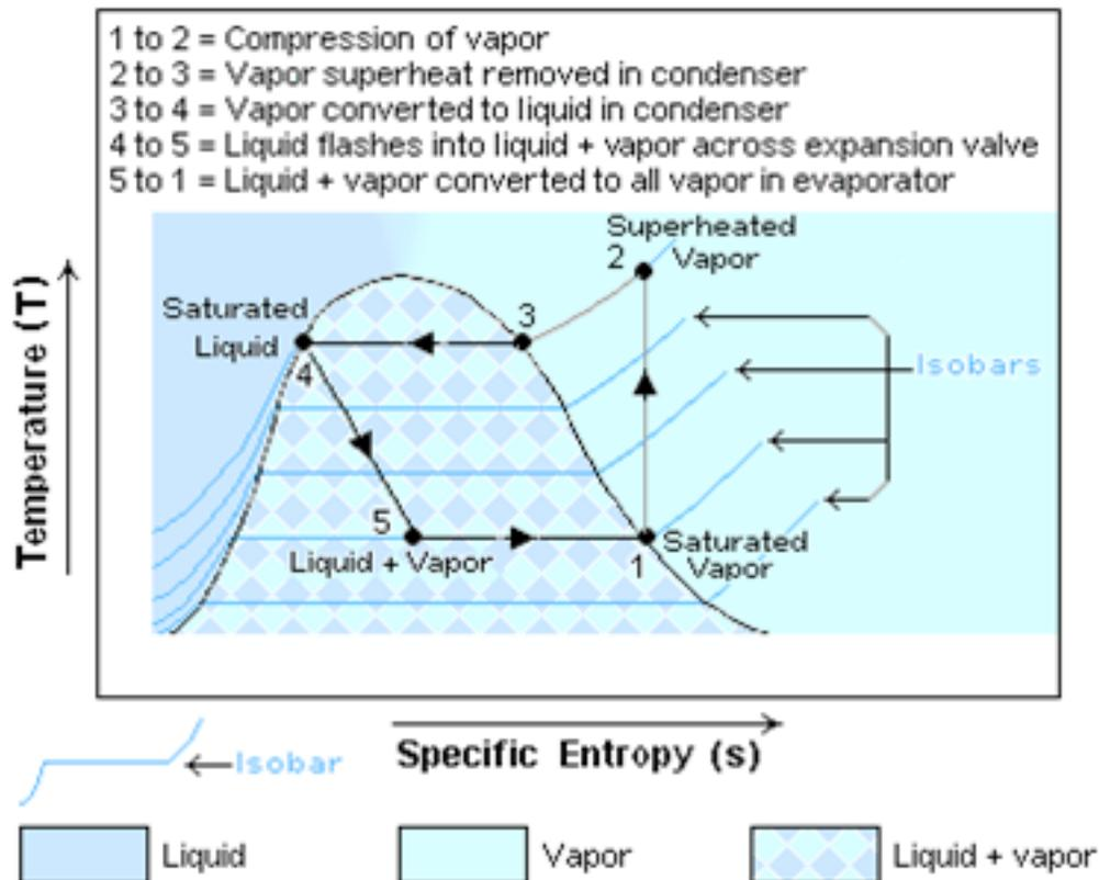
Figure 4: The T-s diagram for a typical refrigerant used in a heat pump.
