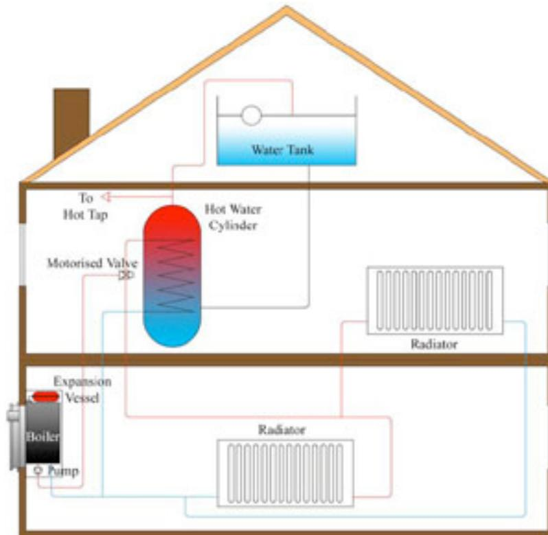
Figure 8: Gravity Fed hot water system (AquaBrand n.d.).
