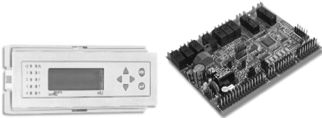
Figure 26: The medium user interface for the EKW08 and the FX10 Controller mainboard.
