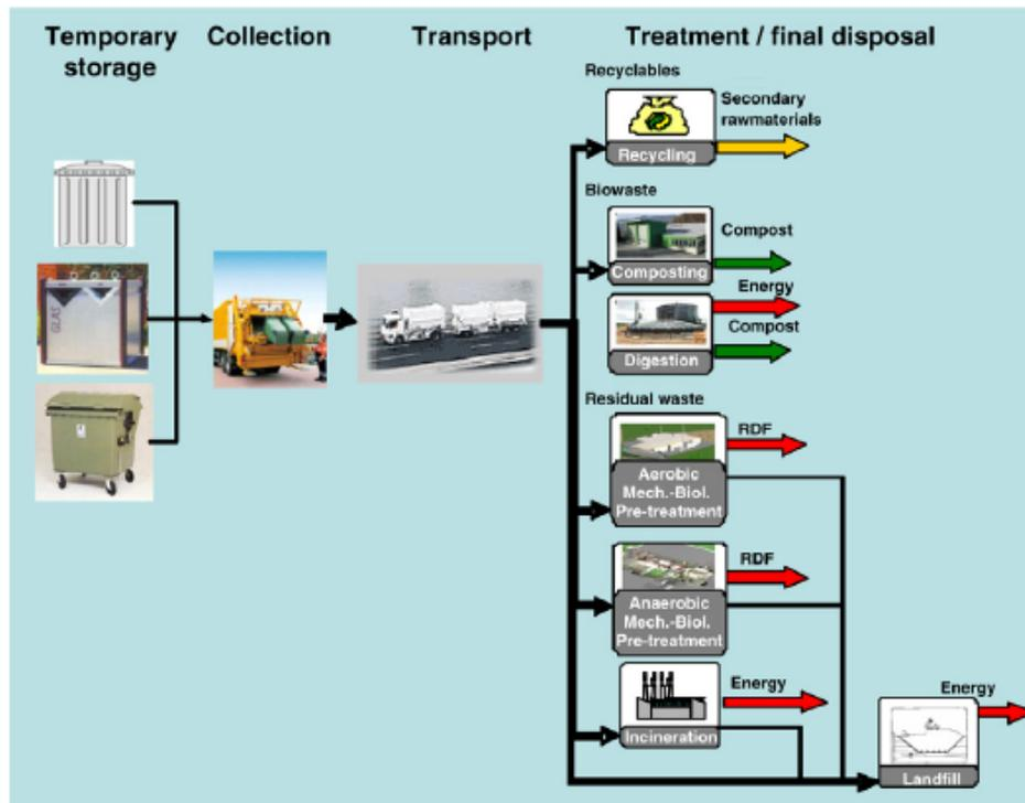
**Figure 6:** An Integrated Waste Management System in the LCA-IWM Assessment Tool
