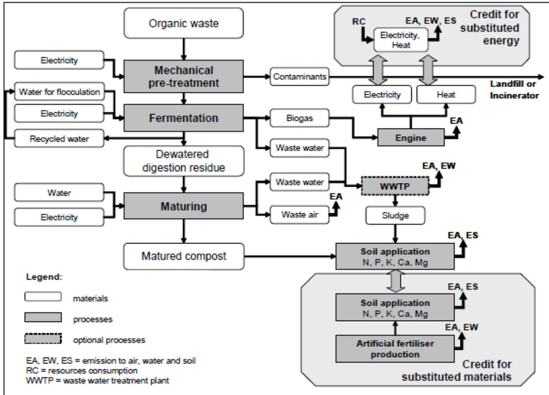
**Figure 18:** Main Material Flows in the Modeled Anaerobic Digestion System
