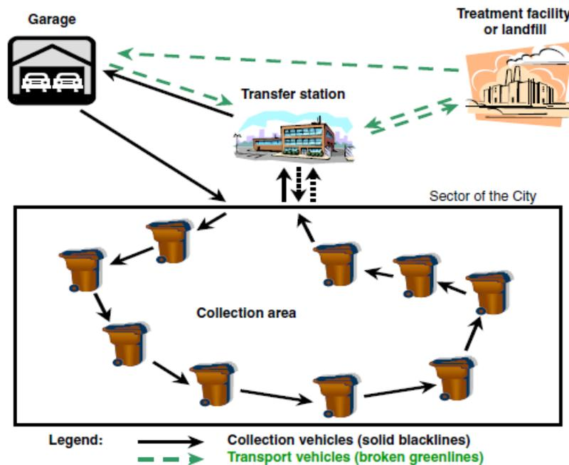
**Figure 4:** Collection and Transport Scheme with Transfer Station
