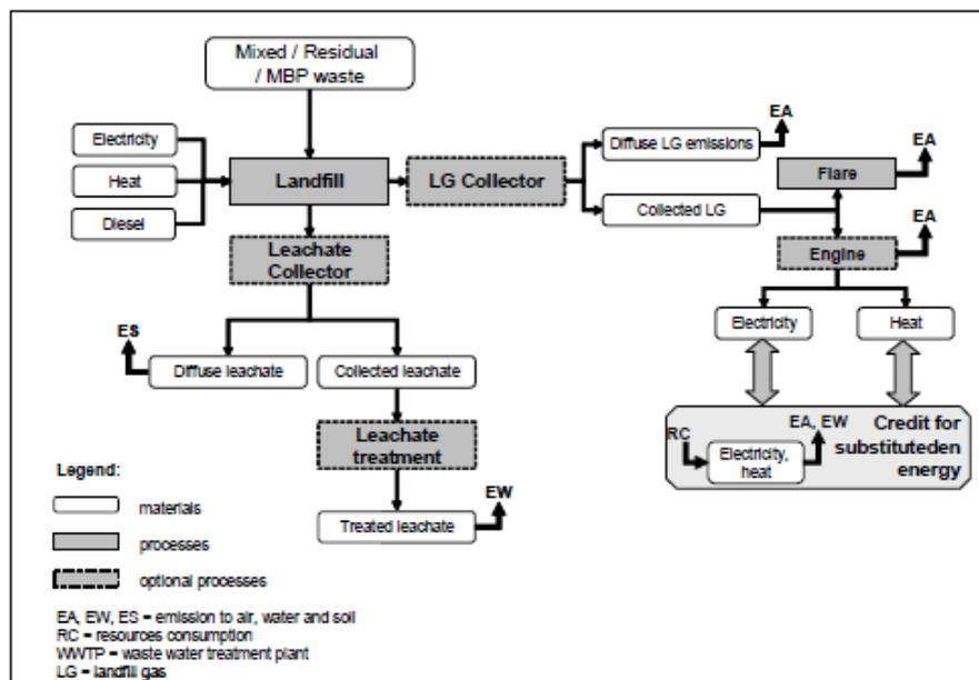
**Figure 20:** Main Material Flows in the Modeled Landfill
