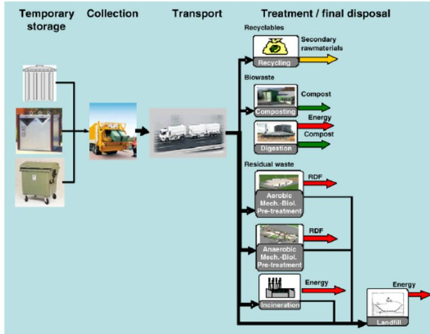
**Figure 1:** An Integrated Waste Management System Containing all the Background Modules of the LCA-IWM Assessment Tool
