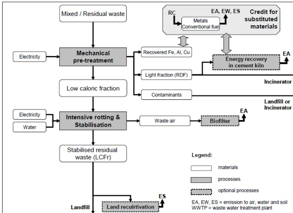
**Figure 19:** Main Material Flows in the Modeled Aerobic MBP System
