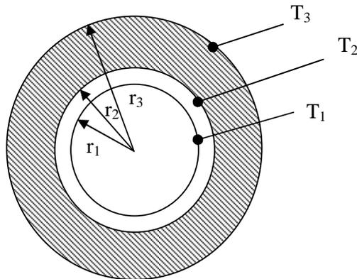
Figure 11 Composite cylinder
