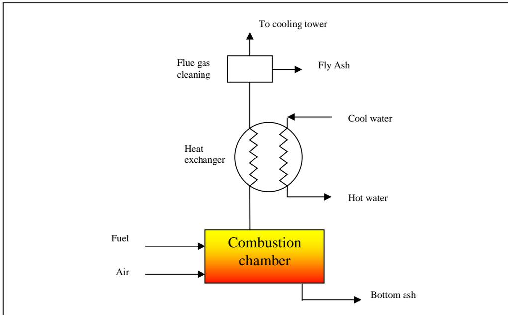
*Figure 7 Biomass boiler*
