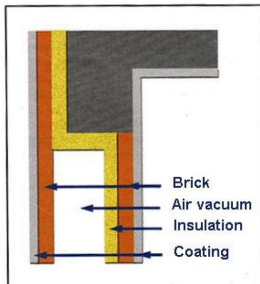
Figure 2.3.6-3: Two-layer insulation with air vacuum [9]
