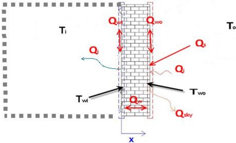
Figure 5.5-1: New built construction exposed to climatic data with variable dimensions
