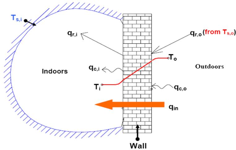
Figure 4.2-1: Homogeneous wall separating a conditioned indoor space from the outdoor environment
