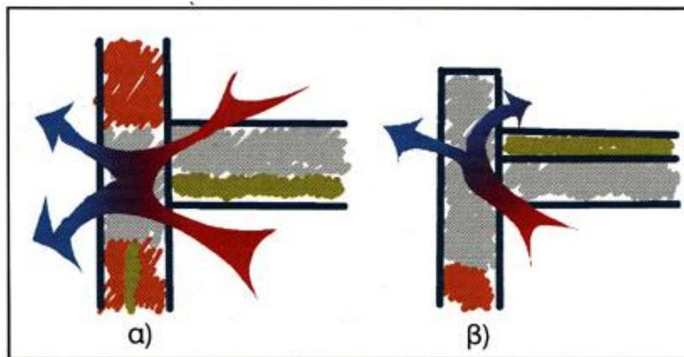
Figure 2.3.6-1: Thermal bridges a) Beam b) Roof [9]
