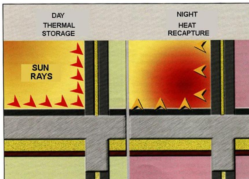
Figure 2.3-1: Function of the floor and walls thermal mass during the day and the night in winter [9]
