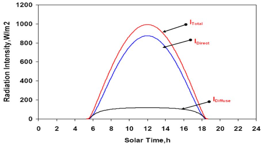
Figure 4.4.2-1:: diffuse, direct, total solar radiation on horizontal surface (clear sky)
