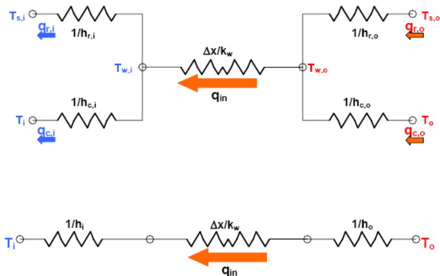
Figure 4.2-2: Heat transfer network considering various heat transfer resistances
