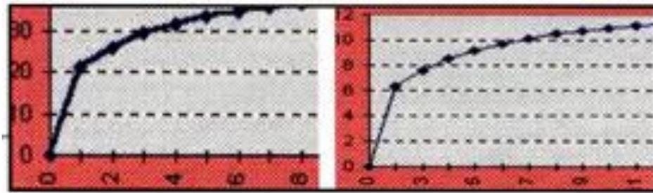
Figure 2.3.6-2: Energy gain due to increase in thickness in the external insulation on a side wall (left) and on the roof (right). Horizontally = the insulation thickness / Vertically = Energy gain in % [9]
