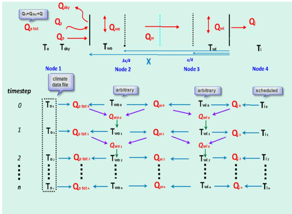
Figure 5.2-1: Time step node temperatures through steady state equations
