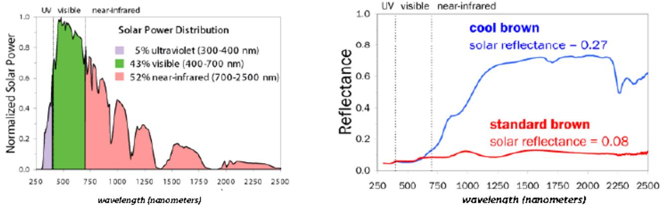
Figure 3.1.2-1: Solar power distribution and a comparison between conventional and cool coatings of the same colour
