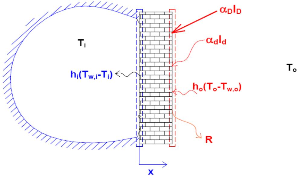
Figure 4.4.1-1: Unsteady state heat transfer through a building construction element
