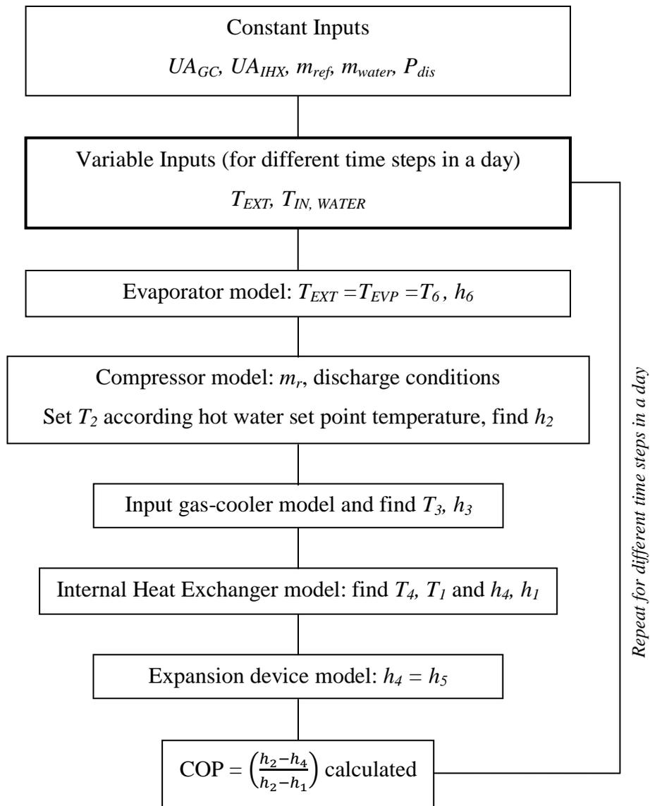
**Figure 4.2.2.1.1** Flow chart for the numerical simulation
