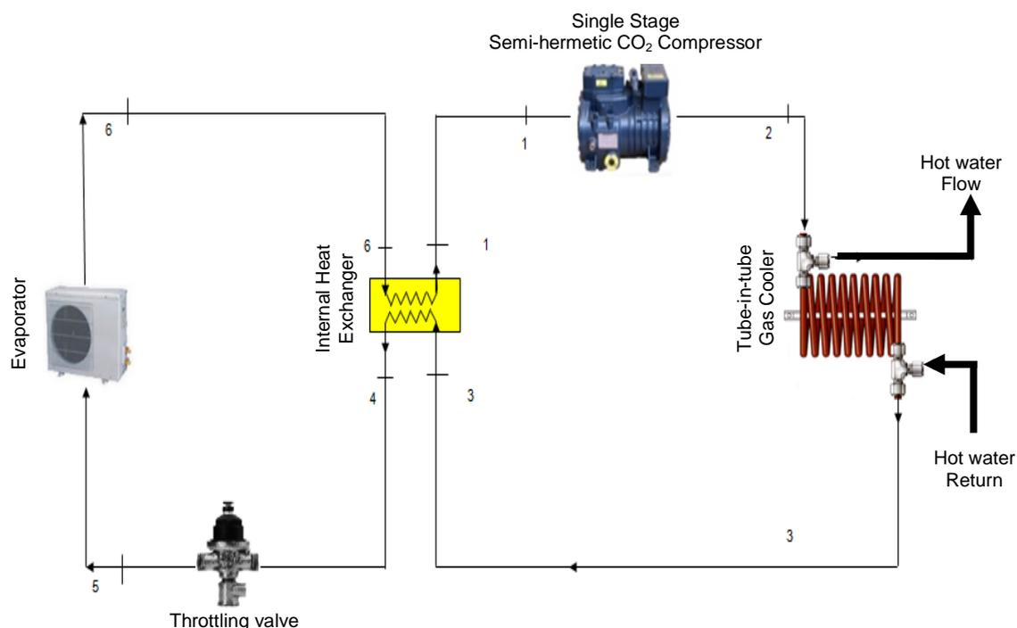
*Figure 4.2.1.1 Transcritical CO<sub>2</sub> Heat pump simulator*
