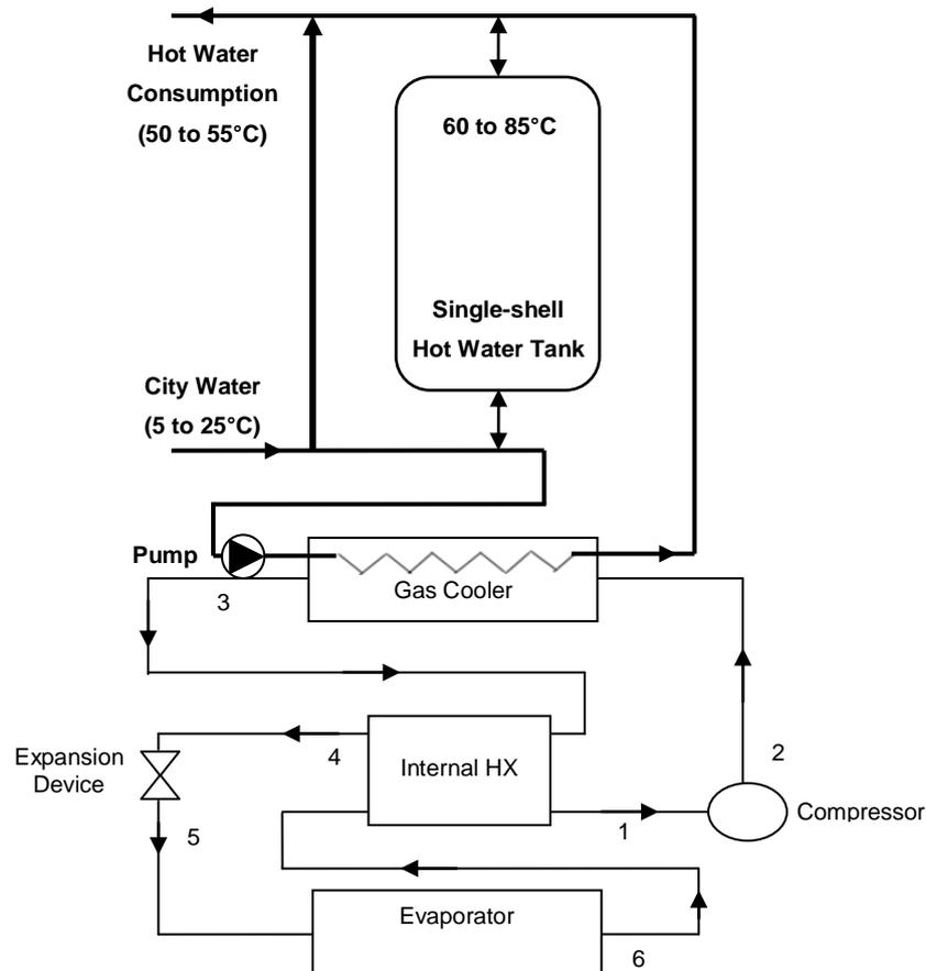
**Figure 2.1.1 Simple CO<sub>2</sub> heat pump water heater**
