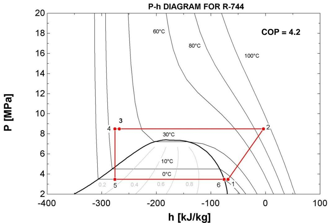
*Figure 4.2.3.2.6 P-h diagram of a CO<sub>2</sub> heat pump system, when hot water temperature profile 80/10°C, high-side pressure of 8.5 MPa. Developed with EES*
