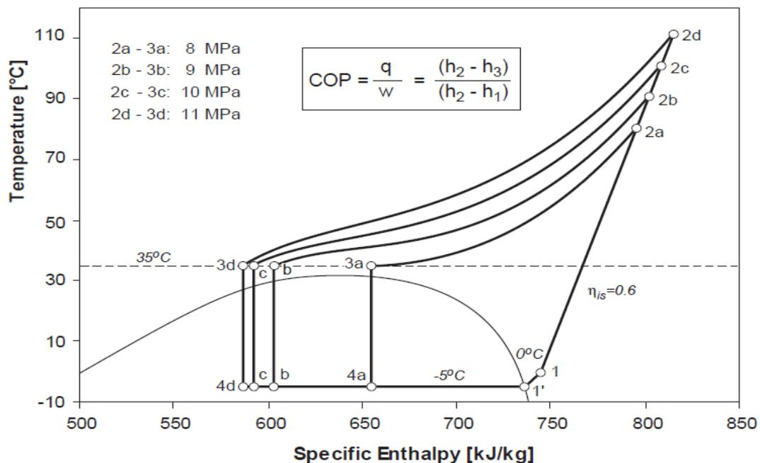
**Figure 4.1.3.3.1** the transcritical CO<sub>2</sub> heat pump cycle operated at four different high-side pressures and gas-cooler outlet temperature assumed to be constant at 35°C (Source: CO<sub>2</sub> heat pump for combined SH and DHW)
