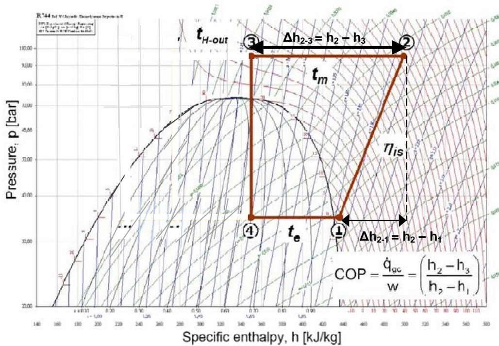
**Figure 4.1.1.1** P-h diagram for COP of simple transcritical CO<sub>2</sub> heat pump cycle
