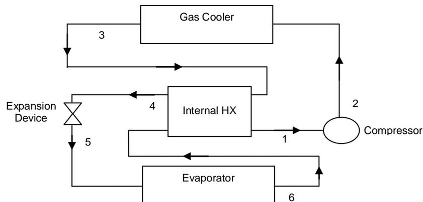
**Figure 1.5.1 Layout of transcritical CO<sub>2</sub> system with internal heat exchanger**
