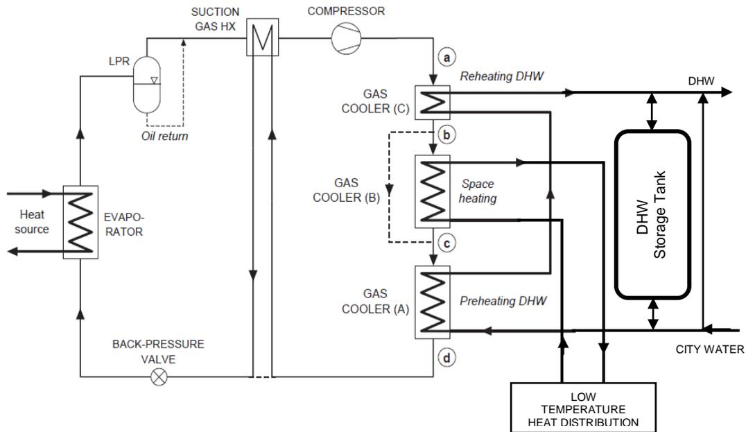
**Figure 2.2.1 Principle design of Integrated CO<sub>2</sub> heat pump for space and DHW heating for Passive housing**
