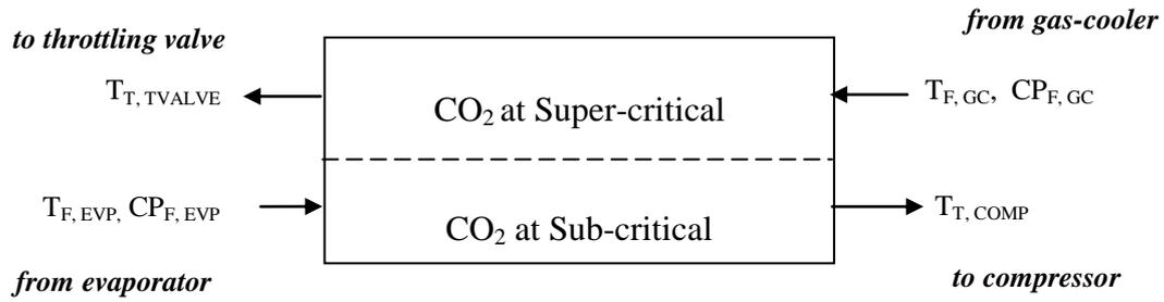
**Figure 4.2.1.3.1 Principle of internal heat exchanger sub-section**
