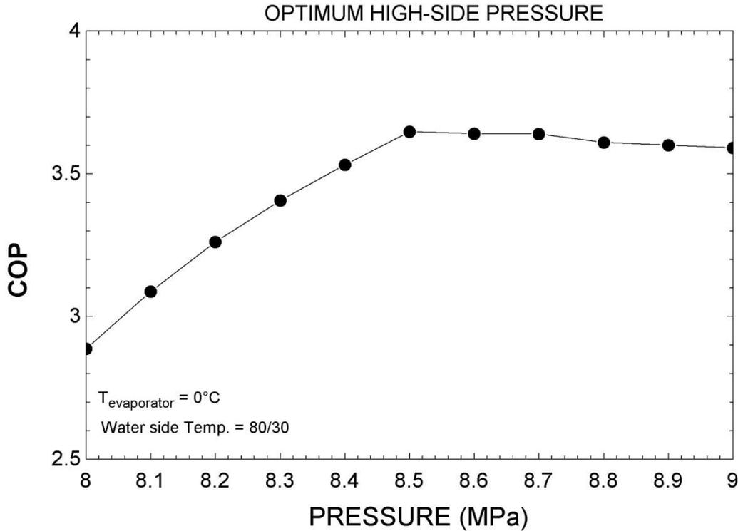
*Figure 4.2.3.1.1 Graph for COP vs. PRESSURE to find Optimum high-side pressure of the transcritical CO<sub>2</sub> heat pump cycle, developed using EES*
