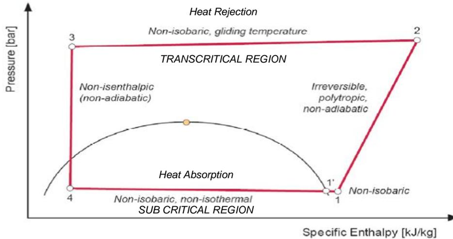
**Figure 1.4.2 Transcritical CO<sub>2</sub> heat pump cycle (Lorentzen cycle) P-h diagram**
