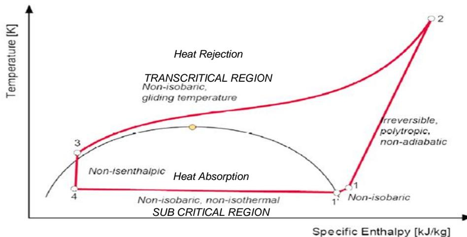
**Figure 1.4.1 Transcritical CO<sub>2</sub> heat pump cycle (Lorentzen cycle) T-h diagram (Source: J.Stene, *Intergrated CO<sub>2</sub> heat pump for space and hot water in passive houses*)**
