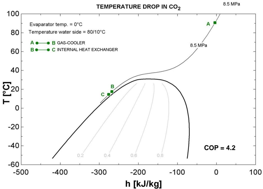
*Figure 4.2.3.2 Temperature glide in gas-cooler, for water side temperature of 80/10°C at a high-side pressure of 8.5 MPa. Developed using EES*
