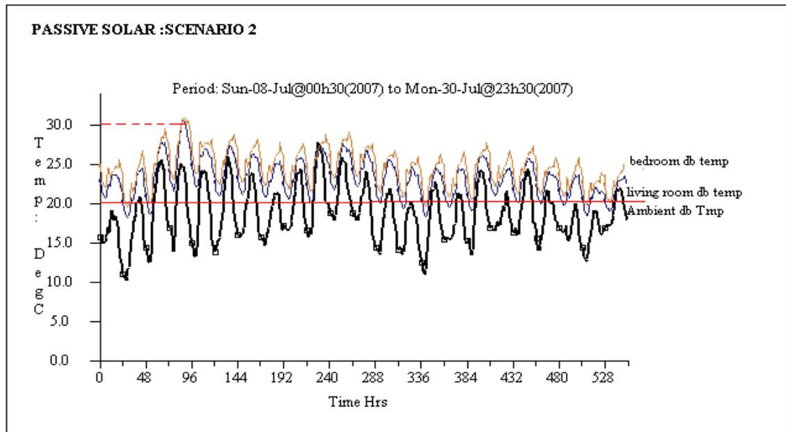
**Fig.4.8: Simulation for Scenario 2 of Passive Solar.**
