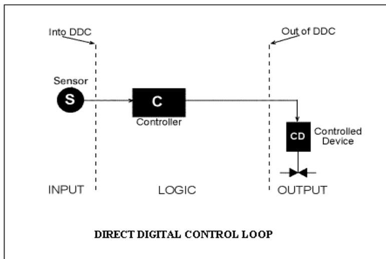
**Fig. 5.1: Diagram showing basic DDC loop**<sup>[32]</sup>
