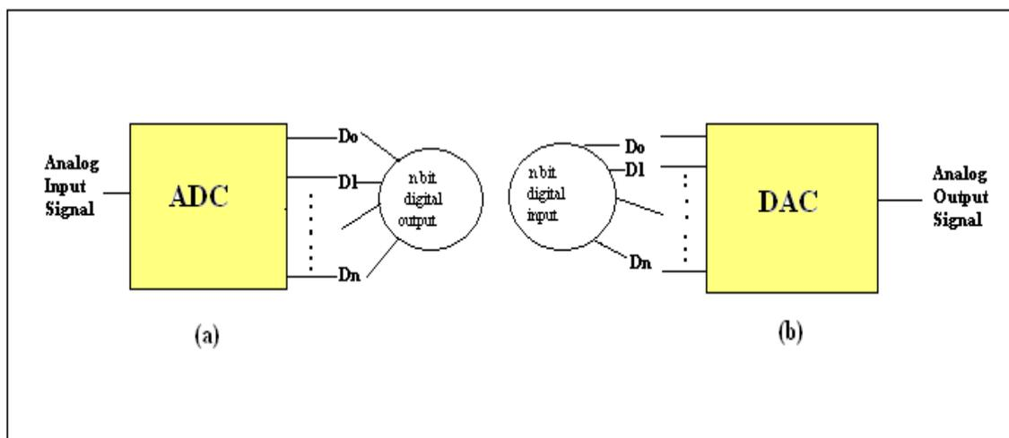
**Fig.5.6: Block Diagram of (a) ADC convertor (b) DAC convertor**<sup>[11]</sup>
