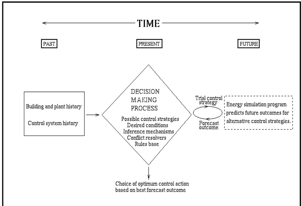
**Fig: 2.1: Energy Simulated-Assisted Control** <sup>[13]</sup>
