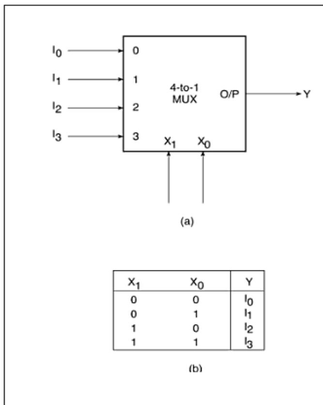
**Fig.5.4: (a) 4 to 1 multiplexer circuit representation, (b) 4 to 1 multiplexer Truth-Table**<sup>[1]</sup>
