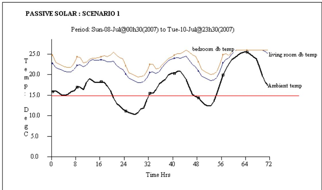
**Fig.4.7: Simulation for Scenario 1 of Passive Solar**
