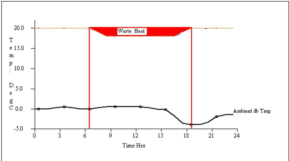
**Fig: 4.5. The waste heat production for the period from 07:00-17:00 (with control)**
