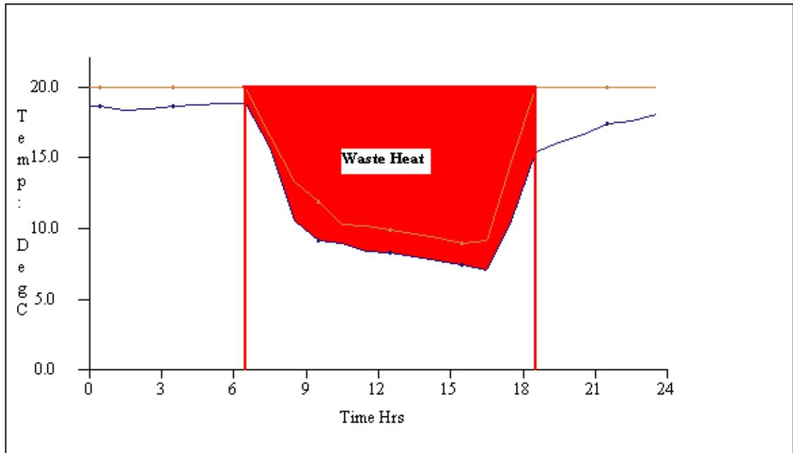
**Fig. 4.4: The waste heat production for the period from 07:00-17:00 (without control).**
