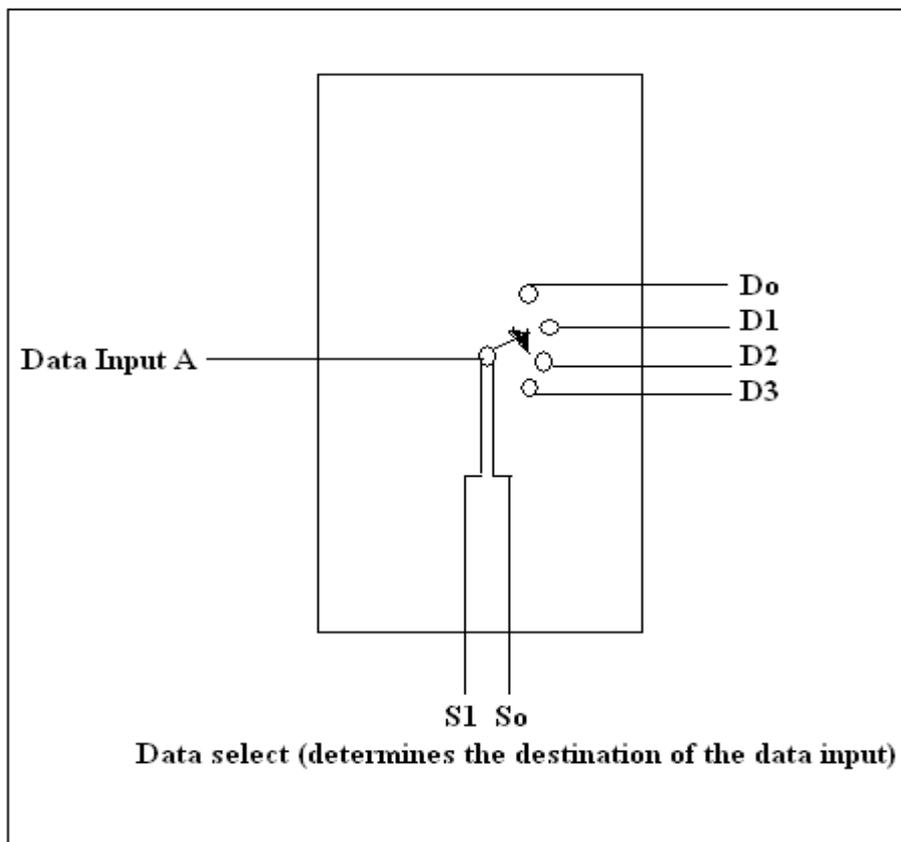
**Fig.5.5: Functional Diagram of 4 line De-Multiplexer** [9]
