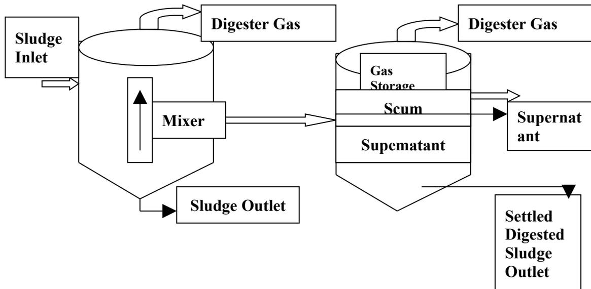
Figure 6: Two stage Digester [1]
