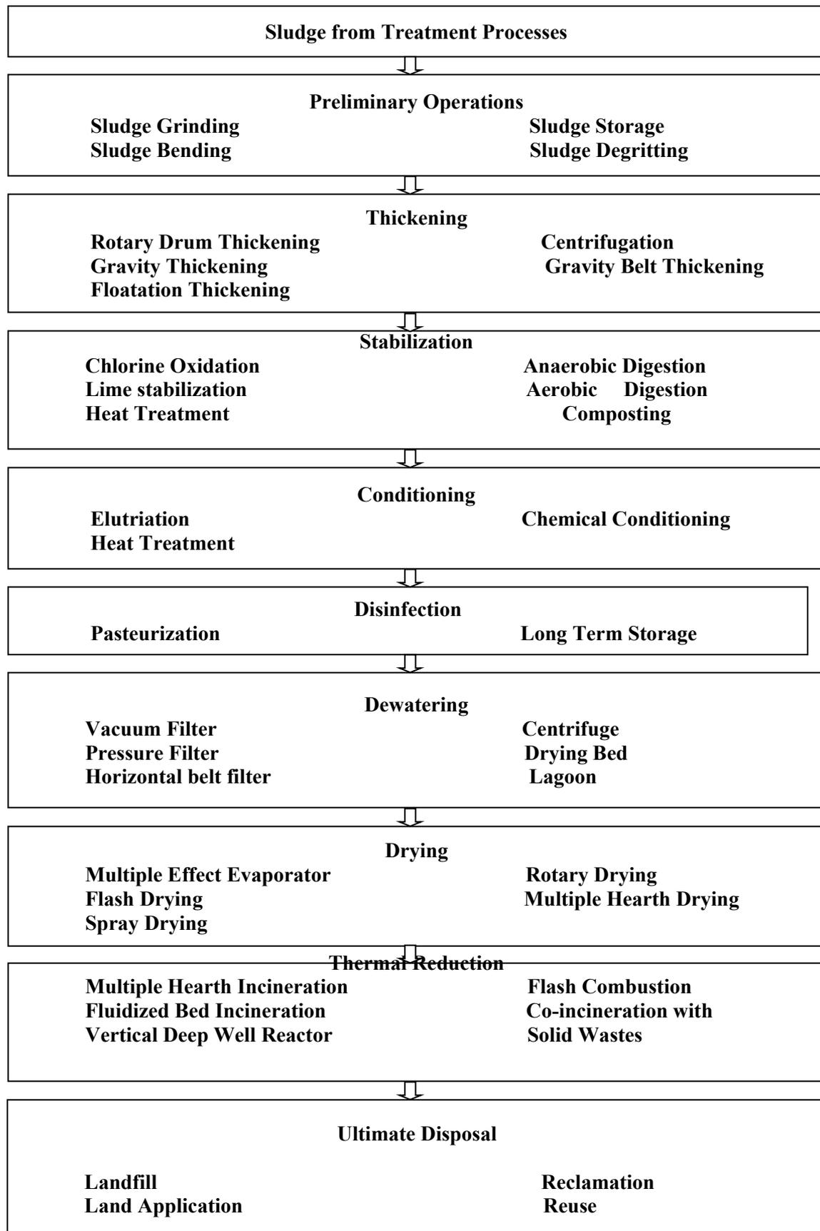
Table 1: Different Process of Sludge Treatment.
