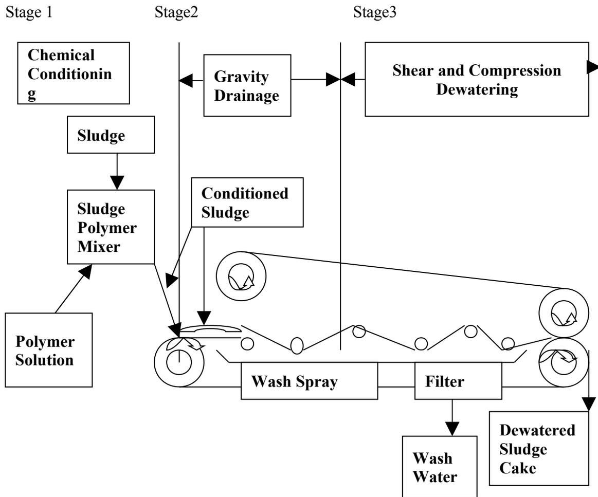
Figure 2: Belt Filter Press [1]
