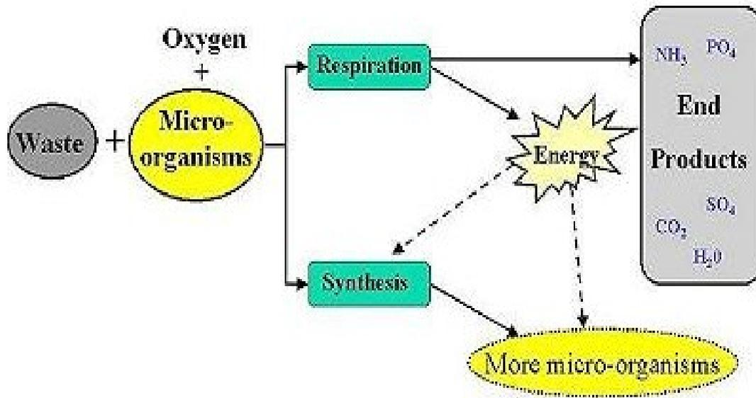
Figure 5: PATH of aerobic digestion [20]
