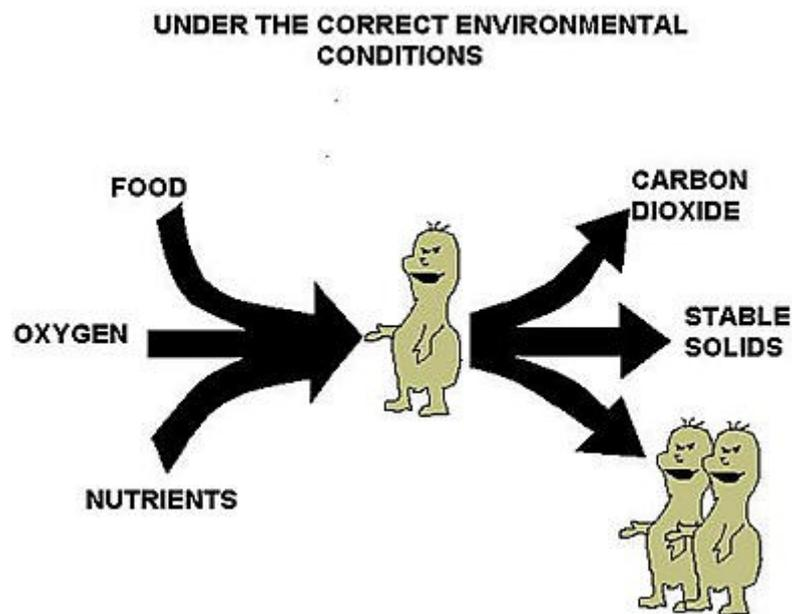
Figure 4: Process of Aerobic Digestion [20]
