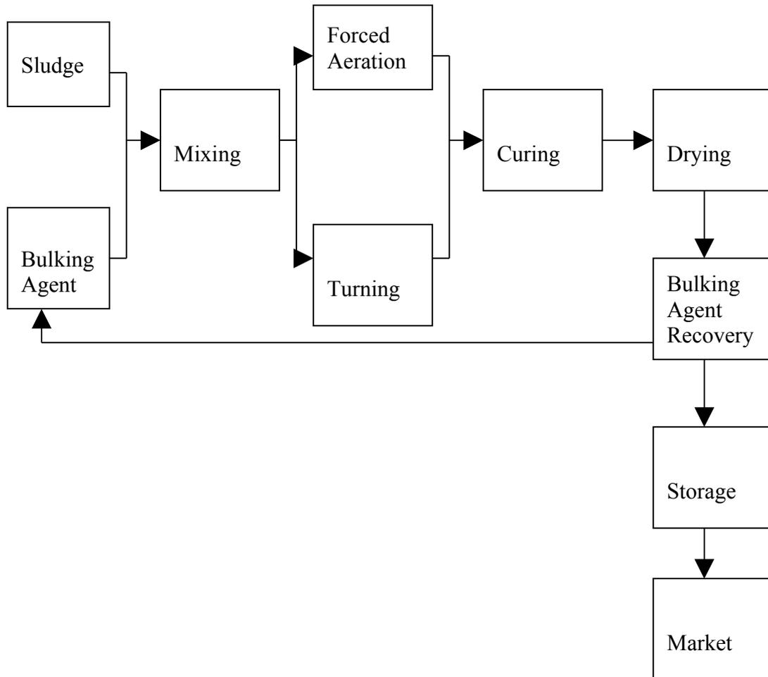
**Figure 1: Composting Process Flow Diagram [1]**
