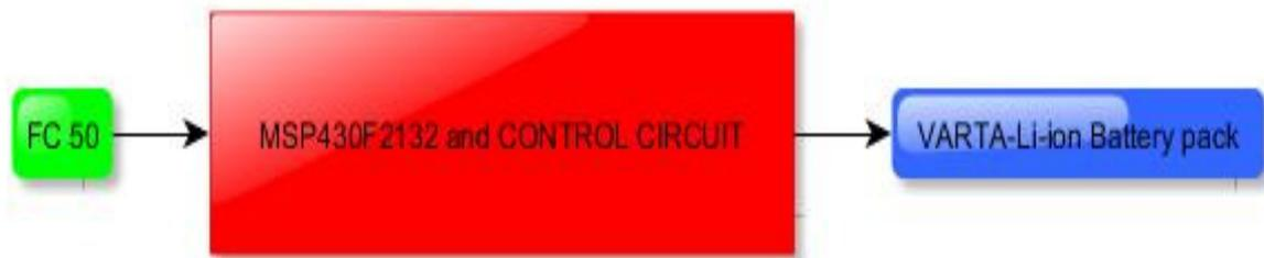
Figure 20a Battery Charger Block diagram
