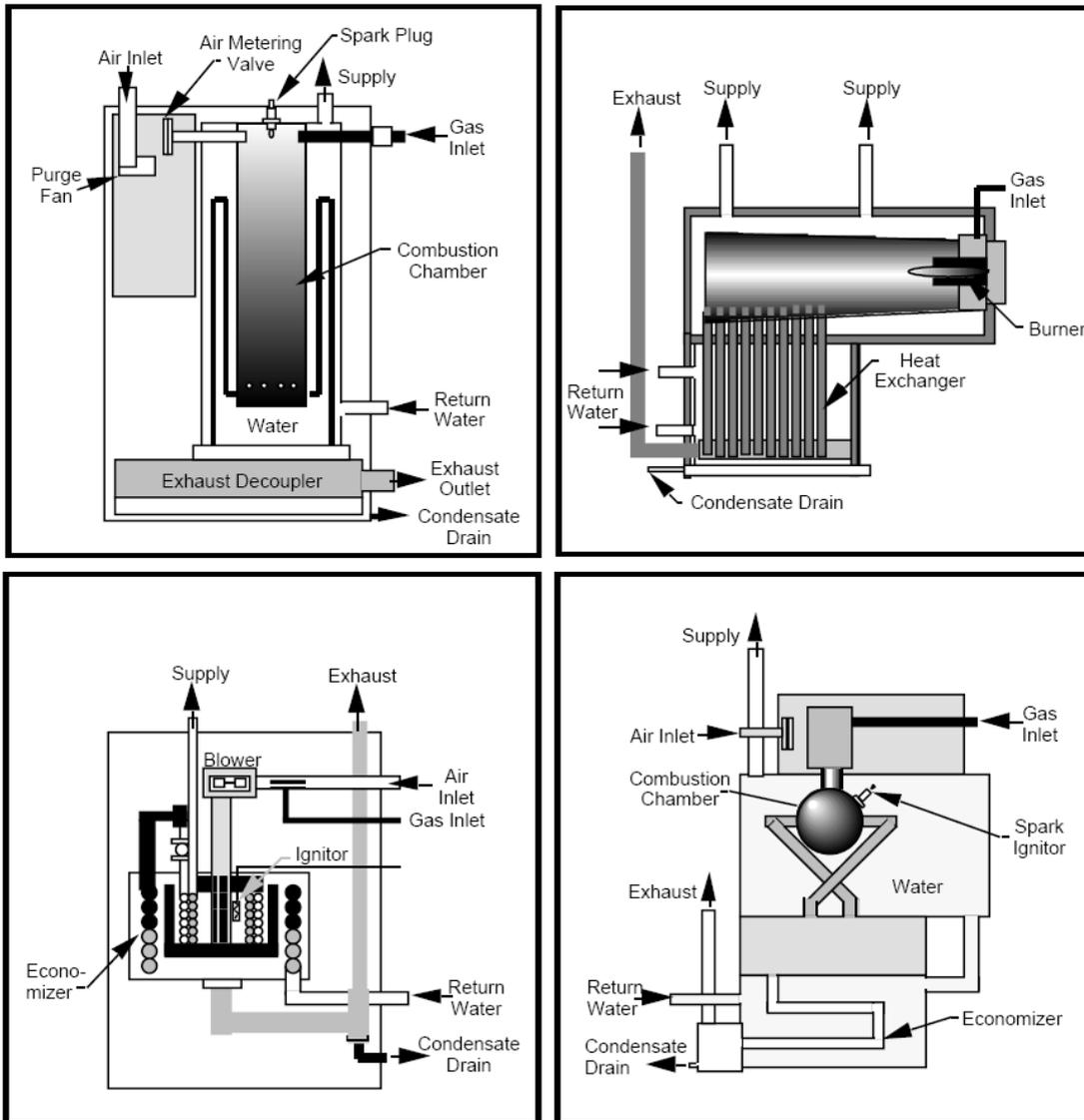
**Figure 4: Types of condensing boilers [15]**
