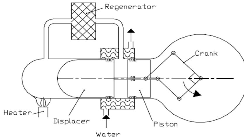
**Figure 2: Example of a Stirling engine (kinematic) [7]**
