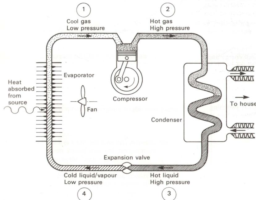
**Figure 1: Schematic of heat pump refrigerant circuit [4]**
