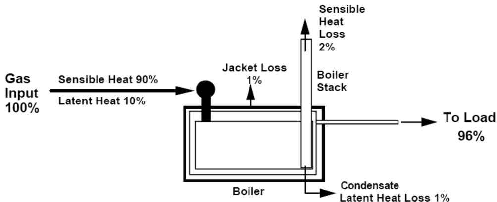
**Figure 3: Efficiency of condensing boiler** <sup>[15]</sup>
