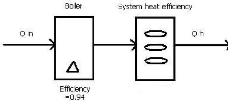
**Figure 9: Calculating the equivalent energy content of a condensing gas boiler**
